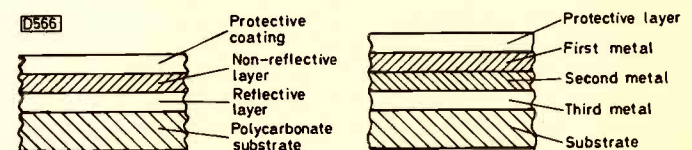
Fig. 5 (left): Structure of Yamaha's CD-R disc.
