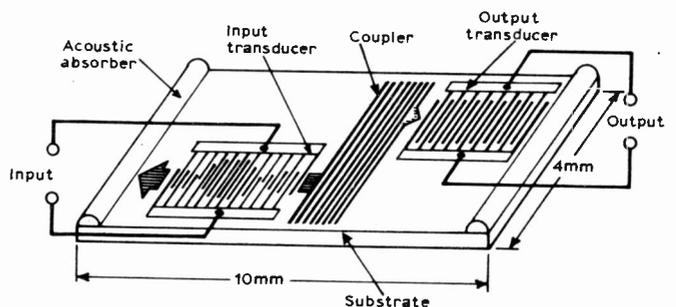
Fig. 2: (a) SAW filter structure.
