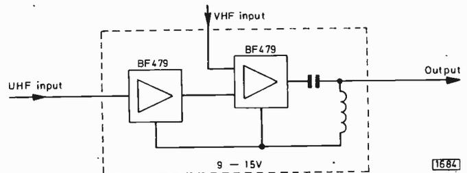
Fig 1: Block diagram of the Jostykit HF385 v.h.f./u.h.f. masthead preamplifier.
