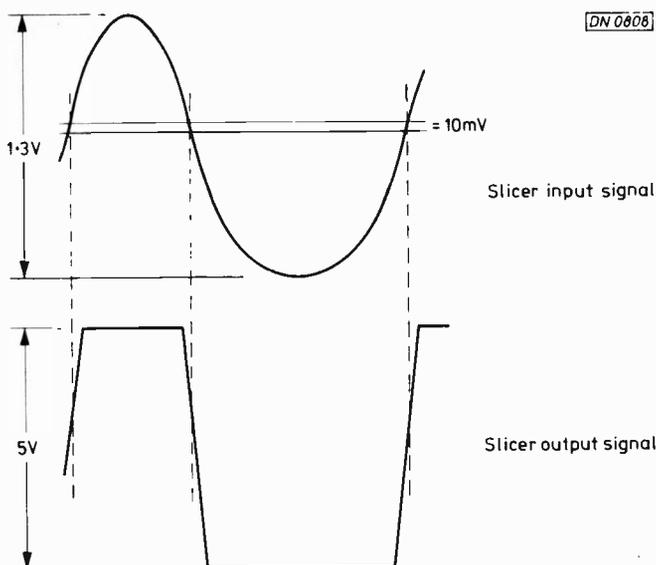
Fig. 3: Operation of the data slicer.
