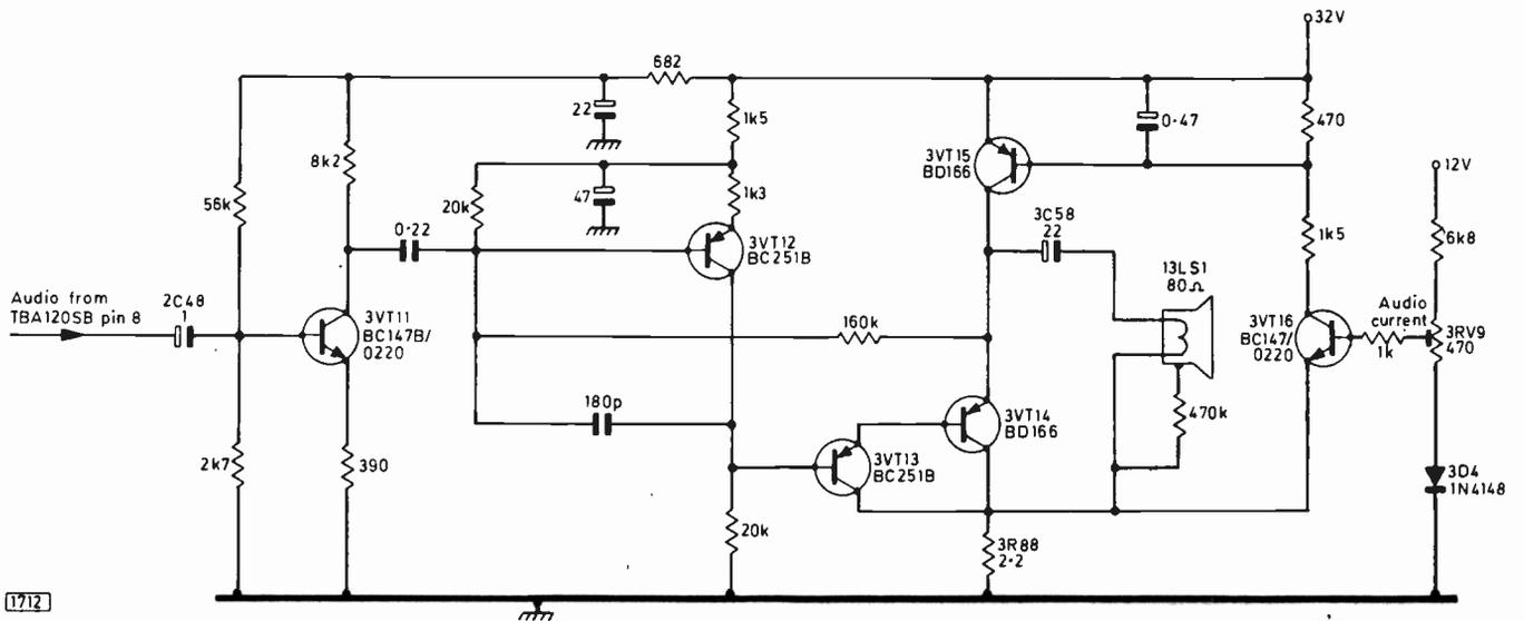
Fig. 2: The unusual looking audio circuit. 3VT15 provides a constant-current supply for the class A audio output transistor 3VT14. The base bias applied to 3VT15 is controlled by 3VT16, which senses the voltage across 3R88.
