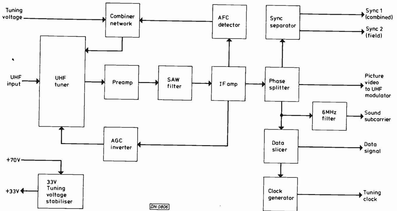
Fig. 1: Block diagram of the receiver/data recovery circuits.
