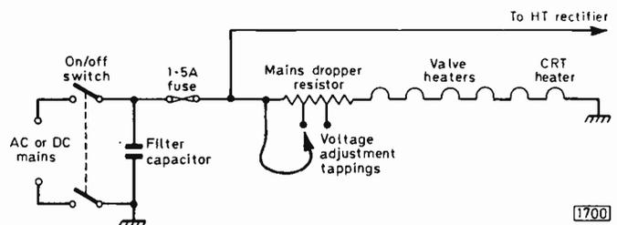
Fig. 8: A simple mains input and valve heater supply circuit for a valve TV set. Variations will be found in practice. The fuse for example may be connected at the input to the on/off switch rather than at its output and, as shown in Fig. 9, the filter capacitor may well come after the fuse.
