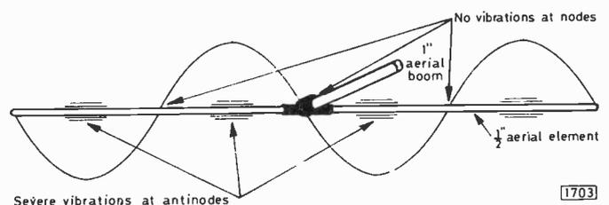
Fig. 1: Standing-wave vibration pattern noticed on a 120in. Band I aerial reflector element.
