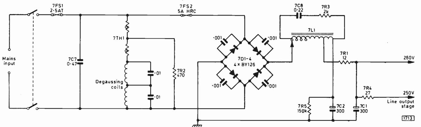
Fig. 3: The unregulated h.t. circuit provides a 250V supply (265V in larger screen models) for the line output stage and a 260V supply (275V in larger screen models) for the RGB output stages and to start up the line oscillator and driver stages. These voltages apply at zero beam current.
