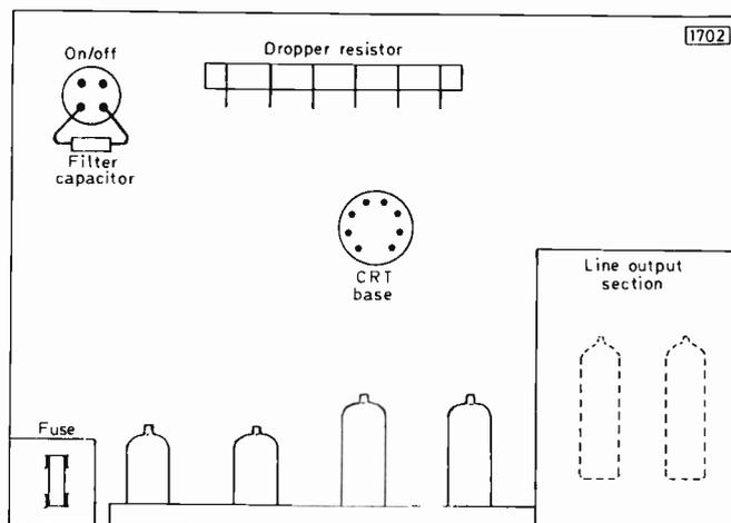
Fig. 10: The arrangement you may well see on taking the back off a typical valve monochrome set. The mains dropper resistor is generally mounted towards the top centre: less often it's mounted vertically at one side or the other, being cooled by acting as a "chimney". Some sections of the dropper are concerned with the h.t. supply.
