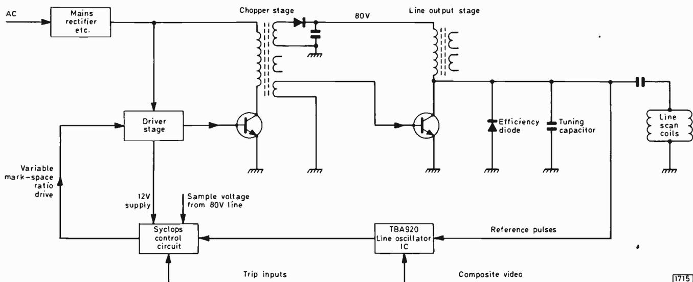
Fig. 1: Basic elements of the Syclops Mk. II regulated power supply/line output stage arrangement.
