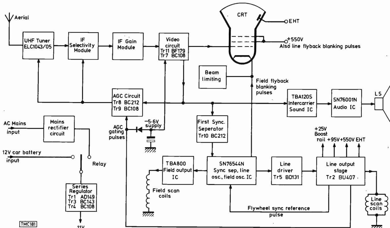
Fig. 1: Block diagram of the Television monochrome portable.
