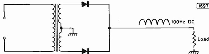
Fig. 5: This full-wave circuit provides a 100Hz output, the two rectifier diodes conducting on the alternate positive- and negative-going excursions of the a.c. input. This enables a smaller value reservoir capacitor to be used than in the half-wave rectifier circuit previously shown.
