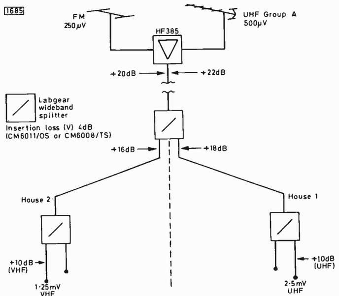
Fig. 2: Supplying two separate houses or flats with v.h.f. and u.h.f. signals, using the HF385 aerial preamplifier to combine the signals from a v.h.f. (f.m. radio) and a u.h.f. TV aerial. To reduce the cost of the installation, diplexers could be used instead of splitters. To simplify the calculations cable losses have been ignored: they must be taken into account of course in a practical installation.
