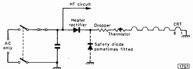
Fig. 9: An alternative mains input/heater supply circuit, using a diode to reduce the voltage applied to the heaters. In hybrid receivers, i.e. those using a mixture of valves and transistors, the i.t. supply for the transistors may be obtained from a filter capacitor connected to the chassis end of the heater chain – in this case tube pin 1 or 8 will not be connected to chassis.
