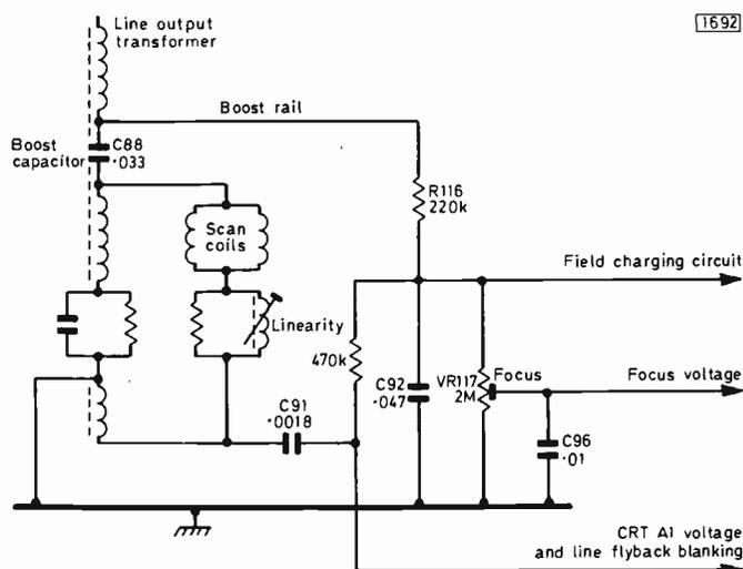
Fig. 1: Boost supply circuitry, Decca Models MS1700/MS2001/MS2401. A defective R116/VR117 network had resulted in a blown h.t. fuse. Note that C91 performs two functions: in addition to smoothing the c.r.t.'s first anode supply, it also couples the line flyback blanking pulses to this electrode.
