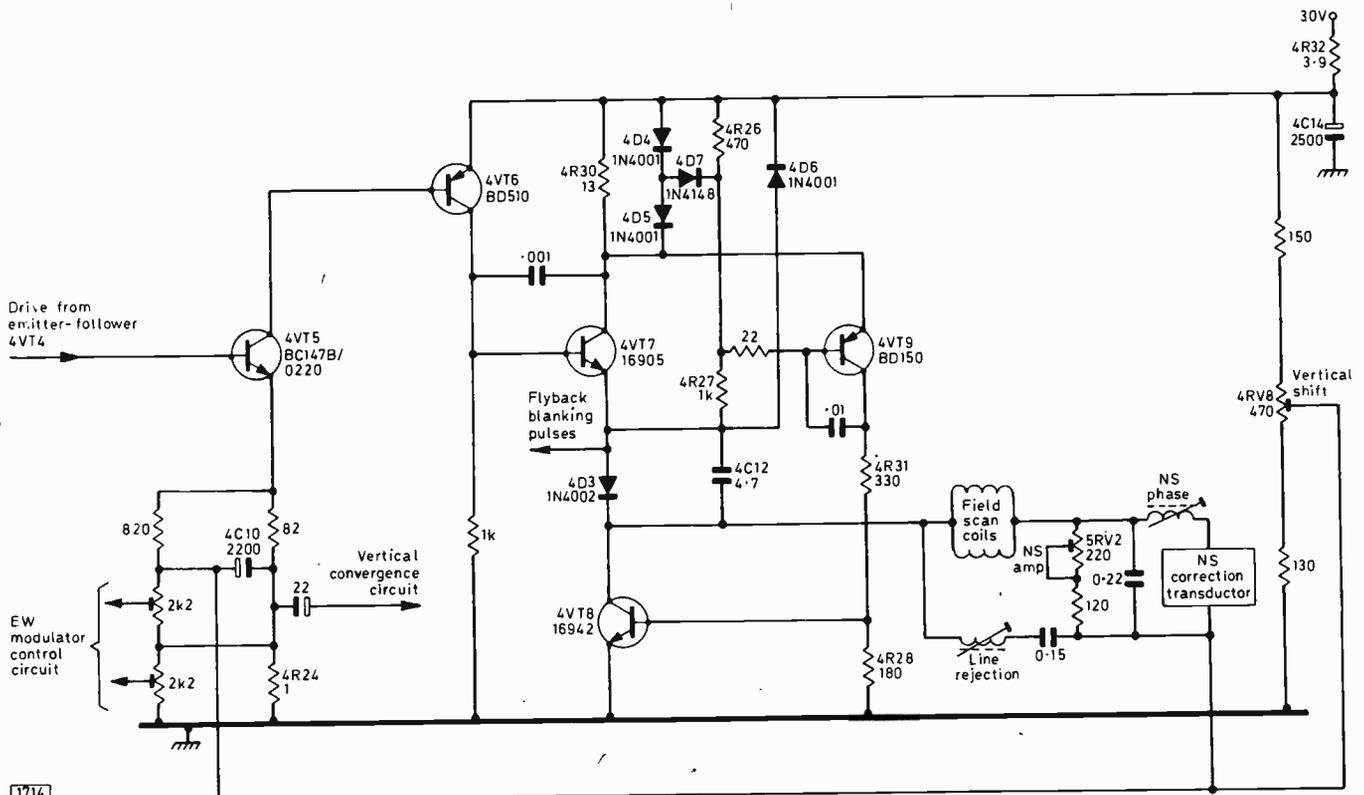
Fig. 4: Another unusual feature is the field output stage. The driver 4VT6 drives 4VT7 throughout the forward scan. Towards screen centre, 4VT9 begins to conduct, driving 4VT8 so that both 4VT7 and 4VT8 conduct during the second half of the scan. The a.c. path through the scan coils is completed by 4C10 and 4R24. 4C10 charges during the first half of the scan, and is discharged via 4VT8 during the second half of the scan.
