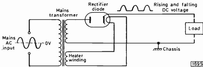
Fig. 3: Use of a diode valve as a rectifier. The output to the load from the arrangement shown would consist of a series of positive-going pulses, with gaps between them where the negative-going excursions of the a.c. input have been suppressed. The transformer can be used to reduce the mains voltage from a high to low value.
