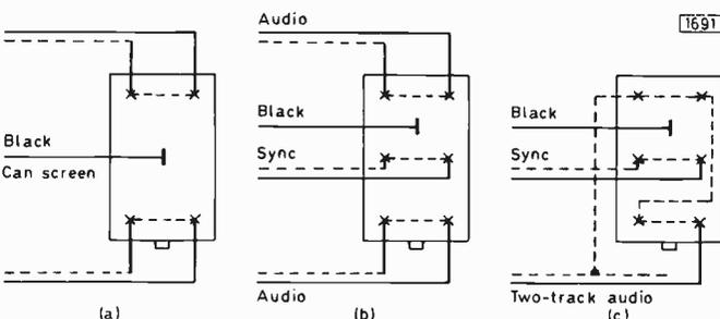
Fig. 1: Philips VCR audio/sync head connections. (a) Model N1500. (b) Model N1520. (c) Modified head arrangement to give two-track audio recording and playback on Models N1500/N1501. Viewed from the back (tag) side. There is single screw fixing at the base. The part number of the N1520 audio/sync head is 4822-249-10082.
