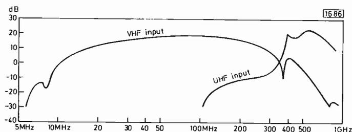
Fig. 3: The frequency responses (u.h.f. and v.h.f.) quoted for the Jostykit HF385 preamplifier. Practical tests confirmed the accuracy of these figures.
