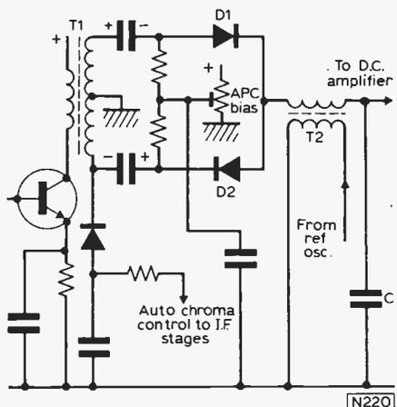
Fig. 12: A burst detector circuit. This phase sensitive detector produces a control voltage to lock the receiver's reference oscillator to that at the transmitter.
