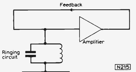
Fig. 7: General circuit of an oscillator as a ringing circuit plus an amplifier with positive feedback. The ringing element can be a series LC circuit, a quartz crystal or an RC circuit.
