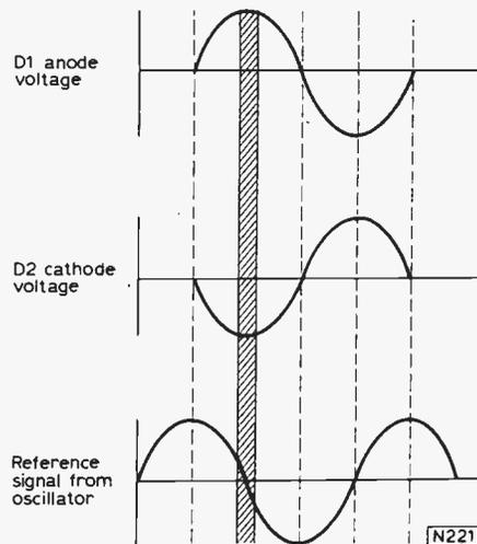
Fig. 13: Waveforms of the circuit of Fig. 12. The reference oscillator runs 90° out of phase with the incoming bursts.
