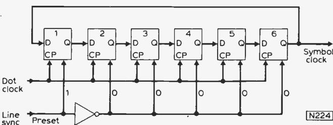
Fig. 45(b): A symbol clock divider using a shift register.
