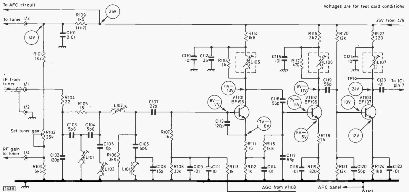
Fig. 2: Circuit of the i.f. amplifier.
