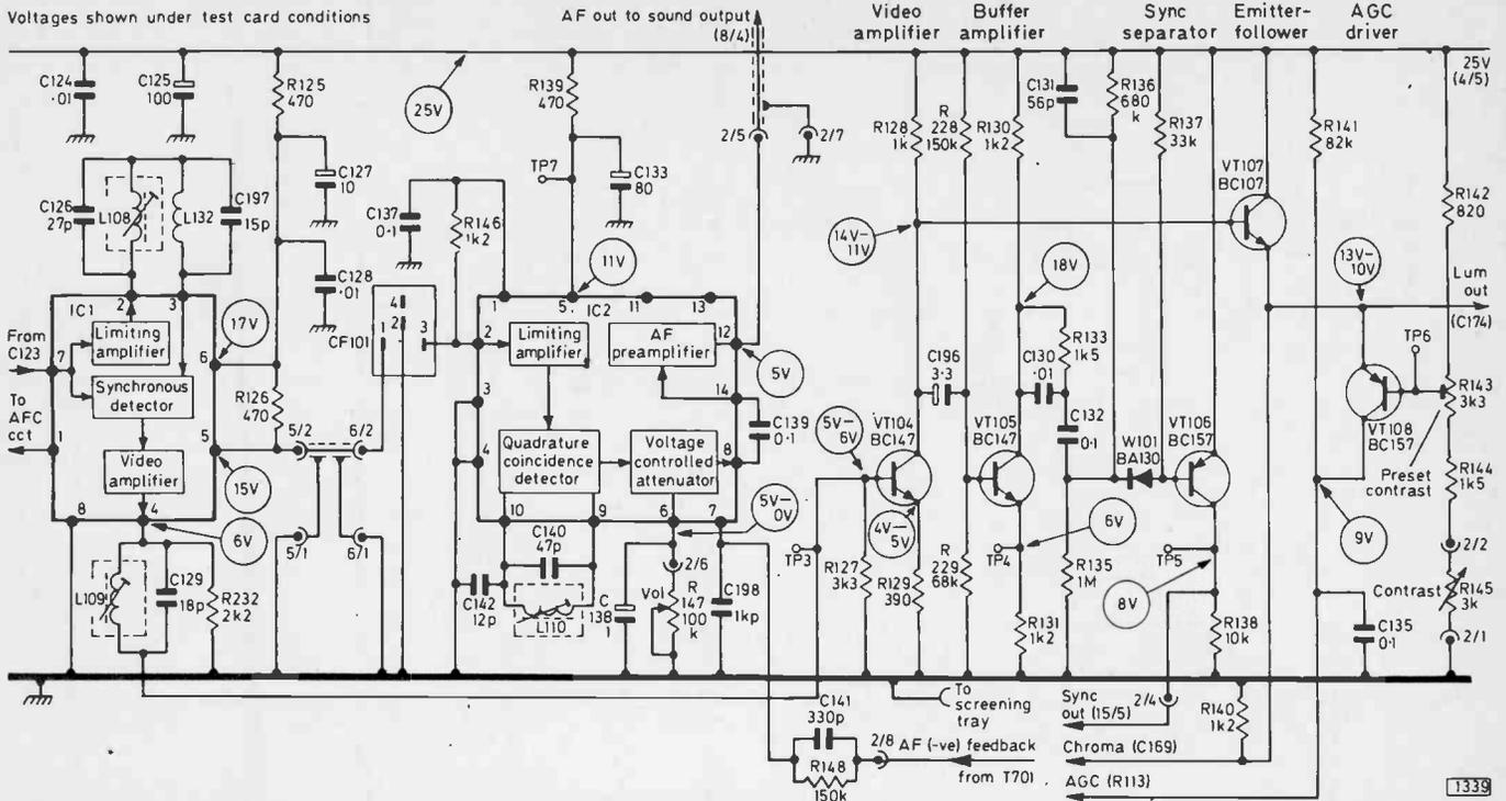
Fig. 3: The video detector (IC1), intercarrier sound (IC2), sync separator and a.g.c. circuits. Negative feedback from the secondary of the sound output transformer T701 is fed to pin 7 of IC2 via R148/C141: the tap on T701 was omitted in Fig. 3 last month.
