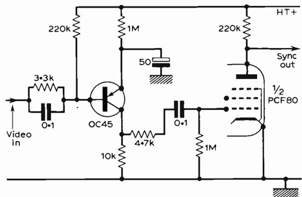
Fig. 5: The only transistor in an otherwise conventional chassis used in the Pye Model V710A was this OC45 sync separator stage. It was followed by a pentode sync pulse amplifier stage.
