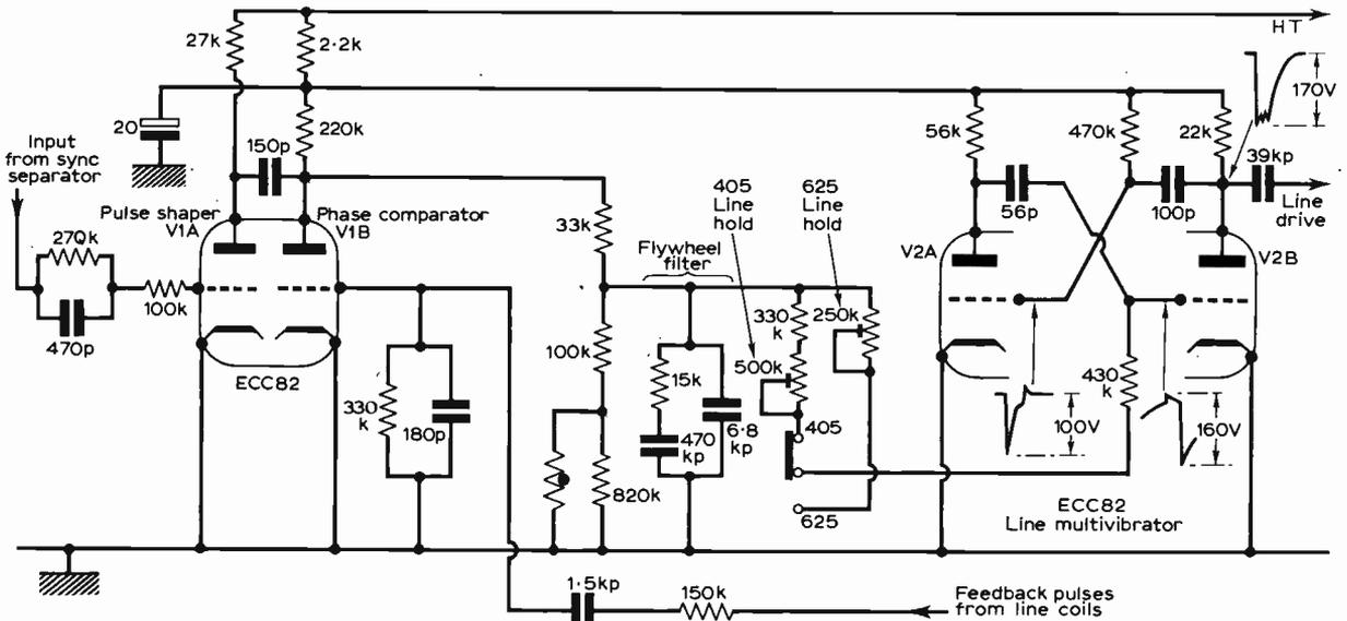
Fig. 3: Complete line generator circuit as found in current Philips models, using an anode-to-grid cross-coupled multivibrator, V2. This is controlled by a flywheel circuit using a simple triode phase comparator.
