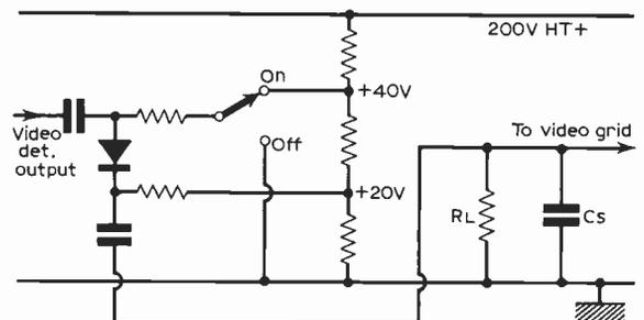
Fig. 3: Practical biased diode switch connected in series with the video signal path.
