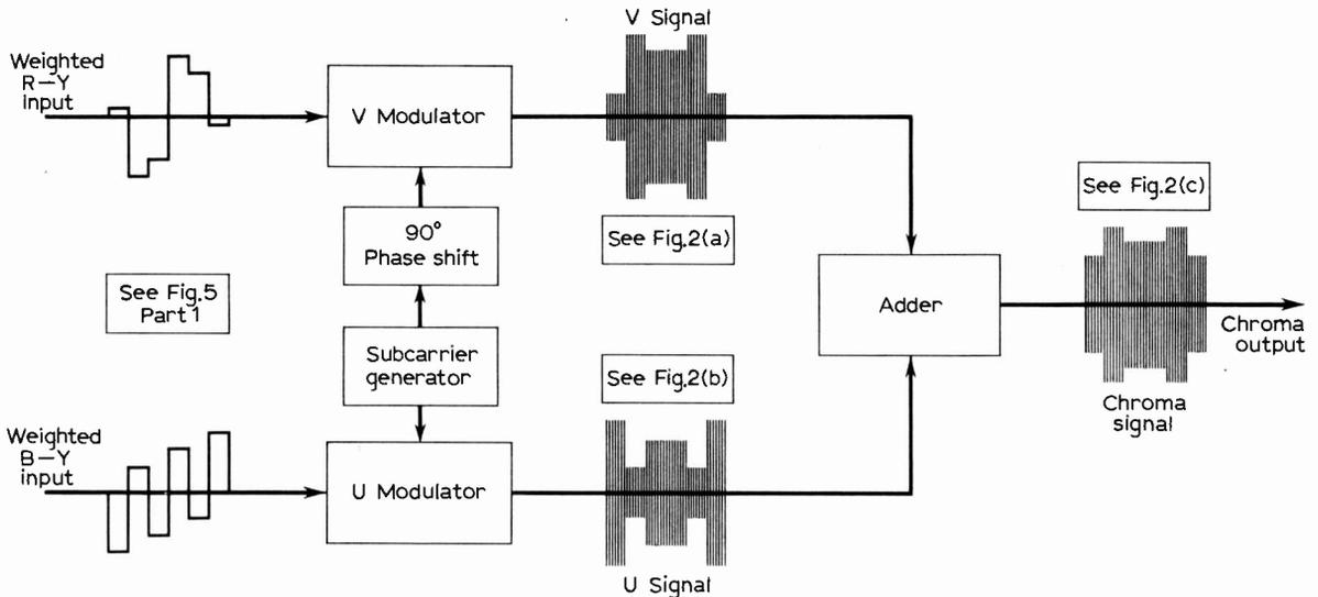
Fig. 3: Detailed block diagram of the chroma modulator section of a colour transmitter.
