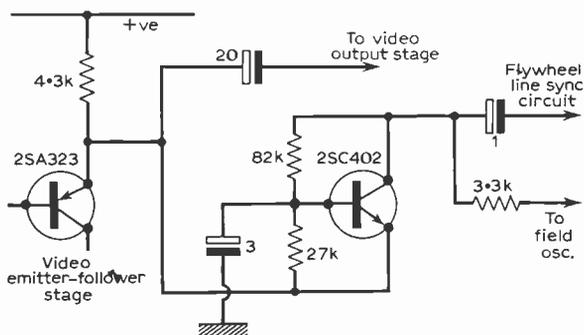
Fig. 7: Sony sync separator circuit.
