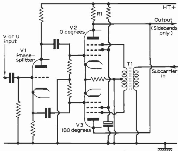
Fig. 1: Simple form of V or U modulator in which the subcarrier is suppressed, an output being obtained only when an input signal is applied via the phase splitter.
