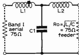
Fig. 2: Low-pass filter.
