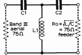
Fig. 3: High-pass filter
