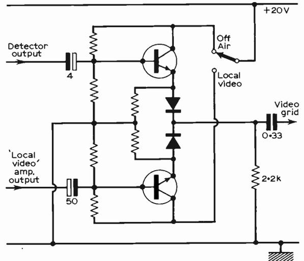
Fig. 4: Dual emitter-follower and switching diode arrangement used to link the video output stage to the detector or local video input.
