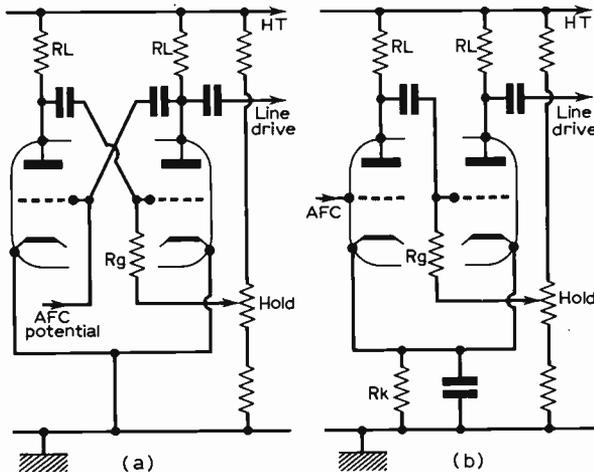
Fig. 4: The two basic forms of multivibrator, (a) anode-to-grid cross-coupled and (b) cathode-coupled with a single RC anode-grid coupling. It was general practice at one time for one valve to control the charge and discharge of a charging capacitor as in the blocking oscillator circuit.
