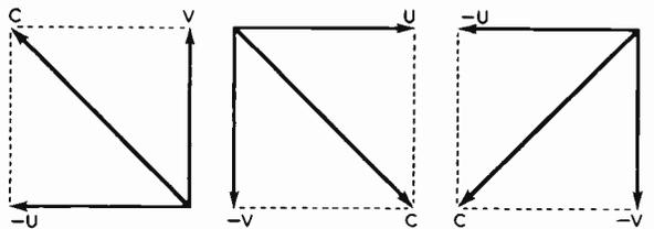
Fig. 8: The C signal can have any position within the full 360° since the V and U signals can have negative as well as positive values, as these diagrams show.
