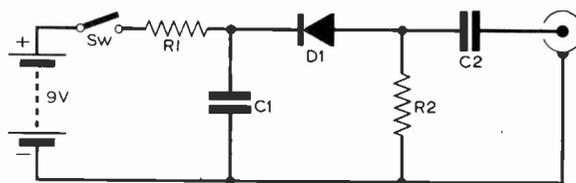
Fig. 3: Simple noise generator circuit.
