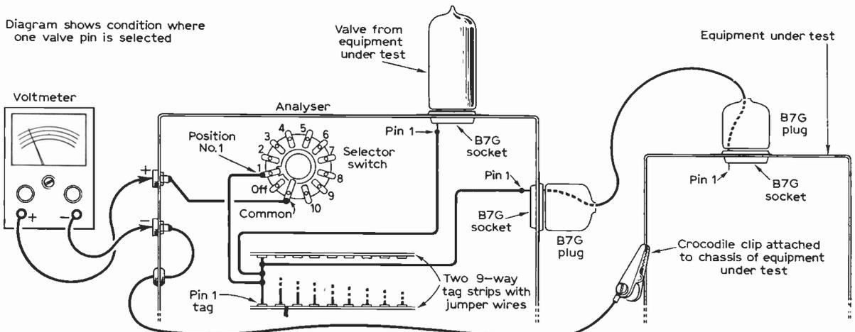
Fig. 1: Simplified circuit of the voltage analyser, showing the method of operation.
