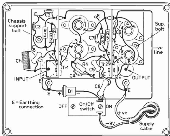
Fig. 2: Layout of the preamplifier.
