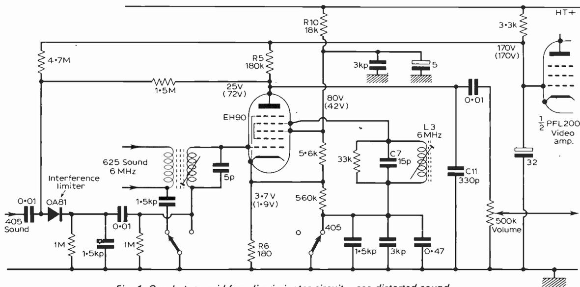
Fig. 1: Quadrature-grid f.m. discriminator circuit—see distorted sound.
