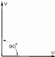
Fig. 6: Because of the 90° phase difference between the V and U signals they can be represented by this sort of vector diagram, where the lengths of the lines correspond to the amplitudes of the two signals.
