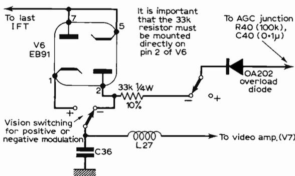
Fig. 4: Overload modification suitable for the Bush TV53-TV66 range of receivers.
