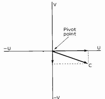
Fig. 9: The C signal can be considered as being pivoted at the centre of this diagram. The C signal swings about the pivot as the values of the U and V signals change.
