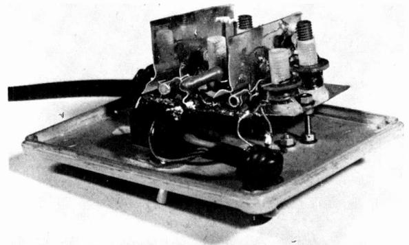
The interior of the prototype. Note the aluminium screening between the input and output circuits in each stage. The collector and shield connections are taken to one side of the screen, the base and emitter connections being taken to the other side.
