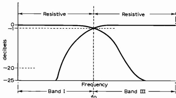
Fig. 4: Typical diplexer bandpass characteristics.
