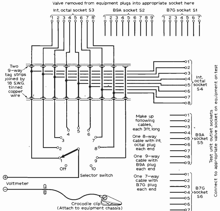
Fig. 2: Basic circuit of the voltage analyser, showing one valve socket and one output socket only connected. The switch numbers correspond to the valve plug and socket pin numbers. The two nine-way tagstrips are joined by 18 s.w.g. tinned copper wire jumpers and the 57 leads from the six sockets and the switch are soldered to these jumper leads.
