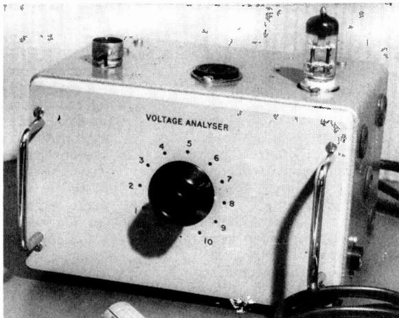
The author's prototype. This is housed in a metal cabinet but in the interest of safety a wooden case is recommended.
