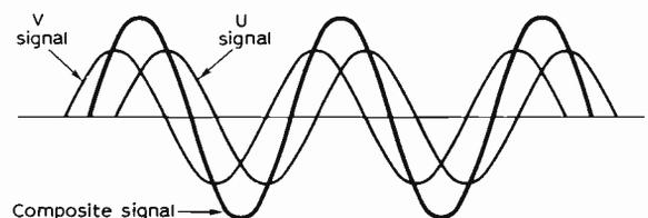
Fig. 5: The addition of the V and U signals, shown in thin line, results in the signal shown in heavy line.
