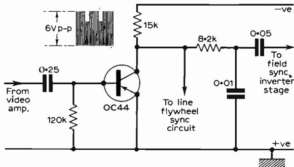
Fig. 3: An early transistor sync separator stage, used in the Pye all-transistor Model TT1 released in 1961. This is a deceptively simple circuit. The transistor acts as a clipper, removing the video content of the input waveform to allow through only the sync pulses.
