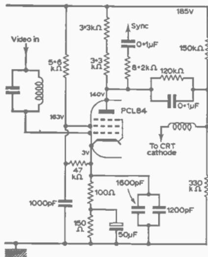
Fig. 22—Video amplifier from Ferguson 506T. Note the use of two series anode load resistors.
