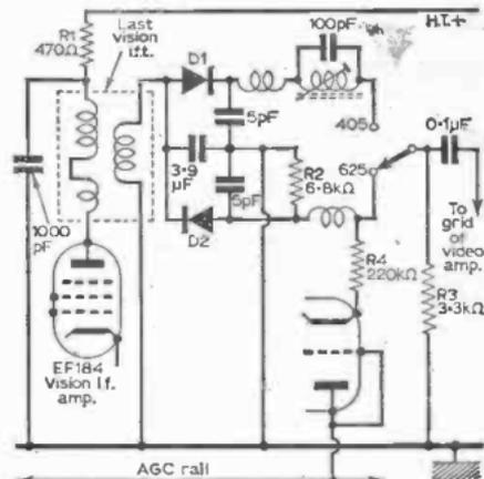
Fig. 2—Dual-standard vision detector employing 2 diodes. (Aib.) D1 and D2 (OA79's) are the 405 and 625 detectors respectively, with R4 3.3 kΩ resistor as common detector load but virtually shunted on 625 by R2 to increase bandwidth to accommodate 6Mc/s inter-carrier sound. Diode connected PCL84 triode functions as overload diode on 625. A.C. coupling to video amplifier valve eliminates need for bias change on system change-over.
