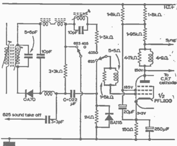
Fig. 25—Method of coupling dual-standard signals to the video amplifier (Philips detector and video circuit).
