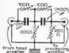
Fig. 32—Basic afterglow correction circuit.
