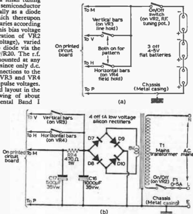
Fig. 2.—Power supplies for the test generator; (a) for battery operation and (b) for mains operation.
