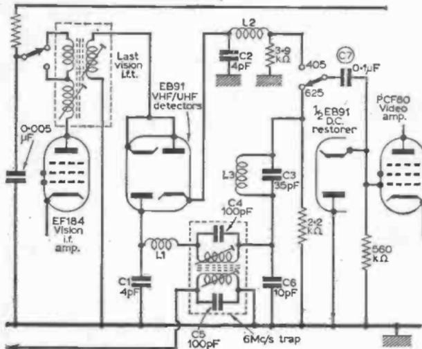
Fig. 3—Dual-standard vision detector circuit (Decca). L1/2/3 are i.f. filter chokes with R1 and R2 respectively being 405 and 625 detector diode loads. A.C. grid coupling V1<sub>8</sub>. C7 to video amplifier grid has d.c. restoration by EB91 diode. Unusually, the 6Mc/s inter-carrier sound i.f. is taken from the detector instead of from the video amplifier valve.
