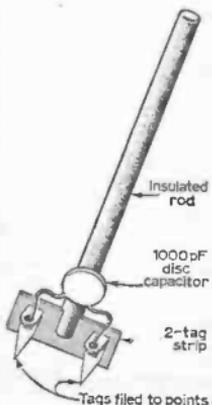
Fig. 5—Home-made in-circuit capacitor tester.
