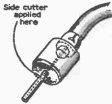
Fig. 1—Method for fitting plug without soldering.
