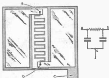
▲ Fig. 3—Thin film circuit.
