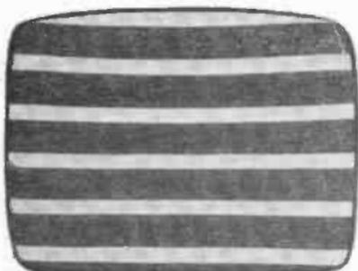
Fig. 6—Horizontal bar generator running at an exact multiple of the field frequency. (Useful for checking field linearity.)
