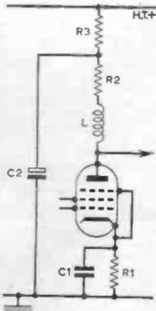
Fig. 20—Basic video circuit.
