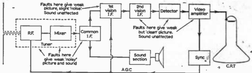
Fig. 2—Block schematic showing the sections of a 405-line receiver prone to sensitivity faults.
