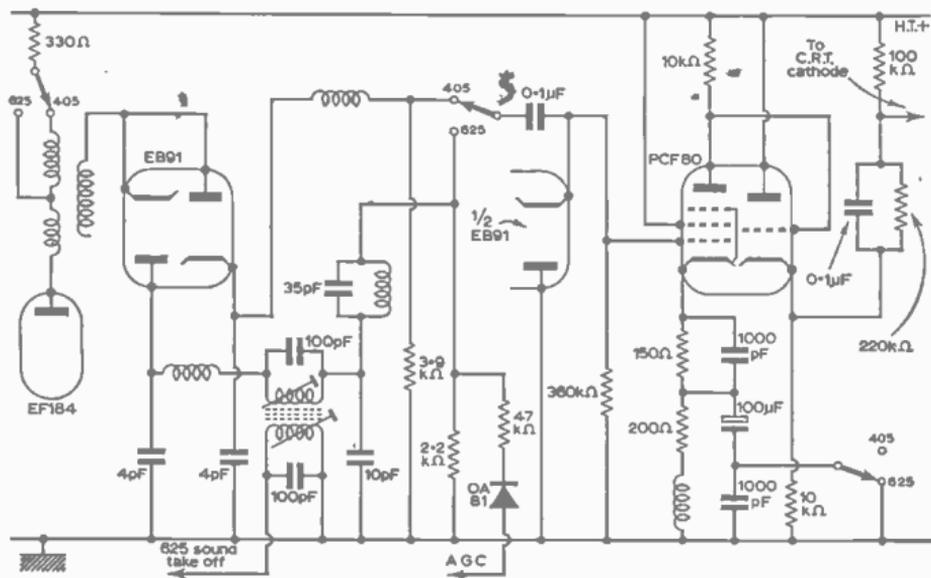
Fig. 21—An example of modern cathode follower video amplifier and output stages is given by the Decca circuit. This has many common features, but also one or two quite individual tricks of design and is worth studying.
