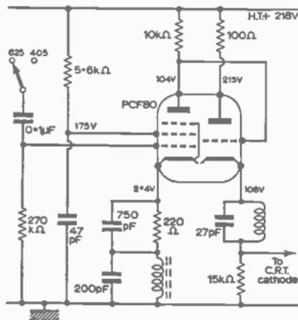
Fig. 24—Cathode-follower circuit used in many Bush models.
