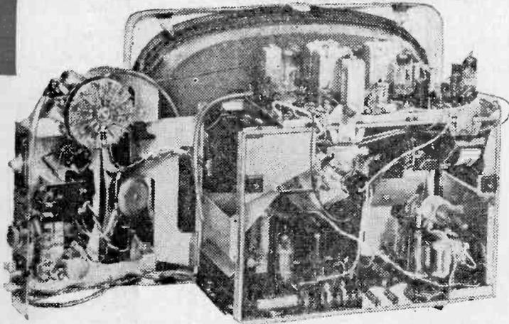
A Ferguson receiver which uses hinged printed circuit panels.
