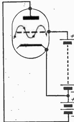
Fig. 1.—A simple circuit illustrating the production of B-K oscillation.
