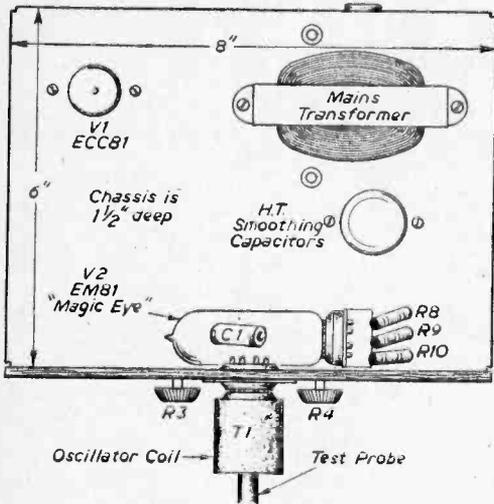
Fig. 3 (above)—An above-chassis view.
