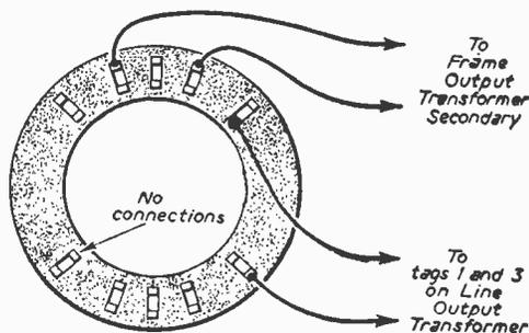
Fig. 20.—The scanning coil connections.
