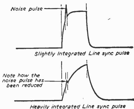
Probably the easiest way of doing this is to reduce the size of the capacitor which couples the sync pulse to the oscillator. The smallest usable hold range is determined by the amount of long term and short term frequency drift, which in turn is governed by the quality and character of the components, and by the temperature rise.
