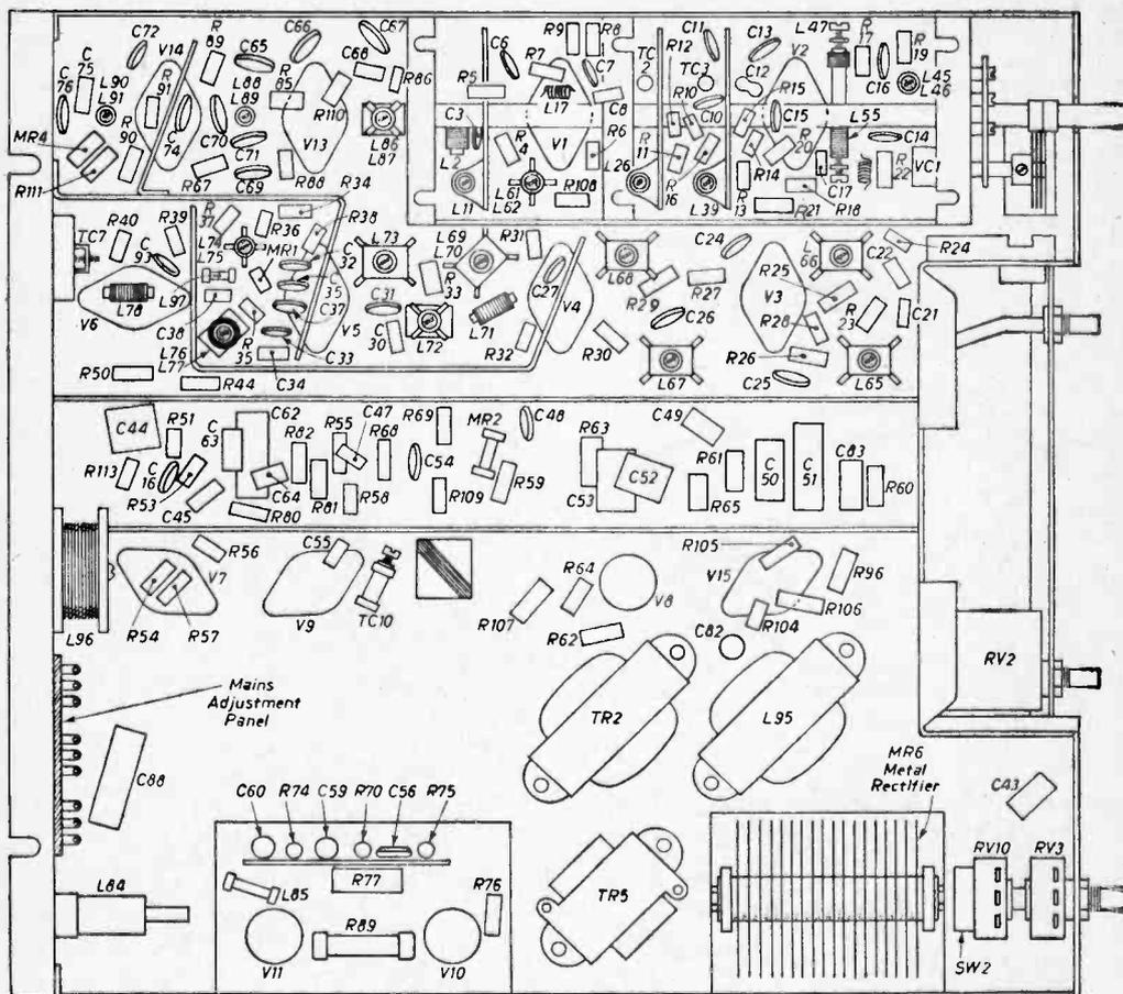
Fig. 8.—The underchassis component layout of the 1854.
