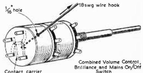
Fig. 3.—Loosening welded mains contacts.
