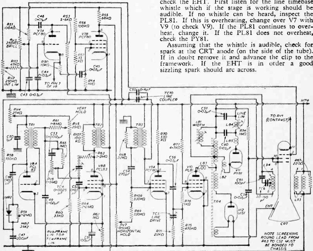
Fig. 6.—The timebase circuit.
