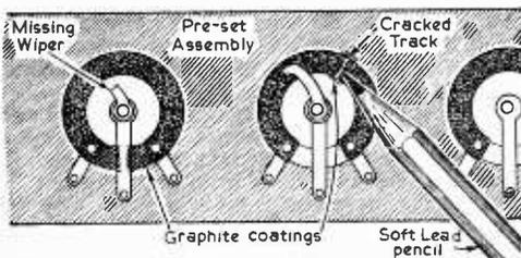
Fig. 2.—Repairing broken pre-sets.
