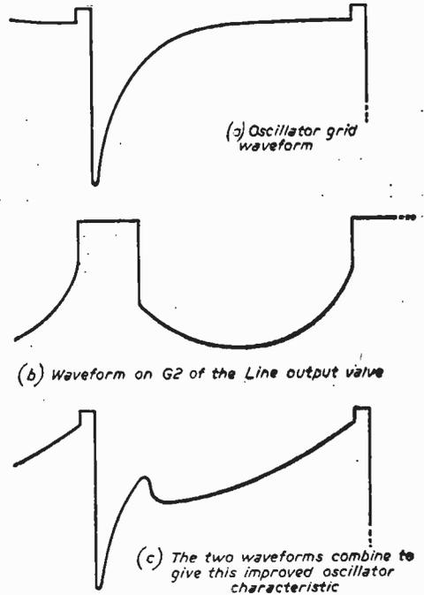
Fig. 21.—Steepening the grid waveform by feedback from G2 of the line output valve.
