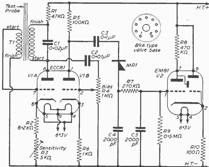
Fig. 2.—The circuit of the tester (without the power section, which is conventional).
