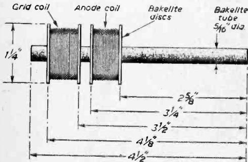
Fig. 5.—The construction of the test probe.
