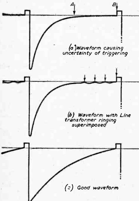
Fig. 20.—Grid waveforms and their effect on synchronization.
