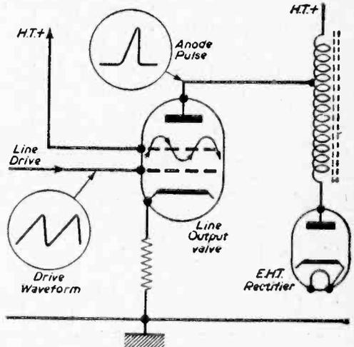
Fig. 2 (above).—The basic circuit of a line output stage and its waveforms. The sinuous arrow traces the path of the electrons.
