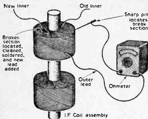
Fig. 4.—Locating and repairing broken windings.
