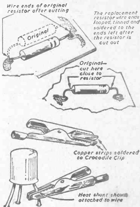
Fig. 2.—Making heat shunts for removing transistors.
