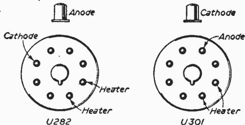
Fig. 6.—To use a U301 valve in place of a U282, the anode and cathode leads are transposed.
