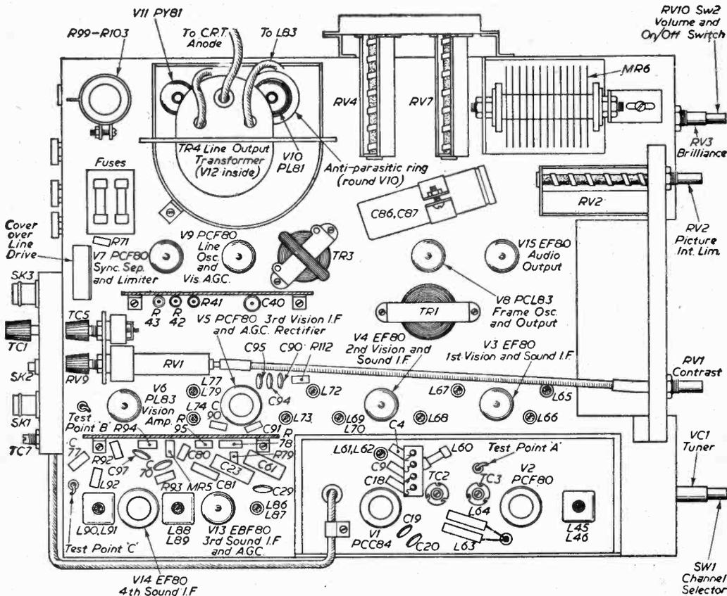
Fig. 4.—An above-chassis view of the HMV 1854.
