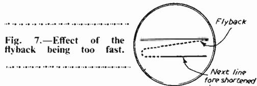
Fig. 7.—Effect of the flyback being too fast.
