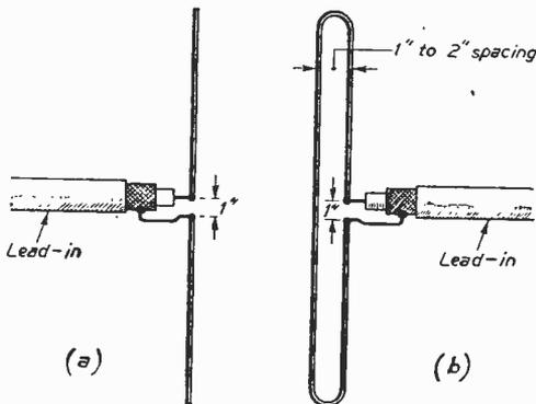
Fig. 1a (left).—The construction of a simple dipole.
