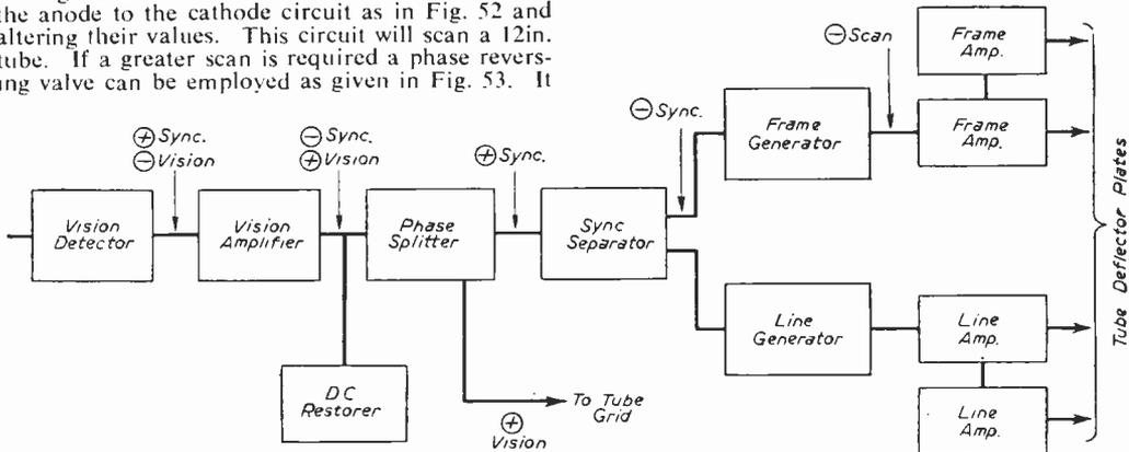
Fig. 51.—Block diagram of a receiver employing electrostatic deflection.
