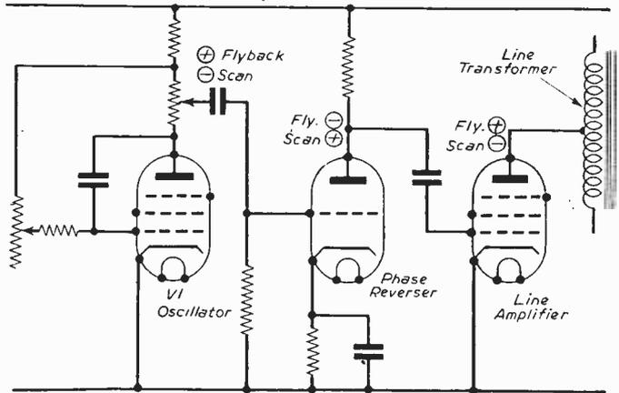
Fig. 53.—Incorporating a phase-reversing valve when changing from electrostatic deflection to magnetic deflection.
