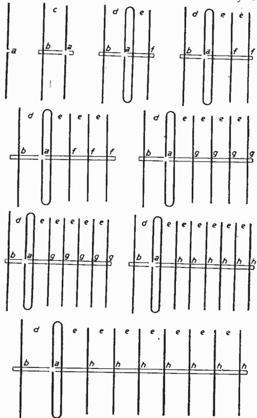
Fig. 5.—Various aerials ranging from a simple dipole to a 9-element Yagi. The letters "a" to "h" refer to the lengths of the elements or to their spacings, e.g., "a" is the length of the dipole, "b" the length of the reflector.
