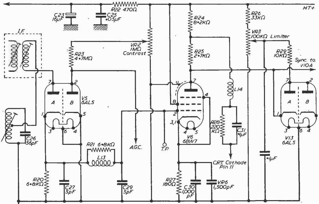
Fig. 1. 5. —Vision detector, AGC diode, video amplifier, vision limiter and H.T. feed (via R22) to early stages.
