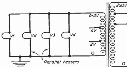
Fig. 55.—Parallel heater circuit.
