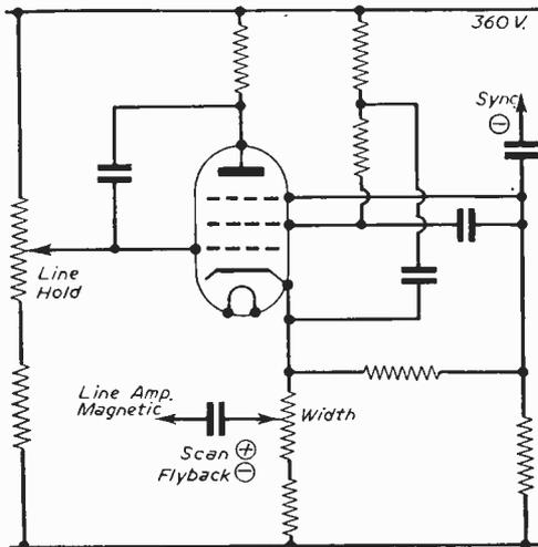
Fig. 52.—Miller transitron timebase.
