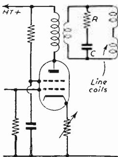
Fig. 5.—Line output stage with damping components.
