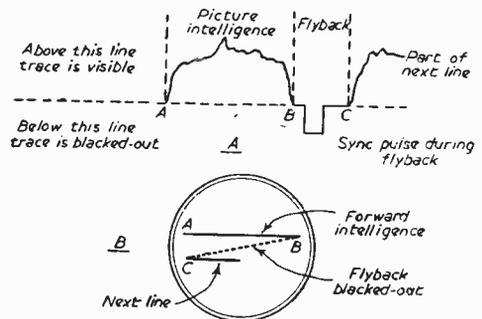
Fig. 3.—Waveform for one line.
