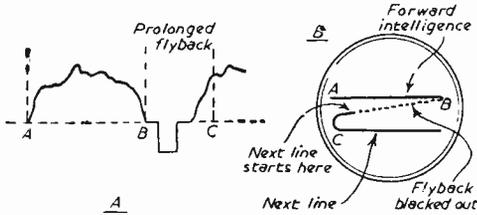
Fig. 4.—Waveform when flyback is late.
