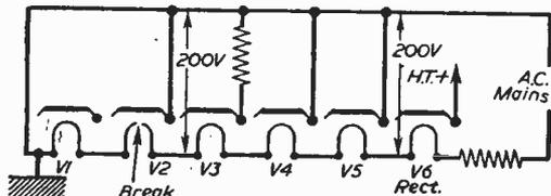
Fig. 59.—An open-circuit heater chain.
