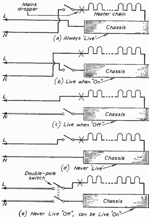
Fig. 1.—Results of various methods of connecting the mains.
