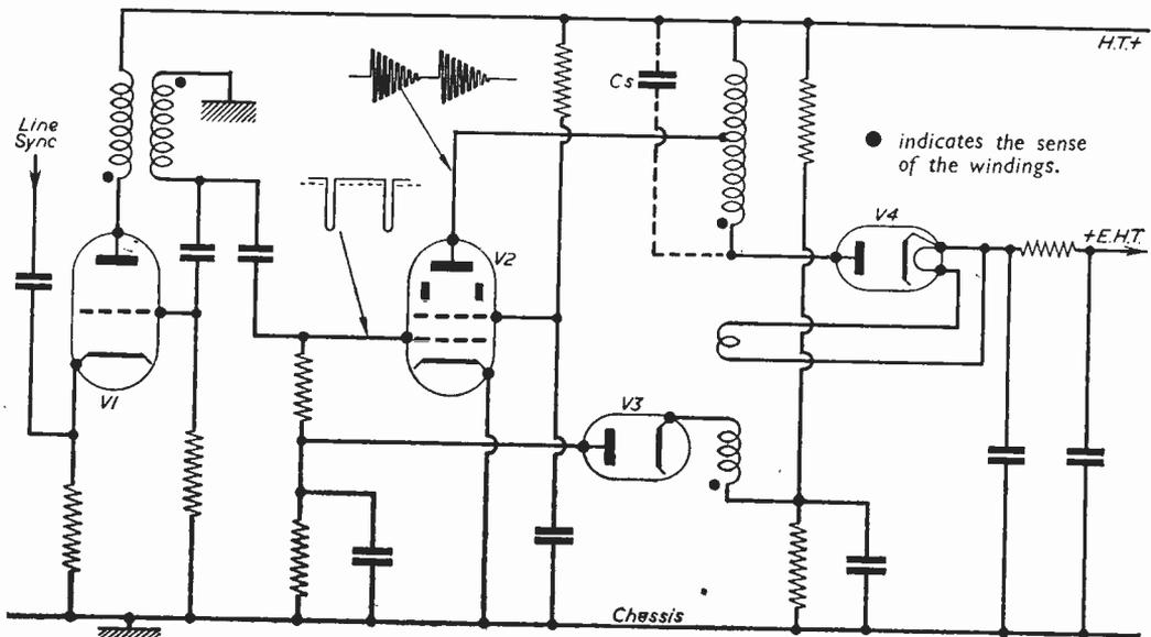
Fig. 9.—Pulse-type EHT supply. A series of negative pulses from the blocking oscillator, V1, releases burst of free oscillation in the anode circuit of V2. The regulation is improved by V3 which supplies a control bias to V2 from a separate winding.
