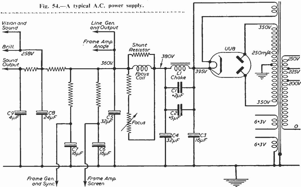
reservoir condenser and C4 and C5 are the smoothing capacitors. Notice the care taken to ensure adequate decoupling between stages to prevent any interaction or feedback along the H.T. line and to ensure a smoothed, ripple-free D.C. supply. The decoupling capacitors are C6, 7, 8, 9. The function of the focus coil has been discussed in a previous article. Transformer fed parallel heaters are shown in Fig. 55.
