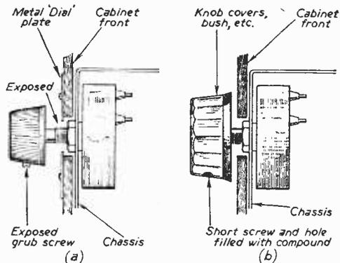
Fig. 2.—The danger of exposed metal parts.
