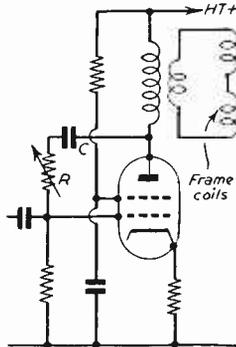
Fig. 6.—Frame output stage with feedback.
