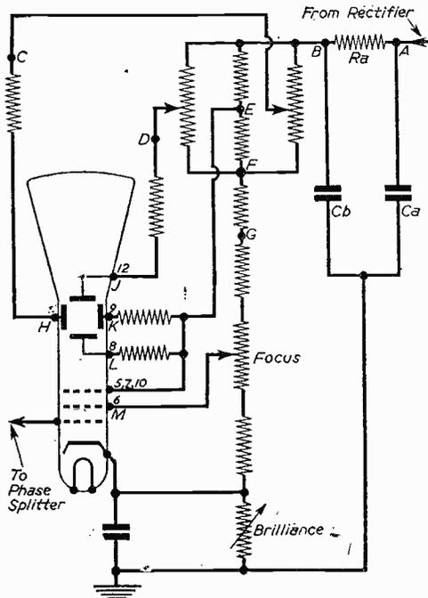
Fig. 2.—Testing points on electrostatic EHT.
