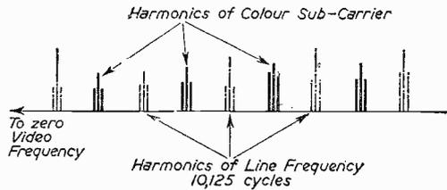
Fig. 1.—Frequency spectrum of the video signal.
