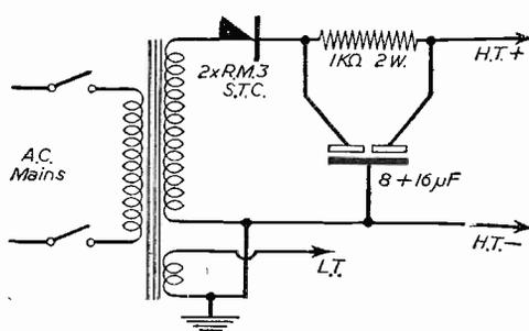
Fig. 4.—Suitable power supply unit.
