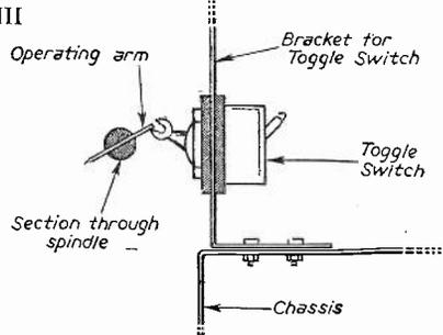
Fig. 5.—Method of mounting power supply switch.
