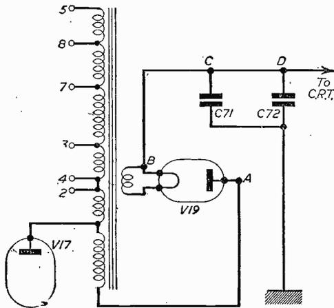
Fig. 3.—Testing points on electromagnetic EHT.
