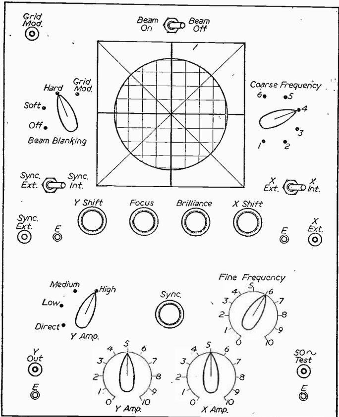
Diagram of the controls for the finished instrument.
