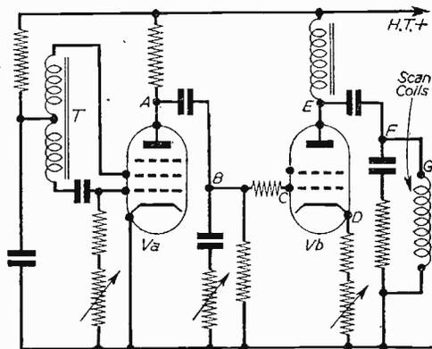
Fig. 7.—Blocking oscillator stage with amplifier.
