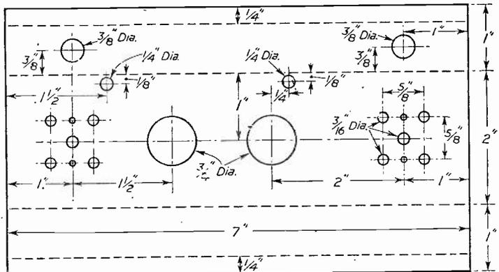
Fig. 7.—Details of the chassis.
