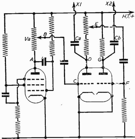
Fig. 5.—Typical line circuit for electrostatic tube.
