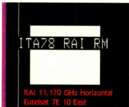
Photo 6: RAI's pulse-and-bar pattern used prior to a feed via Eutelsat W3 at 11-170GHz H.
