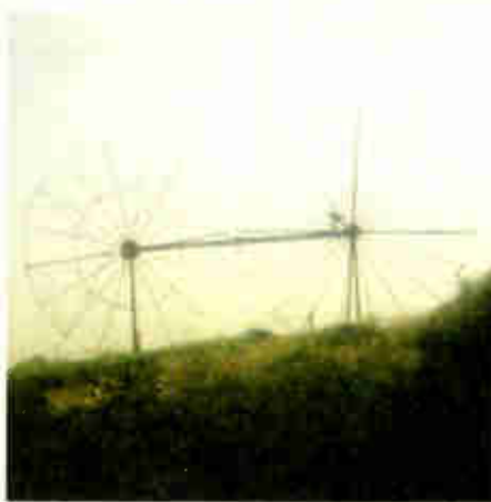
Photo 1: Large skeleton dishes used on the Laois/Kilkenny border in Southern Ireland to receive BBC and ITV transmissions from Wales.
