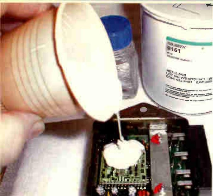
**Photo 2: A motorcycle ignition unit being encapsulated with non-corrosive silicone rubber.**
