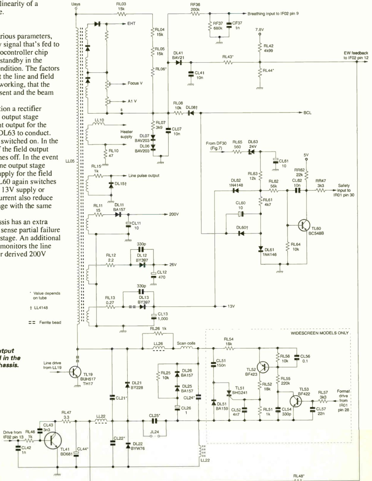
Fig. 5: The line output stage circuit used in the Thomson TX92 chassis.
