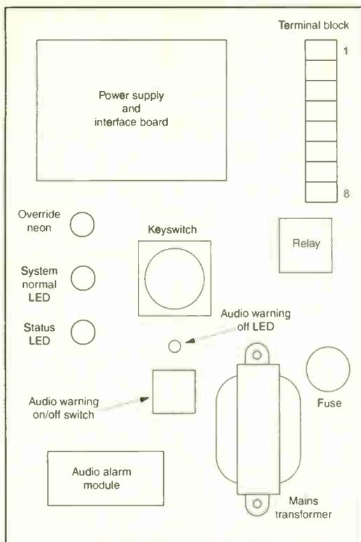
**Fig. 10: Suggested locations of the various items inside the control box. Component layout for the power supply and interface board and the audio alarm module is not critical in any respect. Drill fixing holes for the power supply and interface board to match mounting pillars in the box. Terminal block connections are as follows: 1 signal in; 2 +9V out; 3 0V; 4 mains live in; 5 mains neutral in; 6 earth; 7 and 8 relay contacts (mains or motor control).**
