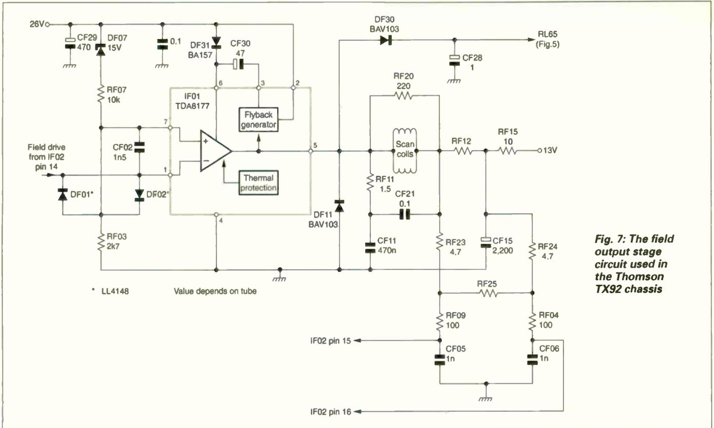
Fig. 7: The field output stage circuit used in the Thomson TX92 chassis
