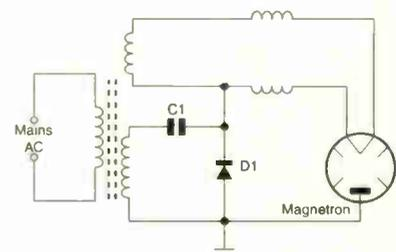
Fig. 1: The basic magnetron circuit.
