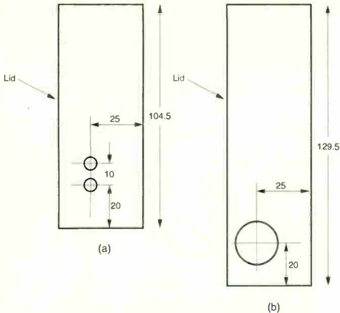
**Fig. 8: Positions of the IR LEDs in the side of the PX1 box (a). Position of the phototransistor tube in the side of the PX2 box, (b). Dimensions in mm.**
