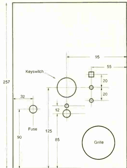
**Fig. 9: Positions of the items at the front of the control box (this is the bottom of the box, see text). Dimensions in mm.**
