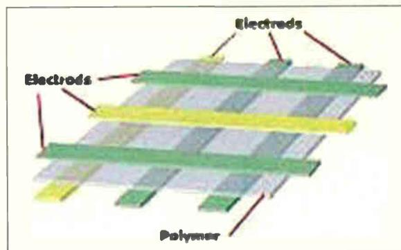
Photo 1: The ThinFilm Polymer plastic memory consists of a sheet of plastic sandwiched between a grid of electrodes. A cell able to store a one or zero exists at each electrode intersection.
