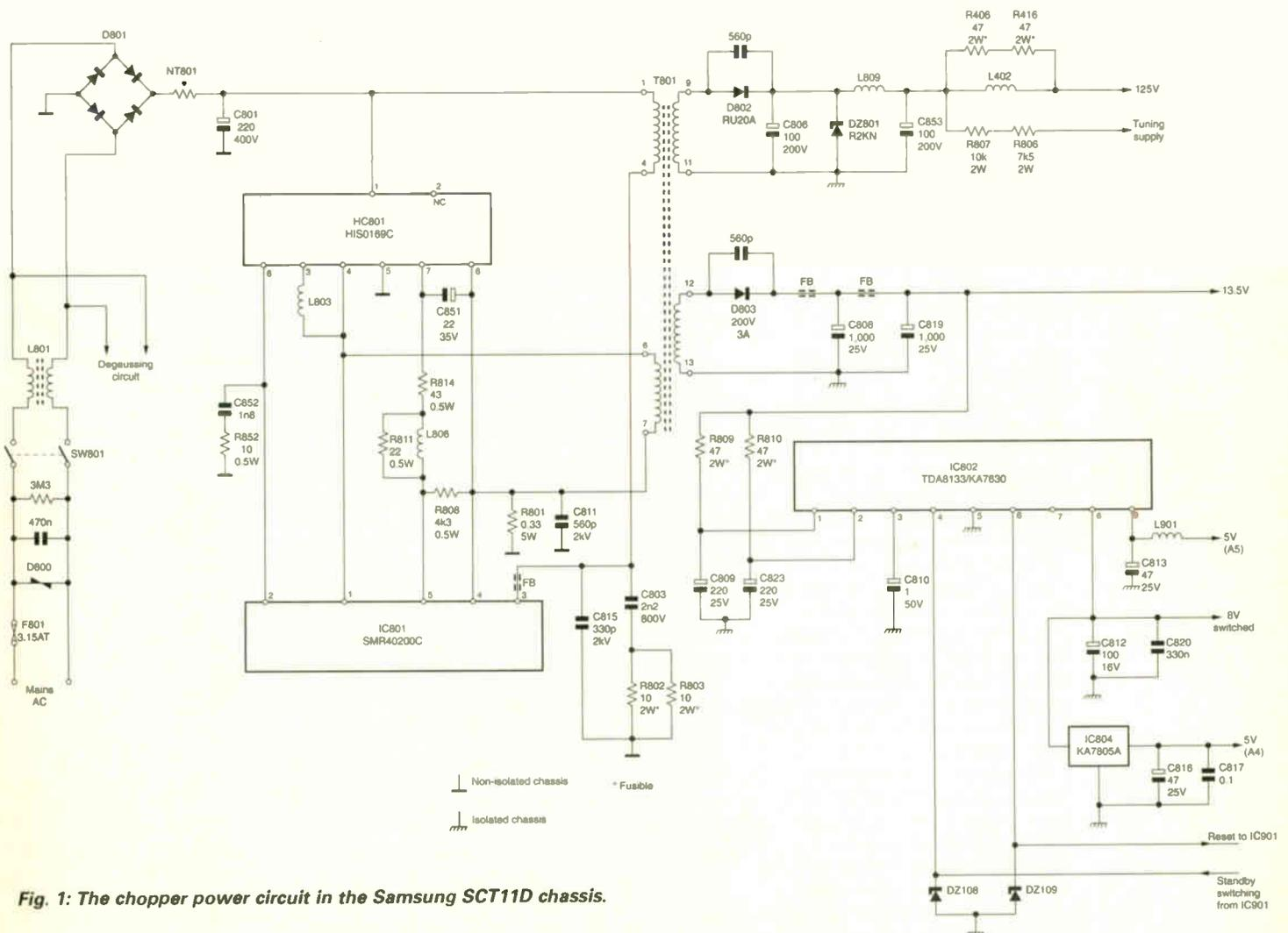
Fig. 1: The chopper power circuit in the Samsung SCT11D chassis.
