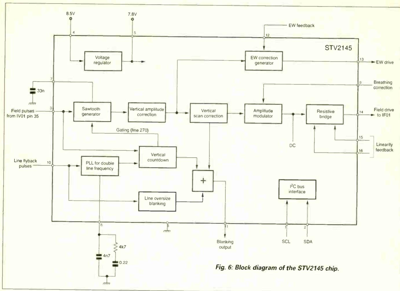
Fig. 6: Block diagram of the STV2145 chip.
