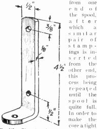
Fig. 265a. - Dimensions of supporting foot of Transformer.
