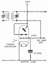
Fig. 469.—Connections for cathode-ray tuning indicator.
