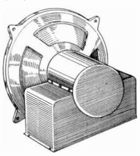
Fig. 241.—A mains energised Moving-coil Loudspeaker.
