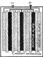
Fig. 28.—Section of a Heavy-duty type of Accumulator
