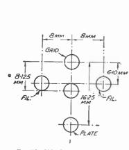
Fig. 458.—Valve-leg spacing for 4- and 5-pin valves. The diameter of the valve pins is 3.2 mm.
