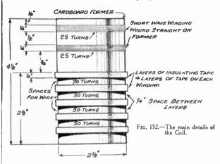
commenced. Drill two small holes in the first (bottom slot slot), thread the wire through several times to it. and secure leave about 6 in. of wire inside of the former for connecting up. Wind fifty turns in the first slot, then cross over and continue winding in second slot, cross over again from
