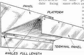
Fig. 87.—A metal Chassis using angle-irons instead of bending the aluminium.
