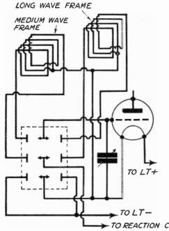
Fig. 384.—Three-pole change-over Switch used for wave changing with Frame Aerials.
