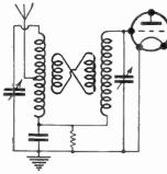
Fig. 439.—The Circuit of the "Link" Coupled Band-oass Tuner.
