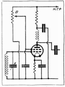
FIG. 167.—With the usual arrangement of a mains set the potentiameter acts as a decoupler.
