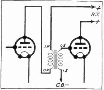
Fig. 162.—Transformer primary directly in anode circuit
