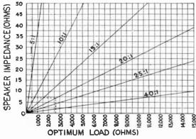
Fig. 303.—Graph for Moving-coil Speaker.
