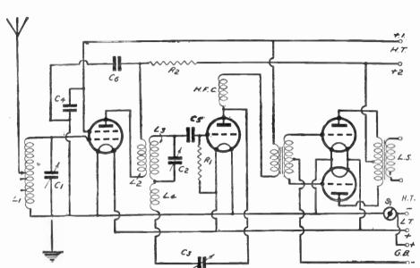
Fig. 114.—Circuit No. 16: Four-valve Circuit with two valves in Push-Pull.
