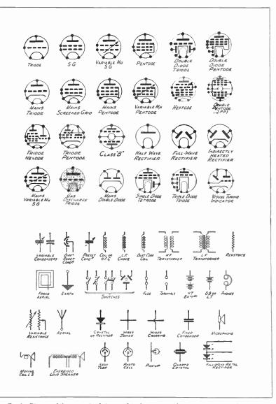
FIG. 1.—Diagram of the conventional signs used in drawing a wireless circuit, which merely consists of a number of these signs joined together. Pictorial diagrams showing the actual components represented are given in the book in their correct alphabetical order.
