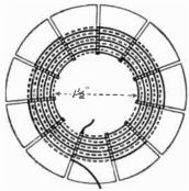
Fig. 126.—The Coil ready for mounting.
