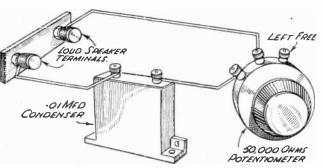
Fig. 291.—A high-note Filter—a cure for whistle, caused by heterodyning.
