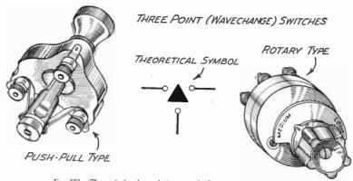
Fig. 373.—Theoretical and actual diagrams of a 3-point wave-change Switch.
