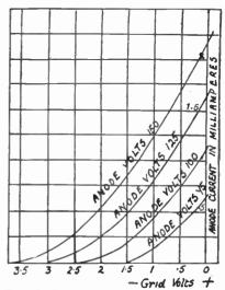
FIG. 465.—Characteristic Curve of a very High Impedance Valve.
