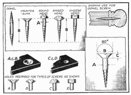
Fig. 484.—Wood Screw proportions and types.
