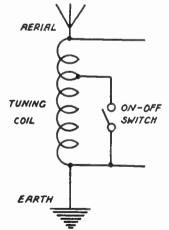
Fig. 377.—On-off Switch used for wave changing.
