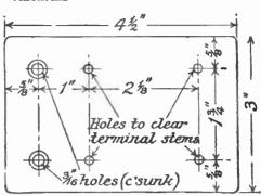
Fig. 45.—How to mark out the Eleonite Base.
