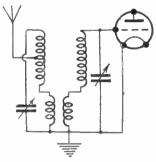
Fig. 454.—A Band-pass Tuner with com-mon Coupling Coil.
