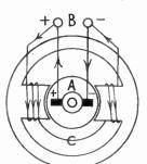
Fig. 14.—A shunt-wound 2-pole dynamo.
