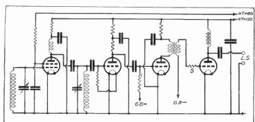
Fig. 165.—A typical four-valve circuit showing the method of inserting the decoupling resistances.
