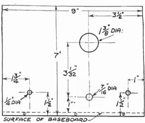
Fig. 182.—The Panel Layout for the D.X. Unit.
