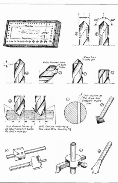
Fig. 176.—Various hints about Drills and Drilling.
