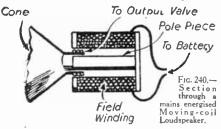
with a certain impedance in its anode circuit, and although valve manufacturers give this impedance figure in the leaflets accompanying their valves, unfortunately loudspeaker manufacturers do not always give the impedance of their products. Usually, only the D.C. resistance is given, and this does not enable one correctly to match up the speaker. There are on the market, however, certain out-
