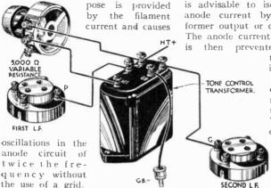
is advisable to isolate it from the anode current by either a transformer output or choke-filter circuit. The anode current of the last valve prevented from flowing
