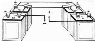
Fig. 5.—Accumulators connected in Parallel.
