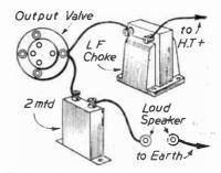
Fig. 354.—The Filter Output Circuit. See also Fig. 191.
