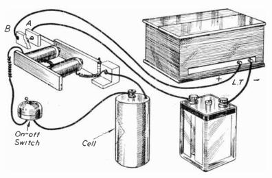
Fig. 352.—A Relay which consists of the Magnets and Armature of an electric bell.
