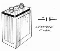
Fig. 3.—Theoretical and actual diagram of an Accumulator. Note that the thick line is always the negative in a theoretical diagram.
