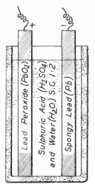
Fig. 19.—State of cell when charged,
