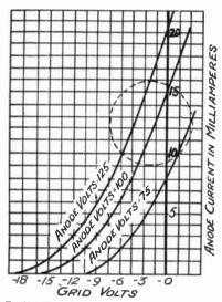
Fig. 80.—The ordinary grid-volts anode current curves.
