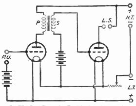
Fig. 205.—Circuit Diagram fos a Two-Valve Gramophone Amplifier
