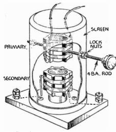
Fig. 145.—Variable selectivity is carried out in this 1.F. Transformer by rotating one of the windings.
