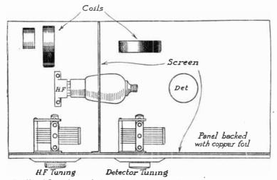
Fig. 226.—A Screen the same depth as the Baseboard is used for "partitioning off" the H.F. stage.
