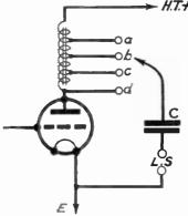
Fig. 306.—Choke-capacity Output.
