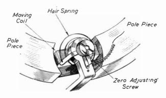
Fig. 269.—Perspective view of the active elements of a moving-coil instrument.
