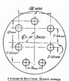
Fig. 459.—Valve-leg spacing for 7-pin valves.
