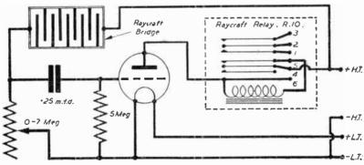
Fig. 229.-The circuit diagram for Light-Ray Control.
