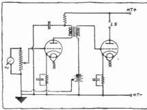
Fig. 208.—Mains version of Circuit shown in Fig. 207.
