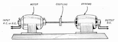
Fig. 7.—Diagram showing the principle of the Rotary Converter and Rotary Transformer. A motor, either A.C. or D.C., is driven from the mains and coupled to a D.C. generator which charges the arcumulators. In practice one machine acts both as motor and dynamo.
