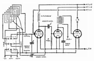
Fig. 110.—Circuit No. 13: Circuit diagram for a Three-valve Portable Set.
