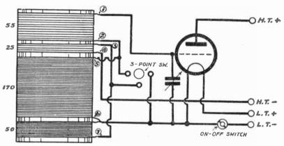
Fig. 480.—Diagram of coil connections for the Heterodyne Wavemeter shown in Fig. 481.
