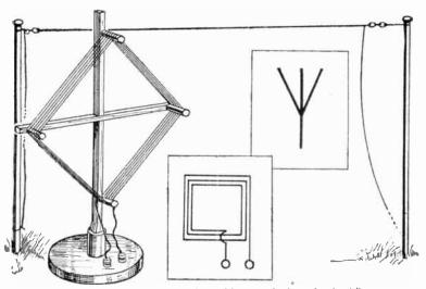
Fig. 40.—Conventional signs for outdoor and frame aerials, shown also pirtorially.
