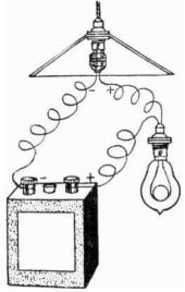
Fig. 208.—Simple Charging Arrangement from D.C. Mains.
