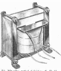
Fig. 2658.—One method of finishing off. Flexible leading-out wires are used.
