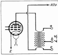
Fig. 305.-Transformer Output.
