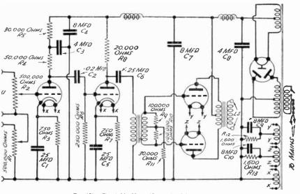
Fig. 120.-Circuit No. 22: A 12-watt Amplifier.
