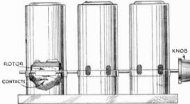
FIG. 389.—Three-gang Tuning Coil with self-contained Switch.
