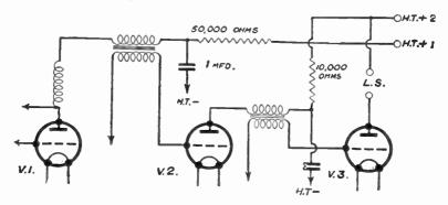
Fig. 184.—The Battery Connections of a simple three-valver.
