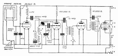
Fig. 119.-Circuit No. 21: A Four-valve Portable.
