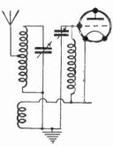
Fig. 450.—Inductive Band-pass Coupling.
