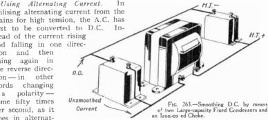
the high tension is derived for the Usually the inductance value of the choke is not less than 30 heuries and the capacity of condensers at least 4 mfds. each.
