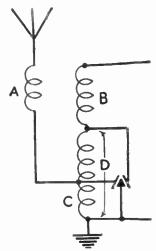
Fig. 69.—Another typical Dual-range Circuit,
