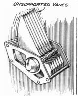
Fig. 293.—Vibrating condenser vanemay cause a microphonic howl.
