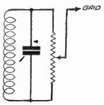
Fig. 478.—A Potentiometer across the Grid Coil.
