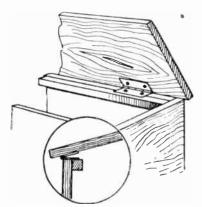
Figs. 75 and 76.—This is the simplest method of fixing the lid by means of hinges. The detail shows the extra strip for strength.
