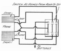
Fig. 111.—The Switch Connection to the Aerial of Circuit No. 13.
