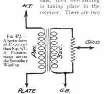
remedies for overloading—one is to increase the handling capabilities of the valve by applying more H.T., and the other is to cut down the signal strength.
