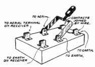
Fig. 35.—The method of connecting up the Lightning Switch.
