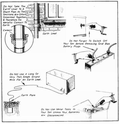
Fig. 302.-Various simple tests to apply, and causes of trouble.
