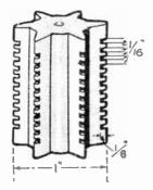
FIG. 215.—Method of cutting ebonice former for the H.F. Choke.
