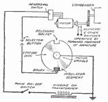
Fig. 349c.—Some forms of automatic tuners are motor driven, the basic principle being as shown here.
