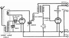
Fig. 105 .- Circuit No. 8: Circuit for a Short-wave Two-valve Set.
