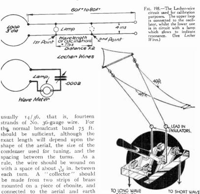
Fig. 198a.—A duplex aerial arrangement for long and short waves.
