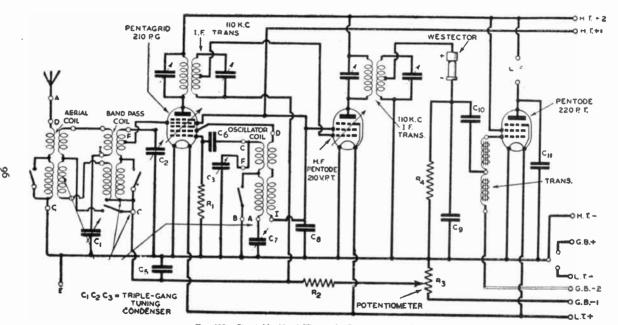
Fig. 108.—Circuit No. 11: A Three-valve Battery-operated Superhet.
