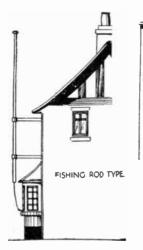
Fig. 197.—A "fishing-rod" type of ventical aerial.
