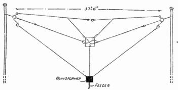
FIG. 47.—The Spider-web anti-interference aerial.
