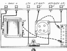
Fig. 121.-A One-valve Amplifier.
