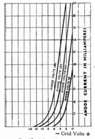
Fig. 467.-A Steep Slope Valve Curve.
