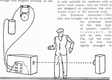
Fig. 235.—The connections for the invisible-ray burglar alarm.
