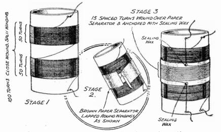
Fig. 49A .- Constructional details of the transformers for anti-interference a rials.
