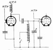
Fig. 451.—The Tuned Grid system.
