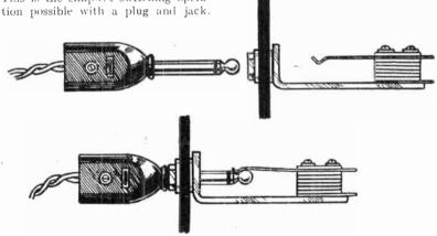
Fig. 327.—How the Plug and Jack connect.
