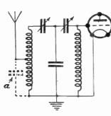
Fig. 438.—The Circuit arrangement of the Band-pass Scheme.
