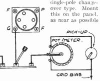
to the grid terminal of the valve holder to which you wish to connect the pick-up. Now disconnect the wire which goes to this grid terminal, and connect it to one side of the switch. Connect a wire from the grid terminal of the valve holder to the arm of the switch, and from the remaining
