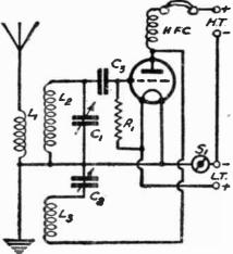
FIG. 98.-Circuit No. 1: A simple One-valve Circuit.
