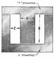
Fig. 2648.—Illustration of the Transformer Stampings to be used in conjunction with the table on p. 238.
