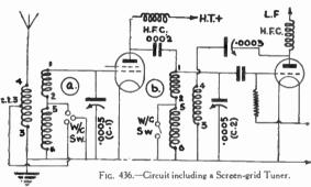
of small angle brackets. The latter method makes the tuner suitable for single-hole panel mounting, the switch bush being used for mounting purposes. Where it is preferred to use a cardboard or paxolin former, the same numbers of turns will be approximately correct and the same spacing between the ends of separate windings should be allowed. As, however, all three windings will have to be wound as single layers, the length of former must be increased.
