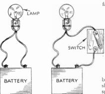
Fig. 390.-How the on-off Switch functions.
