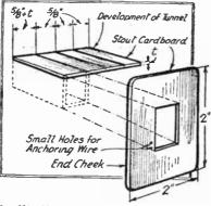
Fig. 221.—How to make the winding bobbin from paxolin sheet for chokes and transformers.
