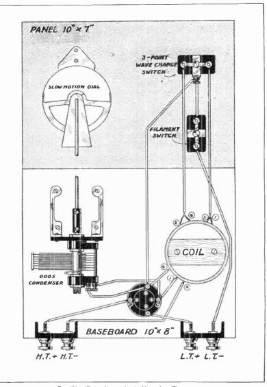
Fig. 481.—Wiring diagram for the Heterodyne Wavemeter.
