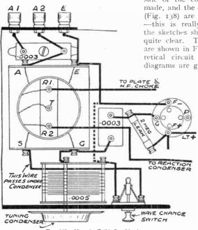
Fig. 141.—How the Coil is fitted in the set.
