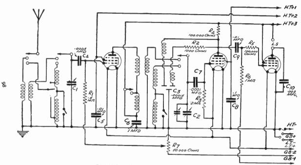
Fig. 109.—Circuit No. 12: An All-wave All-pentode Battery Receiver.
