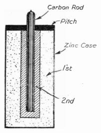
Fig. 470.-Section of a Dry Cell.
