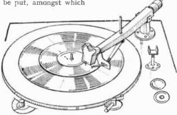
Fig. 310.—The Recorder as a reproducer. The Tracking Arm is cut of action, and weights are placed on the back of the arm.
