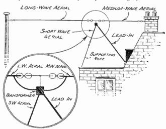
Fig. 48.—All-wave anti-interference aerial.
