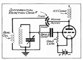
Fig. 171.—The method of connecting a differential condenser when the reaction coil is joined to the earth line.
