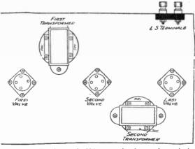
Fig. 228.—The Transformers should be mounted as far away from each other as possible to avoid interaction between them.
