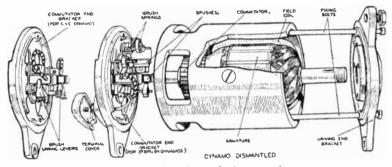
Fig. 12.-A car lighting dynamo, showing construction.
