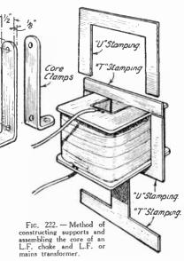
since arrangements have to be made to provide the necessary air gap. This is easily done by fitting all the "T" stampings into the spool from one end, and then arranging all the "U" stampings opposite to them. The necessary gap is fixed by slipping strips of card  $\gamma_{\theta}$  in, thick between the ends of the "U" stampings and the sides of the "T's." Additionally, to prevent the gap being short-circuited, slips of paper must be placed between the core clamps and the core itself.
