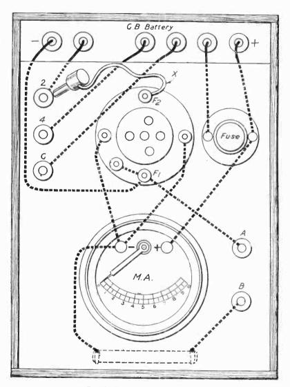
Fig. 468.—Wiring diagram of the Valve Tester.
