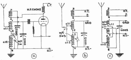
Fig. 435.—Three methods of connecting the Tuner shown in Fig. 434 into a Detector Circuit.
