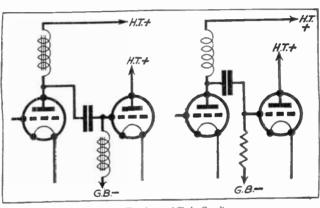
Fig. 164.—Two forms of Choke Coupling.
