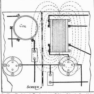
Fig. 226p.—The placing of a Transformer near a Coil (even if there is a Screen) is bad-
