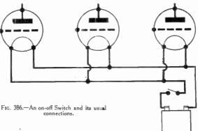
burn them. If, however, the contacts snap apart quickly the spark is of such short duration as to do no damage.
