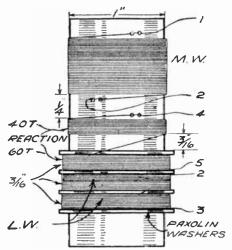
Fig. 148.—Constructional details of an efficient oscillator coil.
