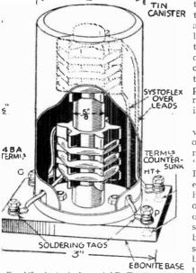
Fig. 143.—A simple form of I.F. Transformer in which variable coupling can be introduced.
