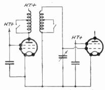
Fig. 453.—A H.F. Transformer with wave-switching.
