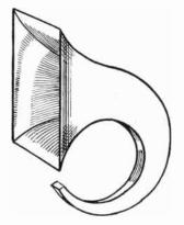
Fig. 248.—A method of curving which avoids bends.
