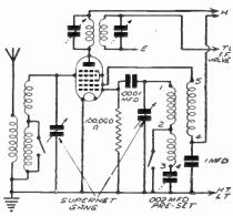
Fig. 149.—Here is the circuit of the frequency changer stage of a superhet employing an I.F. of 110 kc/s.
