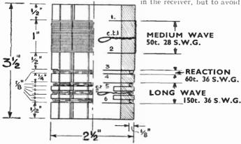
Fig. 434.—Constructional details of a Tuner made on an eight-ribbed 21-in, diameter Ebonite Former. All turns are wound in the same direction.
