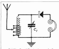
Fig. 96.—Crystal Circuit using tapped coil. List of Components for Fig. 96
