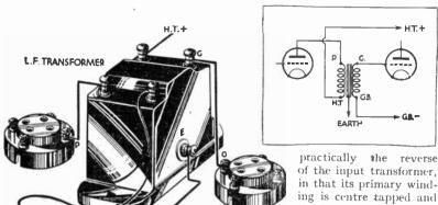
Fig. 258.—L.F. Transformer Coupling.
