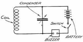
Fig. 479.-A Buzzer Wavemeter.
