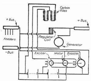
Fig. 67.—Arrangement of Automatic Reversible Booster.
