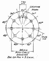
FIG. 460.-Valve-leg spacing for 9-pin valves.
