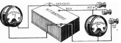
Fic. 270.-Voltmeters for checking different values of high tension.
