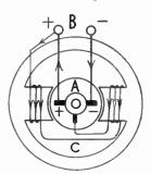
Fig. 15.-A constant voltage dynamo.
