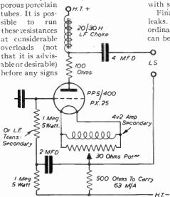
Fig. 359.—An Output Valve which is Mains Operated, and the Power Rating of all Resistances which are included in the Circuit.
