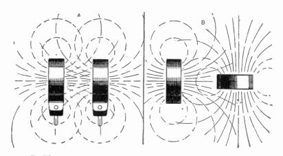
Fig. 225.—Showing the shape of the electro-magnetic field of coils of the usual plug-in type.
