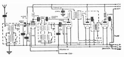
Fig. 117.-Circuit No. 19: A Single Four-valve Battery Set.
