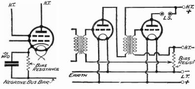
Fig. 60.—The biasing resistance arranged in the cathode lead of a S.G. valve.
