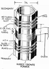
Fig. 146.—A third winding is used in this I.F. Transformer to control the degree of selectivity.
