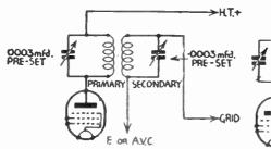
Fig. 142.—In this H.F. Transformer coupling between the two windings is carried out inductively.
