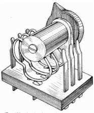
Fig. 382.—Another form of low-capacity Switch.
