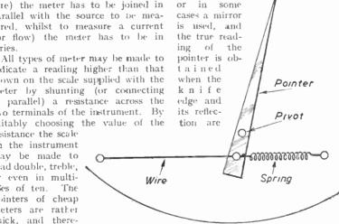
Fig. 268.—Elements of a hot-wire instrument. View showing Spring, Bearing and method of making connection.
