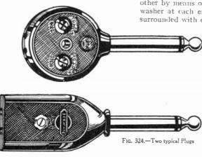
Construction of the Plug. For those who are not familiar with the elements of jack switching an explanation of the construction of the plug and jack and how they work will not be out of place. Fig. 324 shows two popular plugs. The
