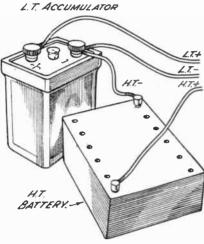
Fig. 230.-The Battery Connections.
