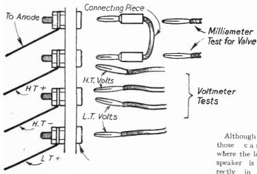
Fig. 273.—Fitting Sockets on the Panel enabling the milliammeter and voltmeter tests to be made from the exterior of the set.
