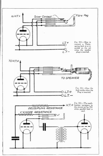
which would normally be joined to the "L.S." terminals are connected instead to the two tags of the jack. from the set, or from the set to the first point, and from there to the next one, and so on. Use whichever ar-
