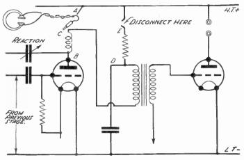
FIG. 300.—How to test for "crackling" noises. To test the H.F. and detector stages disconnect H.T. from E and join phones across A and B. To test H.F. choke as well join phones across A and C. To include transformer join them across A and D. To include decoupling resistance ion across A and E.
