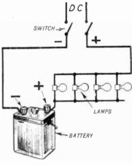
Fig. 2Nc.-The complete Charging Circuit,
