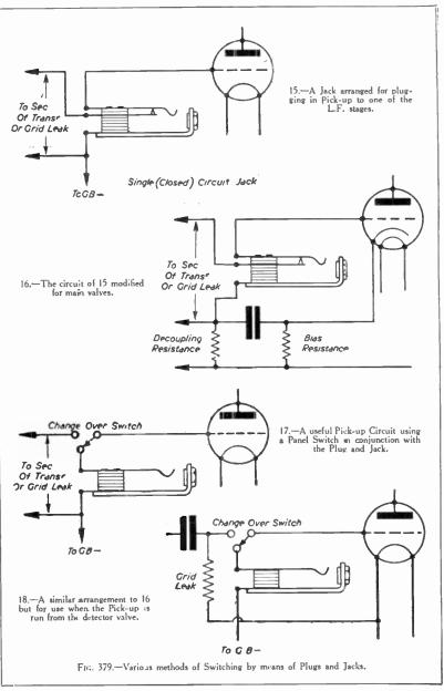
forces the pairs of springs in contact, or allows them to separate according to its position. It thus makes and breaks t h e circuit. This special type has two sets contacts so that two circuits are dealt with at once.
