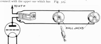
Fig. 329.—Speaker Points can be arranged in different rooms by means of Wall Jacks.
