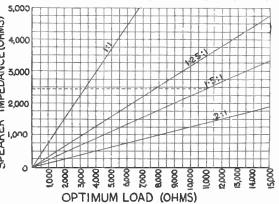
Fig. 304.—Graph for Moving-iron Speaker.
