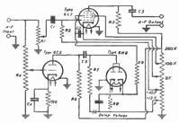
Fig. 478a.—Circuit incorporating Volume Expansion.
