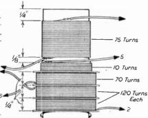
FIG. 151.—Here are the details for an oscillator coil for use with the I.F. transformer shown above.
