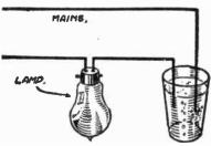
Fig. 17.—Dissolve a teaspoonful of salt in a glass of water and dip the ends of the charging wires in the solution. Bubbles of gas will form on the negative wire. (See also Figs. 26 and 27.) Take care that the two wires do not touch one another.
