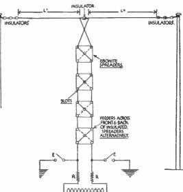
FIG. 197A.—Transposed or horizontal doublet aerial. E=earthing switches. CC=coupling coil. RR=600-ohm resistances. L¹,  $L^2=40$ -ft. aerials.
