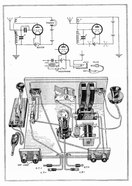
Figs. 426 and 427.—A 1-Valve Transmitter, with circuit showing how it differs from a 1-Valve Receiver. P.W.E.— $\cdot$ M 345
