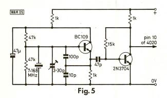
At first the author used the circuit in Fig. 5, but found it needed the second transistor as a buffer amplifier. This didn't seem very economical in terms of components, so the much simpler circuit of Fig. 6, was tried and found to be satisfactory. It was after I had gradually found the component values by the "select on test" method (i.e. suck it and see), that I was told that an almost identical circuit was in the Vol 2 of the
