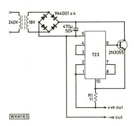
The construction of the circuit is not critical, except that it is worth noting that the external transistor should be mounted externally in free air, no heat sinking at all has been found necessary at the fairly low power involved. For preference, the unit should be run from a 3-pin supply, and all exposed metal earthed. The transistor may be covered with a suitable plastics cover available for this purpose.
