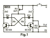
The circuit in Fig. 1 is a standard cross-coupled multivibrator and R1 will adjust the frequency whilst R2 will adjust the deviation to the amount required. Its advantage is cheapness and simplicity, and if good quality components are used it should not drift far with the changes in temperature.
