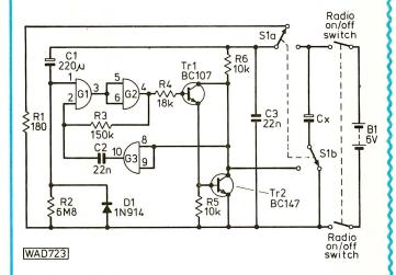
When listening to a radio in bed, it is frequently left on all night after the listener has long since gone to sleep. This circuit was designed to turn off a 6V transistor radio after approximately half an hour. It is also suitable for 9 and 12V radios, but will work as low as 3V.
