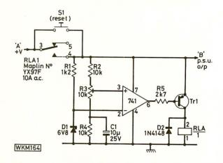
The function of the  $10\mu F$  electrolytic (C1) is to prevent any occasional "spikes" from tripping the relay. Resistor R5 is a base-current limiting resistor. The resistance of the coil of the relay is about  $400\,\Omega^-$ . Diode D2 protects Tr1 from the back e.m.f. from the relay coil.
