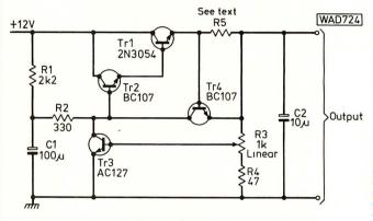
The voltage drop across R1/R2 is determined by the voltage applied to the base of Tr3. As Tr3 conducts, more current is drawn through R1 and R2, which lowers the voltage drive to the series transistor and decreases the output voltage. When the slider of R3 is rotated towards R4, Tr3 is cut off, thus drawing very little current through R1 and R2, increasing the output voltage.
