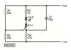
When the capacitor has been discharged the only source of current for the s.c.r. is through the resistor R4. The value of this current is below that required to keep the s.c.r. in a turned on state and thus it switches off, allowing C4 to start charging up and the cycle to repeat.
