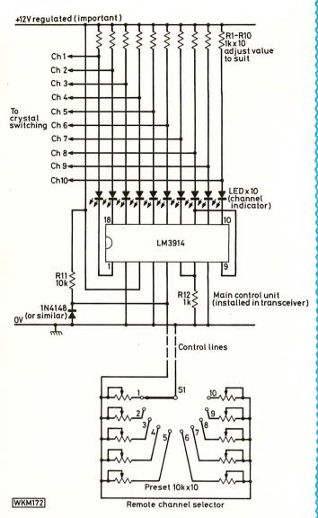
(4) For more than 10 channels the LM3914 can be cascaded; you could use anything up to 10 i.c.s giving you 100 channels. Four LM3914s are required for the 40 CB channels.
