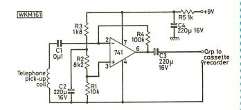
The actual quality depends on the sound circuits in the set but the usual limiting factor is the cassette recorder. As the adaptor picks up sound from the TV loudspeaker it will work with any TV set, 625- or 405-line, and of course from the loudspeaker of a radio as well.
