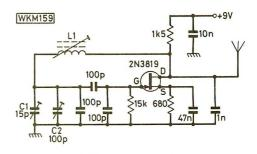
A strong s.s.b. signal (very distorted) is found on the main receiver around 7MHz and the speech resolved by slowly tuning the unit. This technique (similar to using reaction) requires patience at first but is capable of surprising results.
