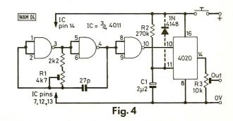
pressed in. The values of R2 and C1 have to be found by experimentation because of the notorious lack of accuracy of electrolytic capacitors, but the author found  $270k\Omega$  and  $2\cdot 2\mu F$  (tantalum) gave reliable results. As with all the circuits, good quality components will greatly aid the stability.
