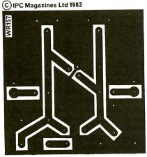
In both circuits I have used single-sided glass-fibre board and all components are mounted on the copper side. I used ordinary ceramic 1nF capacitors for the line decoupling instead of the feed-through types. I found feed-through capacitors hard to obtain, and with my layout no drilling of the board is required.
