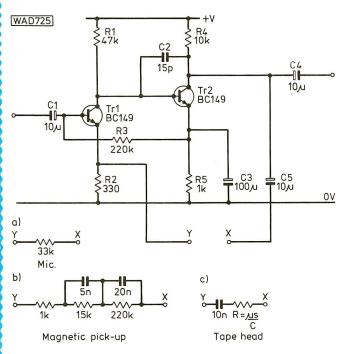
The pre-amplifier has proved useful over the years for matching low-level signal sources into amplifiers without suitable inputs. A feedback pair of transistors is a very common arrangement for a pre-amp.
