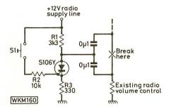
Having chosen the desired radio programme with volume set reasonably loud, set the alarm and set the sleep timing. The push-button is then momentarily operated causing a considerable volume reduction. Once the radio has (automatically) turned off, the latching circuit will be released and when the radio "alarm" is energised the volume will be at the previous higher level.
