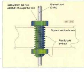
Fig. 5: Wilko Melenhorst uses a simple, but effective fastener for the elements on his long Yagi antenna, making it quick to assemble and strip apart.
