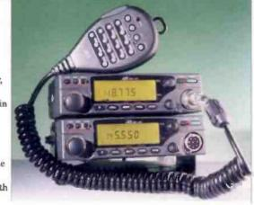
The new ADI AR-147 transceiver (top) and older ARthere will still be many 146 (bottom). The AR-147 covers 144MHz and provides 'receive only' on the 'Air Band'.
