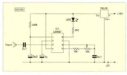
Fig. 2: Circuit of the audio frequency 'Tone Detector' project (see text).
