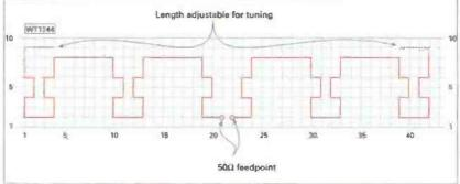
Fig. 2: The wire arrangement on a length of plastic netting (with 50mm - or two inch 'holes') used to make the 28MHz fractal dipole. At the dipole ends enough wire is left to trim the antenna to resonance. The complete fractal dipole can be built on a length of netting which is a considerable length reduction over a normal half wave antenna for the band.
