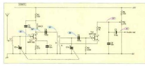
Fig. 3: Test points on the regenerative detector receiver, Receiver 3, with r.f. amplifier (t,r.f.). See text for details on 'anti-swamping' procedure adopted for testing purposes.
