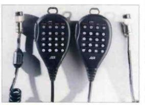
Fig. 1: Close-up photographs of the ADR microphones, clearly illustrating the complex functions provided (see text for comments on repeater working). The newer AR-147 microphone (left) is provided with a ferrite sleeve.
