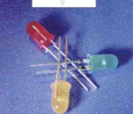
Fig. 3: You can use a colour of your own choice for the l.e.d. in the circuit ... but remember that the longer lead goes to the positive (+) supply).
