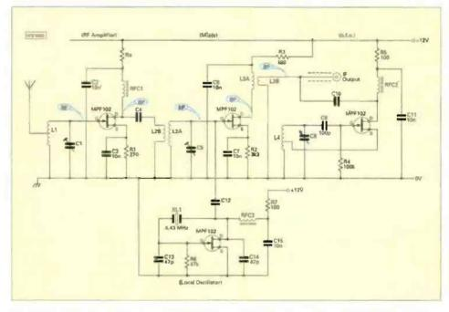
Fig. 4: Test points adopted for use on the 3.5MHz to medium wave converter project (Receiver 4). See text for details on testing car radio i.f. unit and 'sniffer probe' used for checking oscillator output.
