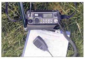
Fig. 2: Phil MOAYB uses a Yeesu FT-290 Mkll 2.5W portable transceiver for his portable contesting.
