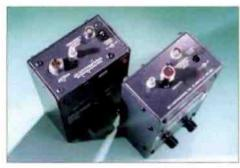
The MFJ-269 on the left with the MFJ-2598 to its right shows that the modifications are more noticeable on the top panel. Note that the output socket is now an N-type rather than the SO-239 of its forerunners.
