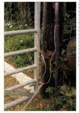
A metal oate set on a wooden nost could be a suitable hidden antenna, Note: the wiring joints are for illustration purposes only and should be far more secure in a permanent installation. (For use in vou own property only for safety reasons).
