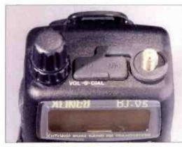
Fig. 2: Top view of the Alinco. ".... the antenna connection is an SMA type and the radio has the famillar 3.5/2.5mm Jack socket-pair for the speaker/microphone extension on the top of the transceiver".
