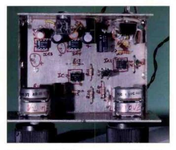
Fig. 3: An overhead view of the prototype Morse Stager showing component placing. (Refer to the overlay diagram of Fig. 4, for more detail).
