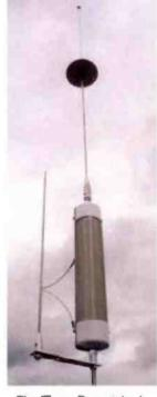
The Texas Bugcatcher' h.f. mobile antenna, with large diameter loading coil, capacity 'hat' and the vertical 50MHz 'add-on' element. is so easy to assemble and install that it's possible to ignore the 'photographs' and just get on with the job! And bearing in mind I wear an artificial arm, assembling the system only took me a few minutes.
