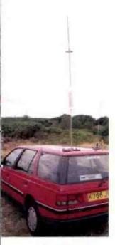
Fig. 2: Rear 'side on' view of G3XFD's car to illustrate the size of the 'Bugcatcher'. finish of the 'capacity hat'. It seemed to be made of very thin and vulnerable aluminium - although I realise of course that this factor may well be dictated to the designer because of the capacity required.
