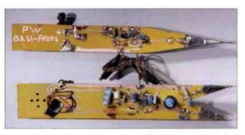
Fig. 5: Partners in detecting 'Crime' (faults!). The completed PW 'Basi-Probe' and 'Basi-Tracer' units.
