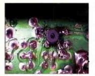
Fig. 1: A picture provided electronically by Shane GONCF, of how the replacement dual gate m.o.s.f.e.t. is fitted into his FT-107.
