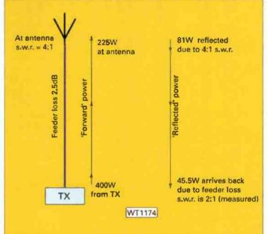
Fig. 2: Showing the conditions involved when the s.w.r: measured at the transceiver/feeder interface is lower than the real s.w.r. at the antenna/feeder interface.
