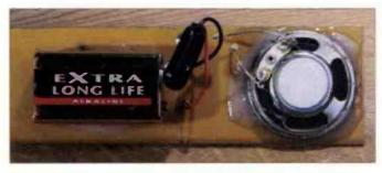
Fig. 4: Photograph showing simple method of attaching battery and small loudspeaker (1.5in, 38mm diameter) to the rear of the p.c.b. using rapid setting epoxy resin adhesive. Take care that the adhesive does not 'run' under the speaker rim onto the paper cone, but only onto the metal rim of the speaker frame.
