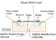
Fig. 1: Structure of a depletion mode m.o.s.f.e.t.
