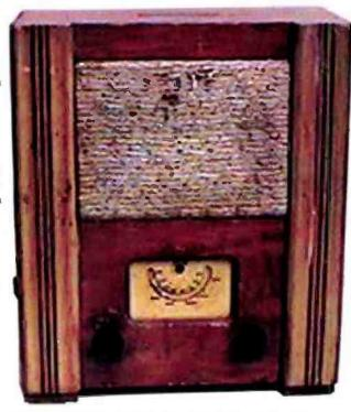
Fig. 1: An unwanted 'War Baby'? Charles Miller takes a look into the history and difficult 'gestation' of the Second World War 'Utility' receiver. The version shown was made by A. C. Cossor Ltd. Westinghouse metal rectifier could have been used !
