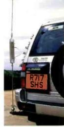
3 inch diameter open coil with adjustable taps for each band. The antenna has a total of length of 229cm and features a "quick disconnect top whip with
