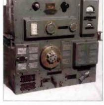
Fig. 1: The Saram 3-10 transmitter. The two doors either side of the large central tuning dial open to reveal the valves for the set.
