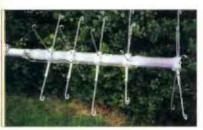
Fig. 3: The resonator adjusters on the end of the elements, showing construction of the resonators with their spokes and adjusters.
