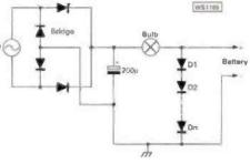
Fig. 5: A simple **NiCad battery** charger based on Fig. 4. (see text).
