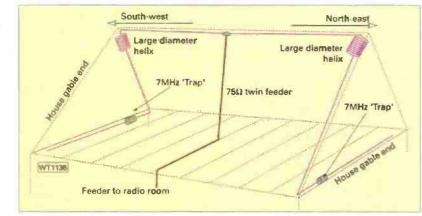
maintained between the antenna and other conductors. Endeavour to run the antenna along the inner apex of the roof space, as high up as possible and keep the feed point (of a dipole) midway along the apex.
