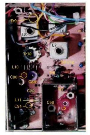
Close-up of the main oscillator and pre-PA r.f. stage area of the 'main' board.
