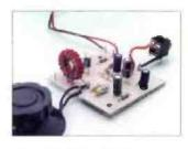
Fig. 8: The built-up Novice Receiver from Lake Electronics. See text for more details.
