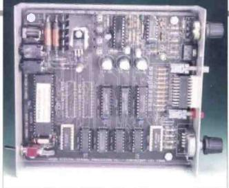
Inside of W9GR DSP-III DSP filter unit.
