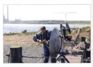
'EN is transmitting on 1312MHz with a pair of directional 'Bow Tie' antennas to concentrate the outgoing radiation pattern towards the north and south of the repeater site at the Enfield Civic Centre.
