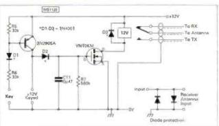
When the key is pressed and 12V appears at the collector of the 2N2905A, the VN10KM switches on and the capacitor (C11) charges up. When the key is released and the 12V disappears from the collector and the capacitor discharges through the resistor (R7). This holds the VN10K on for a short time.
