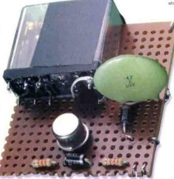
changeover unit assembled using perforated matrix board (see text).
