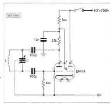
Fig. 1: Circuit of the valved grid dip oscillator using the EM85 'magic eye' indicator (see text for further information on coils, etc.).
