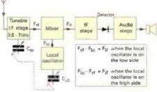
Fig. 2: The simplified block diagram of a superheterodyne ('superhet') receiver
