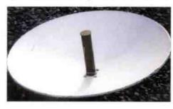
Fig. 5: A 460mm diameter dish (originally made for the PW EXE) with penny feed.
