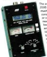
259B saves you so much time. Just conect to the antenna or coax leed and read of the resonant frequency, VSWR and impedance. Ideal for field work. Use it with internal dry cells (not supplied) or run it from an external
