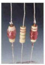
Fig. 3: Winding 'home-brawed' radio frequency chokes on resistor bodies (see text).
