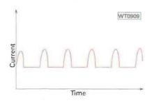
Fig. 2: The current consumption of a Gunn diode showing the current pulses.
