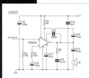
Fig. 1: Circult diagram using the TBA820M i.e. (see text).
