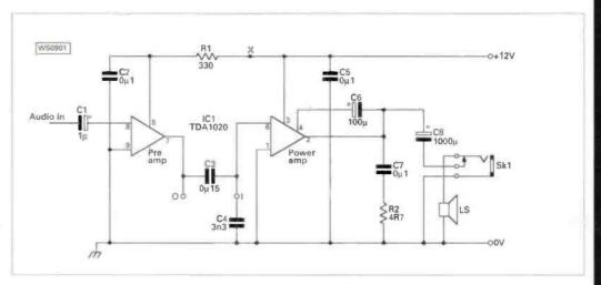
The greatest advantage for our sort of application is that the pre-amplifier and the power amplifier are separate. The output from the pre-amplifier and the input to the power amplifier both come out on pins.
