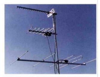
Antennas used by Graham Hankins G8EMX for portable ATV contests. From top: 24, 70cm and 2m for ATV calling. Note: even the 2m antenna is mounted horizontally. Larger antennas would be preferable.
