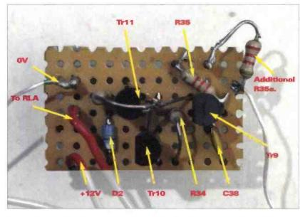
Fig. 5: A small section of Veroboard was used to make up the transmit/receive changeover circuit.
