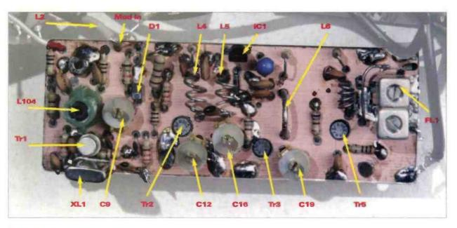
Fig. 3: The transmitter board overlay.
