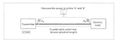
Fig. 2: To find the loss figure, measure the available power at each end of the length of cable, and divide the loss (in dB) by the length of the cable.
