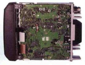
Don't be misled by the apparent lack of 'active ingredients! In fact there's a large component count on this **Impressive** p.c.b. due to the intensive use of the extremely versatile surface mount' devices.
