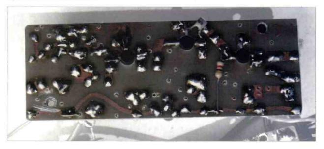
Fig. 4: As space is tight a few components must be mounted on the track side of the transmitter p.c.b.
