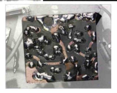
Fig. 2: The underside of the microphone amplifier board.
