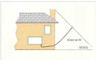
Fig. 5: A sloper antenna for 14MHz could be set up in even a small garden.
