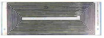
components and parts, a large(ish) box made from two interlocking. 'U's and two soft 'aluminium' facia panels. There was also a rather strange flat coil made from a piece of p.c.b. material with the tapped, rectangular coil etched on it. To complete the kit of course were the instructions. comprising six double-sided A4 sheets stapled together.
