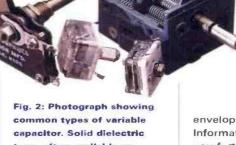
common types of variable capacitor. Solid dielectric type, often available as surplus (left), modern Polyvaricon types (centre) and traditional double ganged 'air spaced' from a broadcast receiver.
