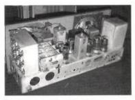
Fig. 3: The inside of the R-103 Mark 1. The coil pack and tuning components are on the left of the picture, with the i.f. stages in the middle. The vibrator power pack is mounted on the right hand side of the chassis.
