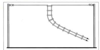
Fig. 2b: Feeder imbalance caused by the feeder not dropping vertically.
