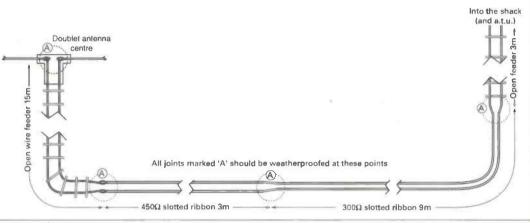
Fig. 1: How John G3BDQ, used different types of feeder for his Doublet Antenna.
