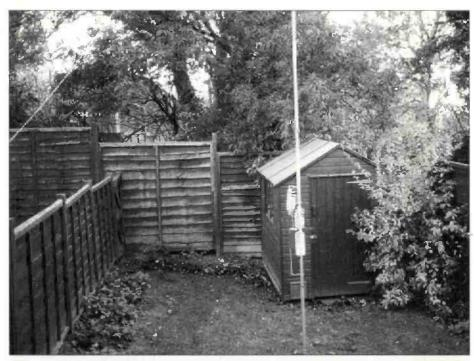
The garden of the QTH at Hastings used on weekdays for two years by G4BUE. The 'postage stamp' sized back garden was just big enough to put up a Butternut HF6V vertical antenna, (3.5, 7, 10, 14, 21 and 28MHz) which with 100W from a TS-440 enabled Chris to keep up his DXing.
