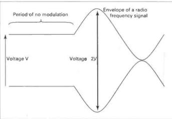
Fig. 2: An a.m. signal with 100% modulation.
