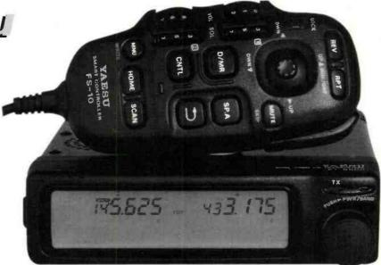
The FT-8500 dual - band mobile transceiver with accompanying 'Smart Controller'.
