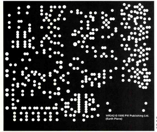
Fig. 4: Groundplane details for the p.c.b. But, without the tuning capacitor connected and the p.c.b. 'naked' on the bench it won't be a usable receiver yet. Despite this it should be apparent if the receiver seems to be working, or else needs some further soldering and
