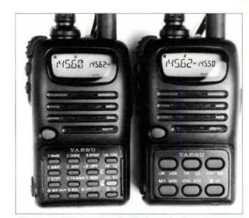
Photograph illustrating the choice of keyboards available on the FT-10R (see text).
