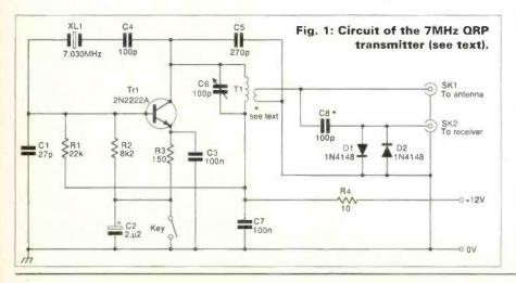
check the wiring and apply 12V, not forgetting that a dummy load  $50\Omega$  resistor should be across the output. The output can then be measured with a diode probe.
