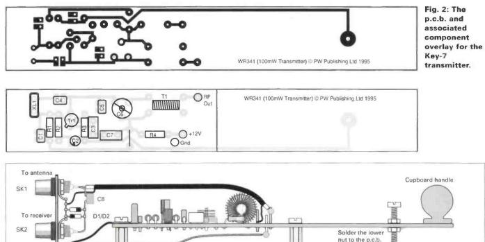
Key contact connects through the screw to the OV side of the p.c.b.
