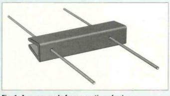
Fig. 1: A spacer made from a section of spine binder (see text).
