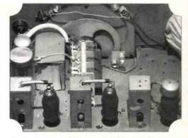
Fig. 6: The well-known Philips PCR receiver used the attractive looking series of Mullard 'Red' valves (see text).
