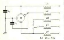
Fig. 4: Supression circuit for windscreen wiper motor interference (see text).
