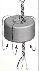
Fig. 2: Showing the stages in making T1, the turns are spread around the toroid as illustrated. Connections are as follows: A' to Tr3 drain and bottom of R15, A to B', B to R9/R15/C6/D1 junction, C' and C go to chassis and the output respectively.
