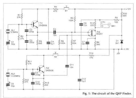
14.060 and 3.5MHz together to produce 21.060MHz.
