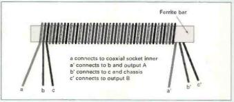
balanced line output with a special transformer. In short, this balanced to unbalanced transformer system is usually called a balun.
