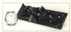
Walford Electronics have recently added a new kit to their range which designer Tim Walford G3PCJ says will be of interest to keen home constructors and designers. The **Reference** kit has been designed to provide a range of highly accurate reference frequencies for use in counter timebases with an optional wide bandwidth **Input** h.f. amplifier and u.h.f prescaler. The Reference kit can be used on its own, or with the Walford Electronics two channel Frequency Counter.
