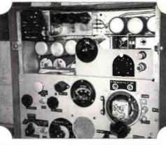
Fig. 5: Close-up view of 52 set, showing crystal calibrator unit (top left).
