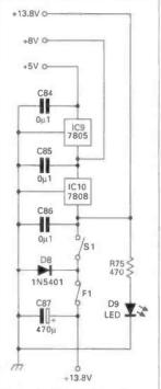
Fig. 1.7: Stabilised power supply circuitry (see text).
