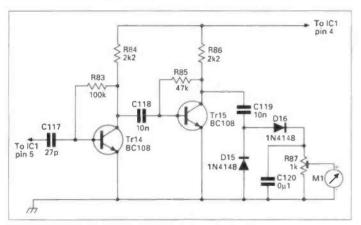
Fig. 1.9: (Left) Signal strength meter circuitry (to be described in Part 2).
