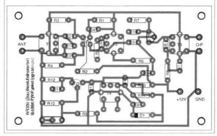
Track pattern and overlay for WR330, the receive converter section of the project. Note the earth plane has been left off for clarity.
