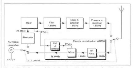
Fig. 2: Block diagram of the full project. The boxed section labelled as being on WR330 is the receive converter partly dealt in this issue.
