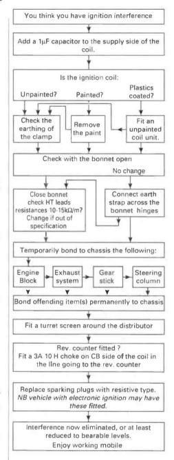
Fig. 1: Interference fault 'flow chart' (see text).
