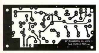
Fig. 7: Printed circuit and component overlay for the power amplifier.
