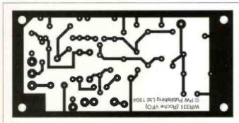
Fig. 6: Printed circuit and associated component overlay for the Roche v.f.o.
