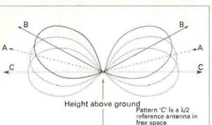
Fig. 2: Compare these superimposed radiation patterns of: A a  $\lambda/2$  dipole ( $\lambda/2$  above earth), B a 1/4 vertical antenna and C a reference  $\lambda/2$ antenna in free space. The angles C-A and C-B will depend on the quality of the earth and, in the case of the  $\lambda/2$  above earth, on how far it is above earth.
