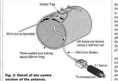
Cut two lengths for each antenna, to the lengths shown in **Table 1**. Allow some extra wire in each element to fold back and secure, by soldering. I bored all the holes with the aid of a hot nail that I held in a pair of lock jaw pliers.
