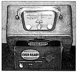
Fig. 6: The Ever Ready *Sky Queen* portable valved receiver, which utilised 90V h.t. valves and a 1.5V filament supply, with its associated battery (see text).
