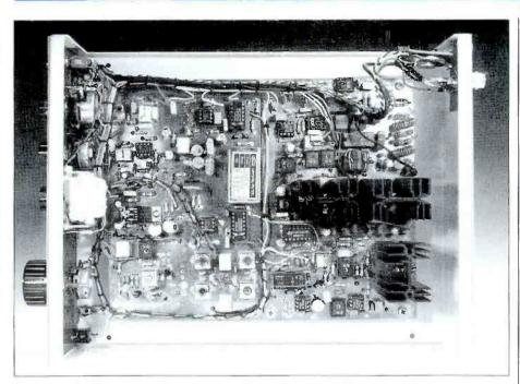
Fig. 1: An inside view of the completed Yeovil 3.5 and 14MHz s.s.b./c.w. transceiver built by G4SLU from the kit designed and supplied by Tim Walford G3PCJ.
