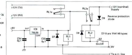
Fig. 2.1: The basic switching circuit used in the PW Jubilee showing the 9V regulated supply for use in the project, plus reverse polarity protection (see text).
