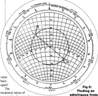
reciprocal values of measured values, can then be converted mathematically if required. But I find it easier to use a Smith Chart. To use this method, mark the admittance value on a Smith Chart, then draw an s.w.r. circle with the radius equal to the distance between measured admittance mark and the centre of the chart. The impedance value is diametrically opposite on the s.w.r. circle as shown in the example of Fig. 5).
