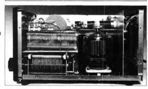
Fig. 2: The 'final' power for the AL-80BX unit is provided by a 3-500Z valve, with a warm-up time of 10 seconds.
