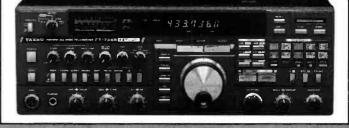
YABSU PT-736R This transceiver from Yaesu incorporates up to 4 band modules covering the 50, 144, 430 and 1200MHz Ham bands. The standard model provides 25 worlds RF power output on the 144 and 430/440MHz bands in SSB, CW and FM modes with any 2 of the remaining 3 bands as options (10 watts output on the 50 and 1200MHz bands). An 8-bit CMOS main micro-processor and 4-bit I/o coprocessor provide exceptional digital integration and control.
