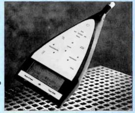
low cost front-end for tape recorders, transferring signals via an unweighted, calibrated a.c. output for spectrum analysis. There is an internal memory that can store results from up to 40 survey locations and for six hours (expandable to 24 hours) of one second results.
