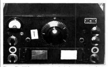
Fig. 4: The HRO receiver, a classic design originating from the 1930s.
