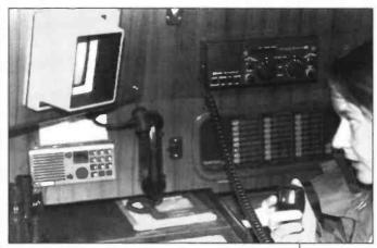
Fig. 5: A typical commercial marine band s.s.b transceiver aboard a large modern yacht.
