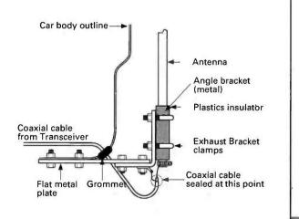
Fig. 2: Alternative method of mounting antenna bracket (see text).
