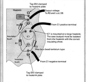
Fig. 2: Diagramatic (pin-side), view of IC1, and most of the other components, mounted on a large heatsink. It is important that the LM338K integrated circuit is insulated from the heatsink.
