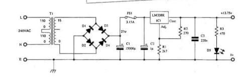
Fig. 1: The circuit diagram of the power supply. Capable of being made to give different output voltages. See the text for more details.
