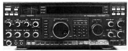
receiver performance utilising quadruple conversion, Yaesu's exclusive DDS, IF notch, IF shift, IF variable bandwidth, CW APF, independent mode and IF filter selection.
