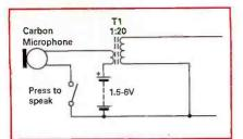
Fig. 2 (above): The alternative carbon microphone circuit (see text)
