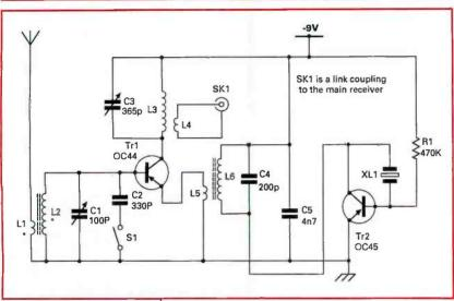
Fig. 4: A simple and efficient crystalcontrolled converter, which enables the 1.8MHz band to be received on a car radio. Coil details are provided in Table 1 opposite. As the unit is link-coupled into the receiver, the positive 'chassis' is not a disadvantage.
