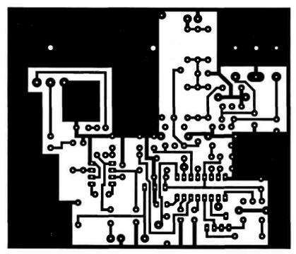
Fig. 2.2; The Chatterbox receiver p.c.b. copper track layout.
