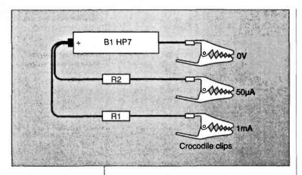
Fig. 3: A simple meter tester, capable of cheking most meters available on the surplus market.
