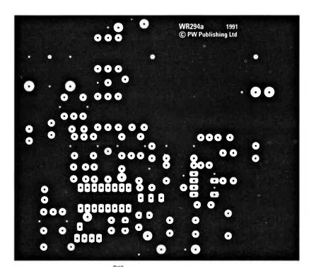
Fig. 2.3: Receiver ground plane details.
