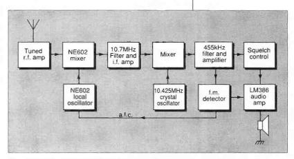
Fig. 1: Block diagram of the Ramsey 50MHz f.m. receiver kit built by Rob Mannion G3XFD.
