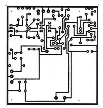
Fig.1.4: The component overlay and copper track layout of the double-sided Chatterbox p.a. and modulator p.c.b.
