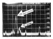
Fig. 4: Harmonic analysis. High order harmonic from an unmodulated 27MHz CB transmitter, interfering with a weak u.h.f. TV signal.
