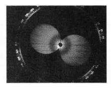
Fig. 6: Electronically generated radiation pattern of a half-wave dipole, used with the display unit shown in Fig. 5.
