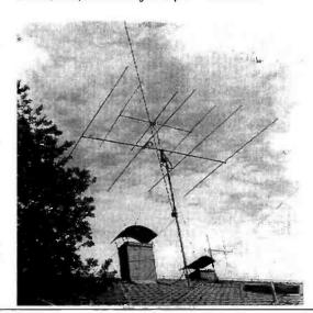
Fig. 1: Wolfgang IN3TWX's 28 and 50MHz antenna system.
