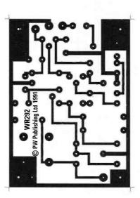
Fig. 1.3: Layout of the v.f.o. p.c.b. with component overlay (left) with the underside of the single-sided p.c.b. showing copper tracks, on the right.
