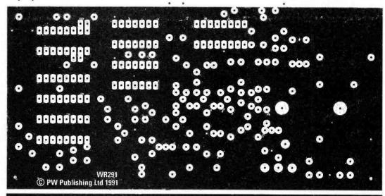
Fig. 2.2: The track pattern side of the PW Robin frequency counter. See Fig. 2.3 for the position of the links on the component side of the p.c.b.
