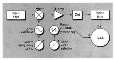
Fig. 2: Circuit block diagram of the Cushman CE15 spectrum monitor.
