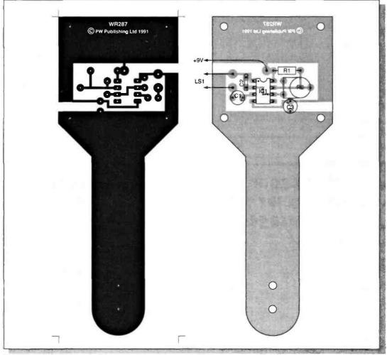
Fig. 2: The p.c.b. track details and overlay for the Morse key project.
