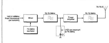
Fig.1: Block diagram of the Meon-4. In general it's almost the same as its predecessor the 'PW Meon'.
