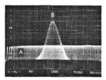
Fig. 2.9: (A) frequency response of the sweep generator (±0.1dBV). (B) transmit-to-received audio frequency response for narrow band f.m. (144MHz band).
