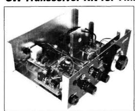
Home construction and QRP go hand-in-hand. Mike Richards G4WNC, built the recently introduced Lake Electronics DTR-7 7MHz c.w. transceiver kit. Mike's constructional efforts produced a QRP outfit that should appeal to many constructors.
