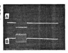
and then the actual display. Another example is the oscillogram in Fig. 2.8, which is the response of a graphic equaliser with all the controls set at maximum.
