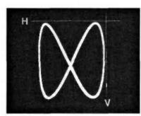
Fig. 2.1: A 2:1 Lissajous Figure. Fred explains frequency comparison using Lissajous Figures in the text.
