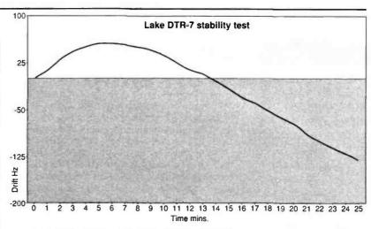
Replacing this capacitor cured the problem and resulted in the expected very good stability. To illustrate the new stability of the DTR-7, I've shown its performance in graphical form in Fig. 1.
