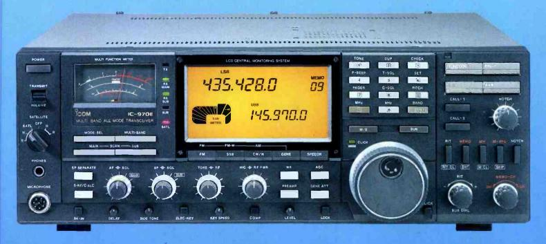
Designed for the serious operator on the 144, 430 and 1200 MHz bands, Icom's new IC-970E has up-to-date technology for DX, digital and satellite communications. The IC-970E is supplied as an all mode dual-bander for 144MHz and 430MHz bands. Optional units expand its capabilities to 1200MHz or wideband receiving from 50-905MHz.
