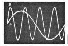
Fig. 2.3: Frequency comparison (A) Time of one cycle measured. (B) Four cycles of unknown (?) frequency (see text).
