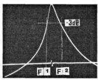
Fig. 2.10: Frequency (bandwidth) response of a 144MHz antenna to -25dBV using a v.h.f. frequency sweep technique. Usable bandwidth f1 to f2 (2MHz) is to the -3dBV points (see text).
