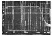
Fig. 2.7: Overall 'flat' frequency response of a high-fidelity audio amplifier using the frequency sweep technique. Marker frequency is at 1kHz. (see text for further details).
