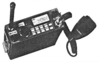
What could Yaesu engineers do to improve on the hugely popular FTX 90R series? The answer was easy, they designed and built the FTX 90R2 series. The FTX 90R2 series of transceivers provide high performance and a 2.5W output, when used with 'C' cells or nicads, ideal for serious portable operations, or when combined with matching linears, and easy to use compact multimode mobile or base station. What more could you ask from a transceiver?
