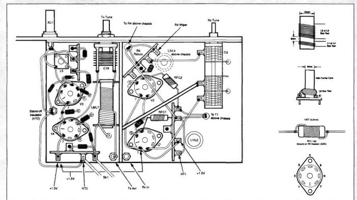
Fig. 4: The Empire wiring interconnection diagram. Note that only the most important components have been shown so as not to complicate the drawing.
