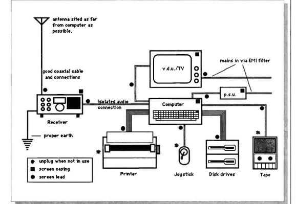
Steps for reducing hash. Do not assume that the audio and VDU cables supplied with your computer are screened - often they are not. grounded and will supply the necessary contact when in place).
