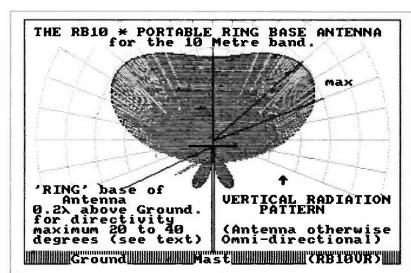
Fig. 1.2: Vertical radiation pattern of the RB10 antenna.
