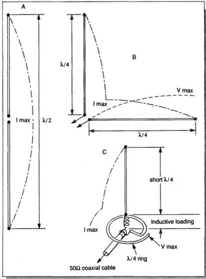
configuration resulted in a relatively efficient but smaller version for 144MHz mobile operation using an inductively loaded 'short quarter-wave' radiator. From this, the RB10 Ring Base antenna for the 28MHz band, has been developed.
