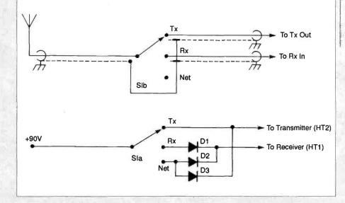
switch S1 to 'NET'. Both the oscillator and the receiver are operating but the antenna is disconnected. Tune the receiver to the strong heterodyne of the oscillator. Reduce the setting of the reaction control to ensure accurate setting at this stage.
