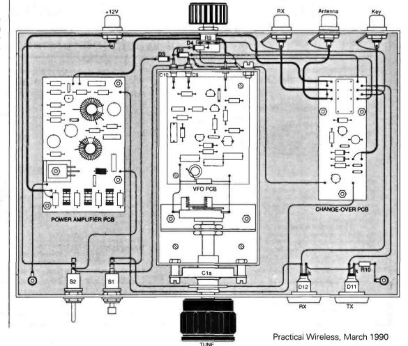
Fig. 3.1: Finished layout of the transmitter showing p.c.b. interconnections.
