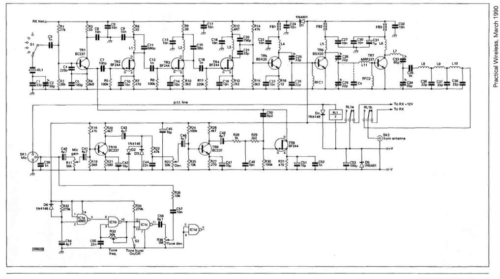
Fig. 1.2: The full circuit diagram of the PW Cub.Showing the three separate areas of the design. The top portion is the r.f. strip above the modulator stage, with the tone burst circuit based on IC1 below
