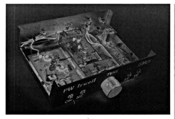
beginning with the 12V via S2, then adding +12, +TX and +RX interconnections leads. The v.f.o. cut-off control, R9, is mounted on the back panel of the outer case behind the the v.f.o.box. The signal connections starting from the v.f.o. may then be added.
