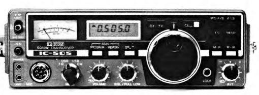
output, 3 watts or 0.5 watts on low power is available when using internal batteries. Other features include 5 memories with memory scan, program band scan, dual VFO's with split operation.
