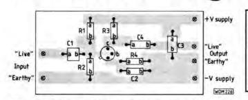
Fig. 3.7. Possible printed circuit board layout for Fig. 3.6
