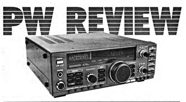
This latest addition to the Kenwood range has many features including h.f. and 50MHz amateur band coverage, and AMTOR/Packet compatibility. Mike Richards G4WNC gives the TS-680S a good airing, whilst Geoff Arnold G3GSR examines the laboratory performance.
