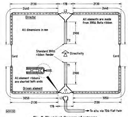
Fig. 2: Electrical diagram of antenna
