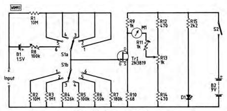
Fig. 1: The circuit diagram of the meter
