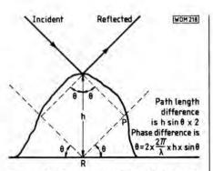
Fig. 6.5: A wave reflected from a bump suffers a phase difference of  $\theta$  compared to reflection from the level surface. The surface can be considered smooth if the total phase change is less than  $\pi/4$  radians or 45°
