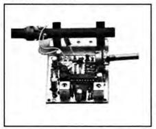
Lock into the National Physics Lab Atomic clock with the Rewbichron II and MSF receiver. The 60KHz receiver will tune to the MSF transmitter from Rugby, the data is displayed on the Rewbichron II in 12 or 24 hour format with day and date information. Bright 6 digit LED display.
