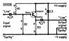
Fig. 3.9. Practical common collector amplifier
