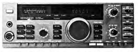
rotary control on the rear panel. When the break-in option is turned off the transmit/receive switching is achieved by either grounding the p.t.t. line or by operating the SEND/REC push button on the front panel.
