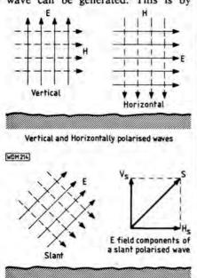
Fig. 6.1: Vertical, horizontal and slant polarised waves. The slant polarised wave has a vertical component Vs and a horizontal component Hs
