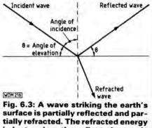
surface is partially reflected and partially refracted. The refracted energy is lost and so the reflected wave is smaller than the incident wave *Practical Wireless, May 1988*
