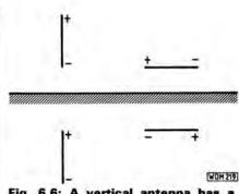
Fig. 6.6: A vertical antenna has a positive image in a good conductor and a horizontal antenna a negative image
