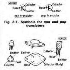
Fig. 3.2. Some different transistor shapes
