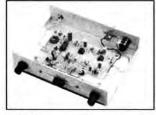
The RC14 is a simple direct-conversion receiver for the 14MHz amateur band. The design has been originated by the RSGB as an introduction to home construction. The RC14 nevertheless offers a very good specification with sensitivity of 1uV, wide dynamic range, a stable VFO and a steep-sloped audio filter.
