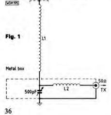
The prototype, when loaded at 3.54MHz, has a useful bandwidth of about 80kHz without having to re-tune the a.t.u. With minor adjustments to the antenna, it will go up to 3.8MHz. The a.t.u. is earthed by a 6m length of cable taken to a water pipe; but other earthing arrangements have been tried (see later) and the Eightypole does not seem to be too fussy in this respect. The bandwidth is greatly reduced without the top hat, and loading becomes more critical.
