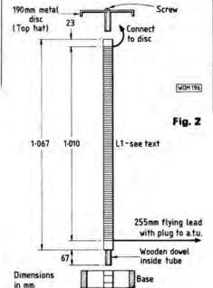
used. The centre pin, with the insulation surround removed, of a coaxial plug is soldered to the 255mm flying lead for plugging into the a.t.u. The metal shroud of the plug can be disposed of.
