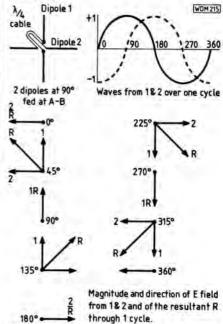
Fig. 6.2: Generation of a circularly polarised wave by a pair of crossed dipoles. The resultant wave rotates through 360° clockwise every cycle
