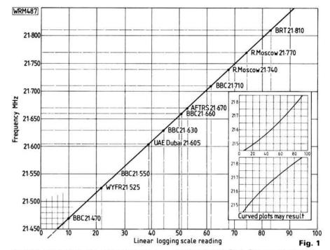
squares, enter along the horizontal axis a scale incorporating 50 such squares to provide effectively a linear scale 0 to 100, corresponding to the new receiver logging scale. If a receiver with only one s.w. band is being calibrated, mark in along the vertical axis of the graph 1MHz steps at each line forming every other square. If the receiver has bandspread scales, prepare a separate sheet for each band and mark the vertical axis in steps of 100kHz or 50kHz at every fifth square.
