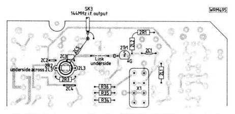
Fig. 2: Revised component location. 2L3 is tapped at 2 turns from the top
