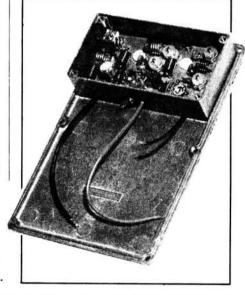
The lid-mounted Spectrum Communications 50MHz p.a.
