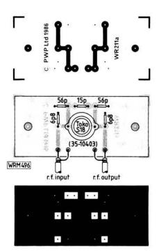
Fig. 9: Component layout and p.c.b. track layout of the filter board
