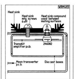
Fig. 4: Heatsink and p.a. mounting details
