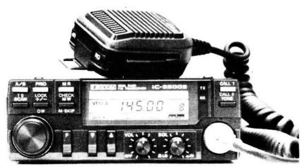
A new exciting set is the ICOM IC-3200E FM Dual-band transceiver (144-430/440 MHz). The IC-3200E delivers 25 Watts of output power on both bands.
