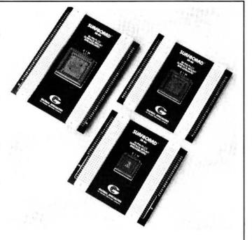
JEDEC "type A" p.l.c.c. polarised for easy registration. Stand-offs are provided for heat dissipation.
