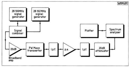
Fig. 7: Arrangement used for i.m.d. measurements
