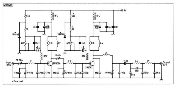
Fig. 3: Circuit diagram of the Spectrum TA6U2 p.a.
