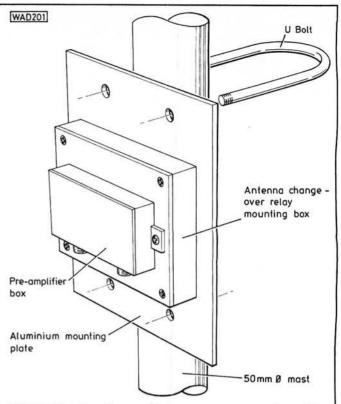
Fig. 5: Masthead mounting arrangements adopted by the author. For increased isolation on TX the antenna C/O relay RLC is fitted inside a separate weatherproof enclosure
