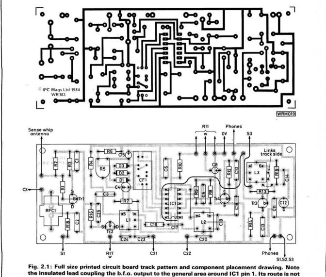
the insulated lead coupling the b.f.o. output to the general area around IC1 pin 1. Its route is critical but care must be taken to ensure that it does not short to any other component
