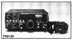
ability to tune whilst transmitting, 25 watts output, 6 memories and of course memory scan: TRIO's two metre multimode, the TR9130.
