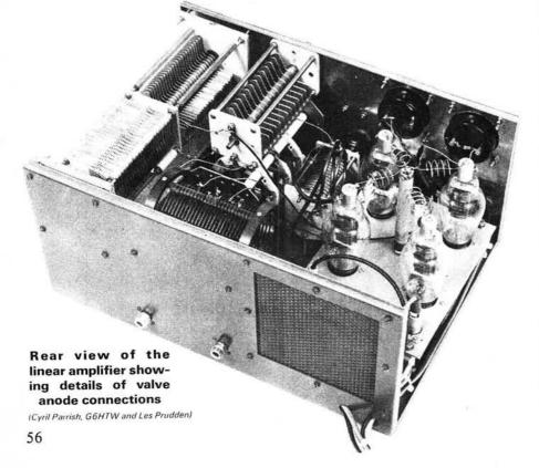
and adjusting the trimmer capacitor (Cin) for 1:1 v.s.w.r.
