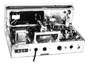
collector of Q5 are labelled e, b, c on the lower side of the board, which helps in locating the solder points of C16. Using a small size soldering iron and a desoldering aid such as solder braid or a suction device, remove C16. The hole spacing on the board corresponds to the pin spacing of the resonator so the latter pushes in easily in place of C16. Solder below the board, check T16, T17 and T18 and try out the set.
