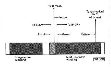
Fig. 2: Ferrite rod antenna, viewed from rear
