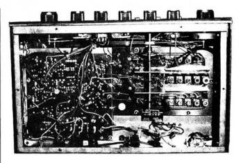
pin 6, the black one from BLK goes to pin 3 and the remaining yellow wire coming from B-YELL is soldered to pin 4. The new r.f. transformer is soldered to a small bracket which is attached to the rear of the main tuning capacitor using the small screw that holds on a wiring clip. The four short ends of the wires left on the medium wave winding on the ferrite rod are tied onto the rod so that they are available in the future.
