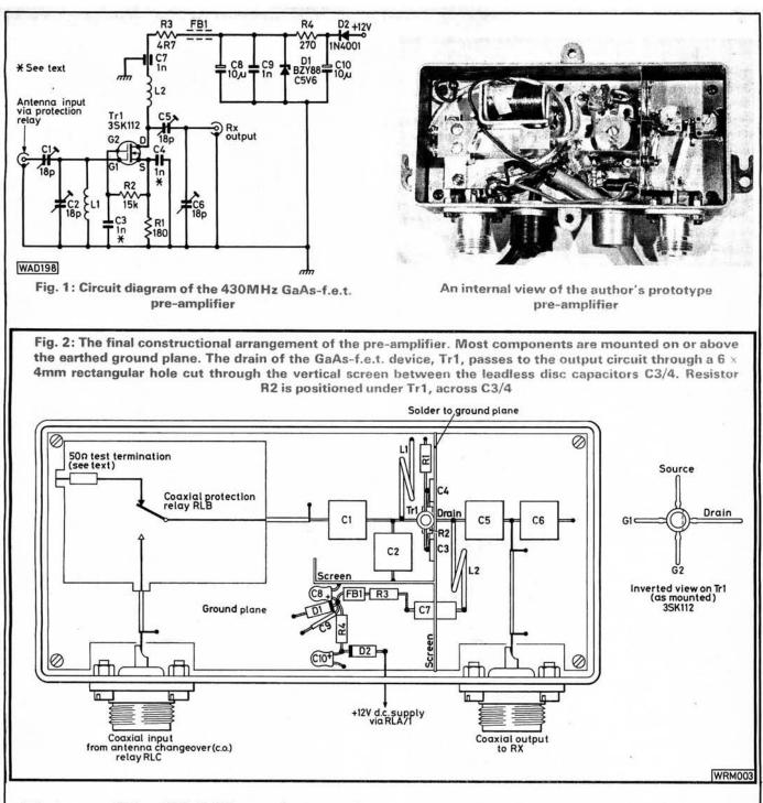
within the range 220 to 1000pF. Of greater importance is their size, which means using slightly higher voltage components. Leadless disc capacitors are notorious for exploding when heated during soldering. The use of higher voltage devices will lessen the likelihood of this happening.
