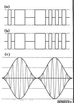
Fig. 1: (a) Typical c.w. or Morse code characters where the power output is either maximum or zero. The sharp rise time would create a series of undesirable harmonics which are suppressed in the transmitter to produce a rounded waveform as in (b). In (c) a sinewave modulates the carrier to give twice the amplitude of the c.w. carrier
