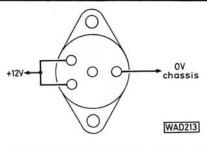
Fig. 4: Power socket connections
