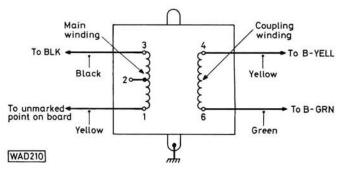
Fig. 3: Medium wave r.f. transformer connections
