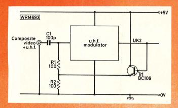
The video signal is fed from the p.c.b. into the modulator by a short length of tinned copper wire, entering the modulator through one of the holes in the plastics grommet. This wire must be carefully unsoldered from the plated-through hole in the p.c.b., making sure that the pad is not lifted, and bent so that it is horizontal and in line with the grommet hole.
