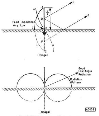
Fig. 84: The 1 wave vertical antenna
