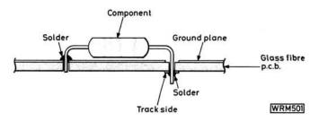
Fig. 9: The correct method of mounting components on the p.c.b.
