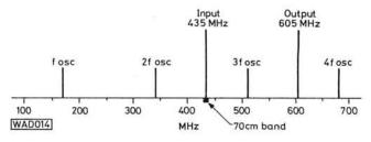
Fig. 3: Frequency spectrum showing oscillator and signal frequencies
