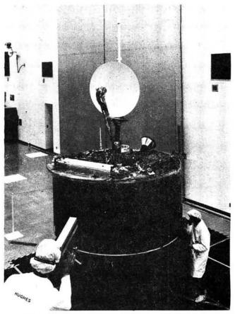
The *Pioneer* Venus Orbiter probe. Data is returned to earth via the parabolic dish
