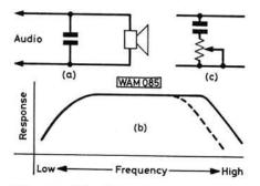
Fig. 1: (a) Capacitor connected across audio circuit to reduce response at high frequencies. (b) Response curve of audio amplifier is shown in solid line, modified to the dotted line when the capacitor is added. (c) Commonly used tone control circuit
