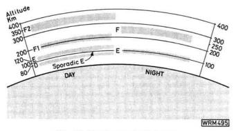
Fig. 81: The ionospheric layers
