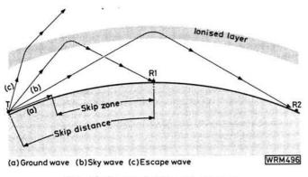
Fig. 82: Ionospheric propagation
