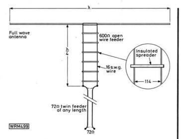
Fig. 91: A  $\frac{1}{4}$  wave transformer
