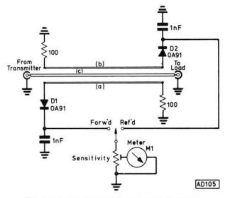
Fig. 88: A simple standing wave ratio meter
