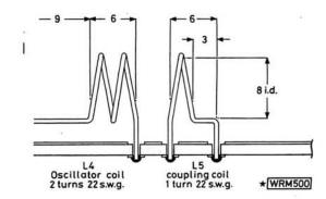
Fig. 8: Details of the wound components, L4 and L5, and their mounting
