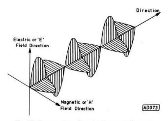
Fig. 80: Propagation of an electromagnetic wave
