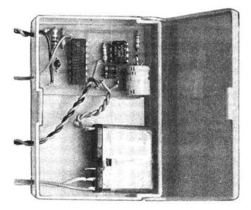
The photograph above shows the author's prototype unit housed in a small plastics box.
