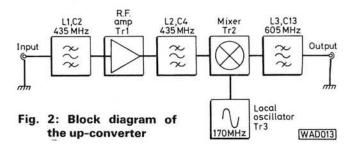
The converter uses a double-sided p.c.b. with "stripline" tuned circuits and matching flat T pack transistors.
