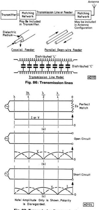
Fig. 87: Transmission line terminations
