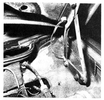
Fig. 1: Additional bonnet bonding strap fitted to an Austin Maxi
