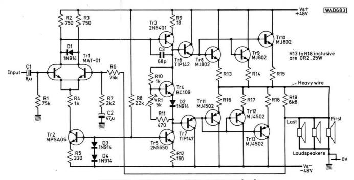
Fig. 19: An amplifier for very high output power levels
