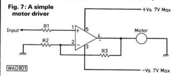
the amplifier are at the same potential; that is, when the input is at ground potential. As the input is made positive with respect to ground the motor will rotate in one direction, but when the input is made negative, the motor will rotate in the other direction. Resistors R2 and R3 set the gain and therefore the sensitivity of the circuit.
