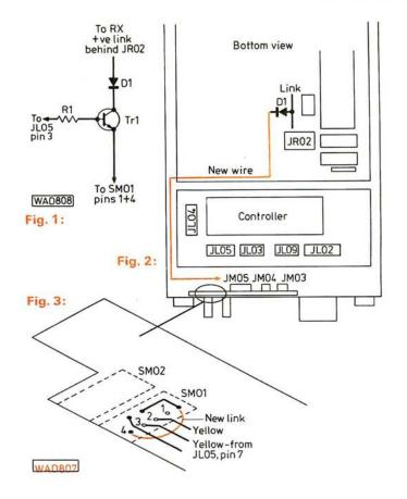
wire coming from pin 7 of JL05 to pin 3 of SM01, and then solder the remaining piece of yellow wire to pin 2 of SM01. Solder the emitter of Tr1 to SM01 at either pin 1, pin 4 or to the linking wire.
