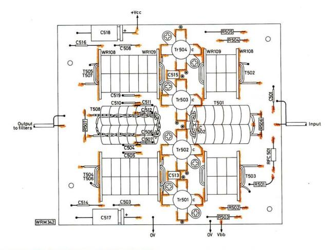
As readers will no doubt have realised, the printed circuit track pattern in Fig. 23: Component placement drawing (page 43 last month), was printed upside down. We therefore repeat it here, with apologies
