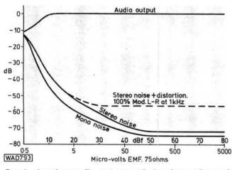
Graph showing audio output and signal-to-noise and signal-to-noise-plus-distortion on stereo for various input signal levels on 98MHz
