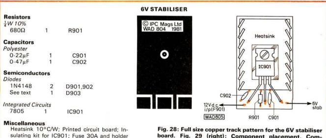
board. Fig. 29 (right): Component placement. Components are soldered directly to the copper
