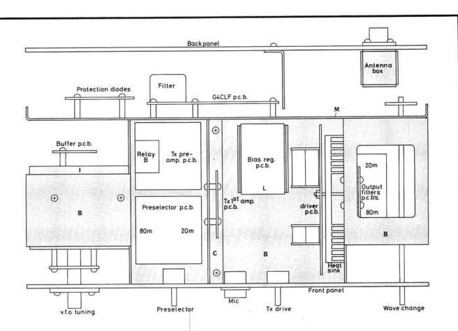
Fig. 34 (above): Underside view of the *PW* Helford case showing how the various screens and p.c.b.s mount. Fig. 35 (below): Top view of the case
