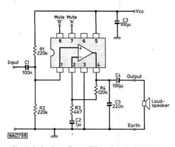
Fig. 4: A simple audio amplifier using the SL6310C
