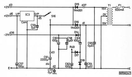
Fig. 1 (top): Circuit diagram of f.m. and TV sections of the *PW* Winton Tuner Fig. 2 (left): Circuit diagram of a.m. section Fig. 3 (above): Circuit diagram for *PW* Winton power supply
