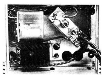
The photograph above shows the 6V stabiliser, relay A and the protection diodes D903
