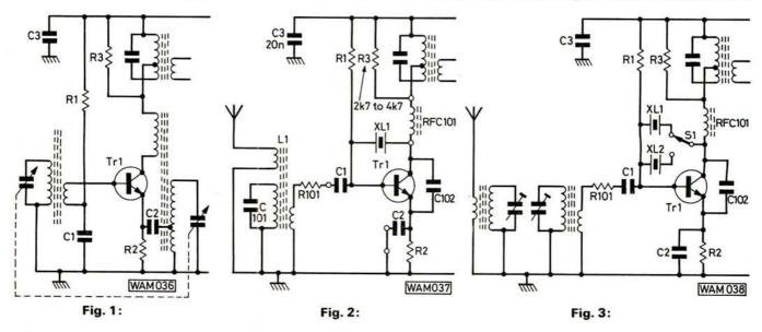
separate board and then fixing it to the receiver circuit board, so an unusual mixer/oscillator combination was tried and the original circuit was modified as shown in Fig. 2. This was found to be quite satisfactory since a minimum of extra components was required and even the original mixer/oscillator transistor was used.
