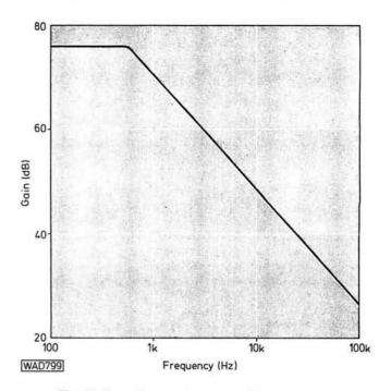
Fig. 5: Open-loop gain versus frequency
