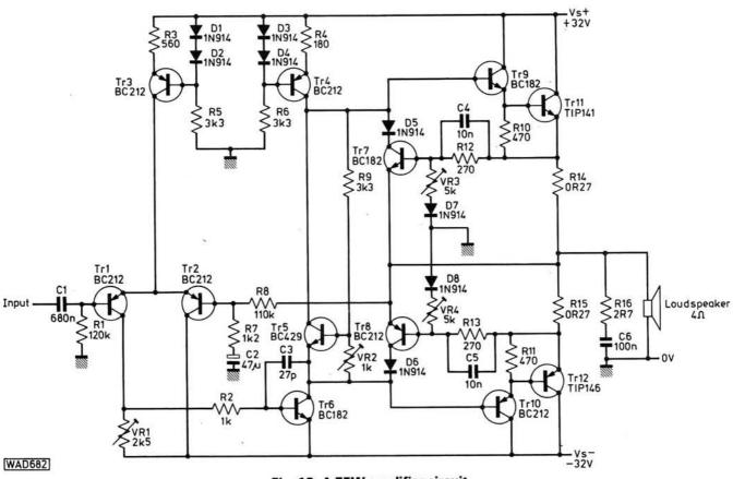
Fig. 18: A 75W amplifier circuit
