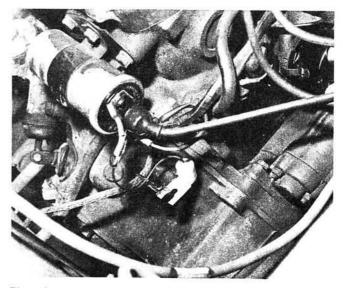
Fig. 2: Temporary quick-fit capacitor connected between the h.t. coil + terminal and earth
