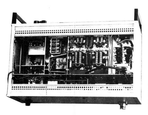
View of the top of the *PW* Helford with the lid removed. The p.a. is central with the preselector capacitor and the v.f.o. to its left. The speaker is mounted on the lid with its magnet fitting into the space above the v.f.o. capacitor
