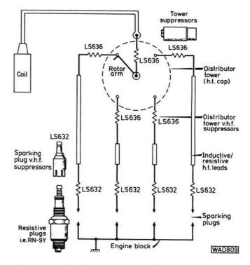
Fig. 4: Block diagram of a fully suppressed h.t. distribution system
