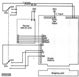
Fig. 4: Connections of the d.f.m. board and display showing the switching arrangements and power supply connections used in the prototype unit. Other arrangements are possible to allow the d.f.m. to be used for other purposes and these are detailed in the comprehensive instruction booklet supplied with the d.f.m. module
