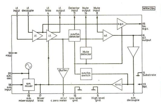
Fig. 15: Block diagram of the ULN2242A/TDA1090 integrated circuit
