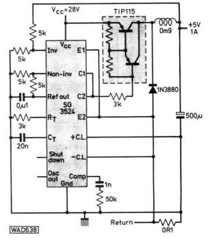
Fig. 4: This circuit uses an external TIP115 Darlington to boost the maximum ouput current to 1A
