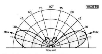
Fig. 2: Approximate vertical radiation pattern when the centre point of the radiating section is ½2 above ground of good conductivity, and the aerial is situated in very clear surroundings
