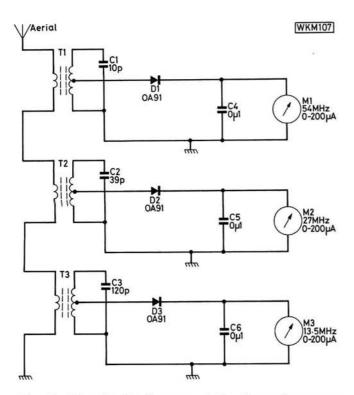
Fig. 1: The circuit diagram of the three frequency wavemeter
