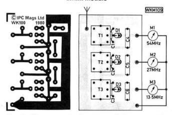
Fig. 5: The copper track pattern of the wavemeter p.c.b. shown here full size. Fig. 6 (above right): The component placement drawing of the wavemeter p.c.b. Ambit International will be able to supply ready built and aligned boards for those constructors without the necessary gear
