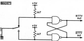
Fig. 23: The simplest method of converting 80 volt signals down to TTL levels, but not the safest. Consider, for instance, the result of the  $470\Omega$  resistor going open-circuit
