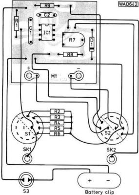
Fig. 3: The p.c.b. copper track pattern is shown full size at the top. The component placement is indicated, together with the other wiring above
