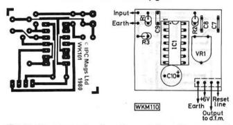
Fig. 7: The copper track pattern of the add-on period measuring unit shown here full size. Fig. 8 (above right): The component placement drawing for the add-on unit. This board plugs directly onto the main d.f.m. board as shown in Fig. 4
