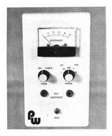
forward biased silicon diode D1. R7, R8 and M1 comprise the voltmeter circuit which has a sensitivity of about 6 volts f.s.d. (i.e., ten times the reference voltage). The voltmeter sensitivity can be varied to some extent by adjustment of R7 for calibration purposes. R2 to R6 are the equivalent of Ra in Fig. 1(b), and one of these is selected by S1. This provides the unit with five measuring ranges of  $0-1k\Omega$ ,  $0-10k\Omega$ ,  $1-100k\Omega$ ,  $0-1M\Omega$ , and  $0-10M\Omega$ .
