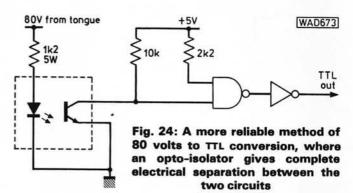
to isolate the 80V supply completely from the TTL circuitry by means of an opto-isolator as shown in Fig. 24.
