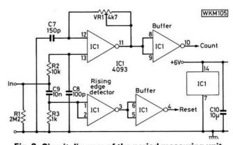
Fig. 3: Circuit diagram of the period measuring unit
