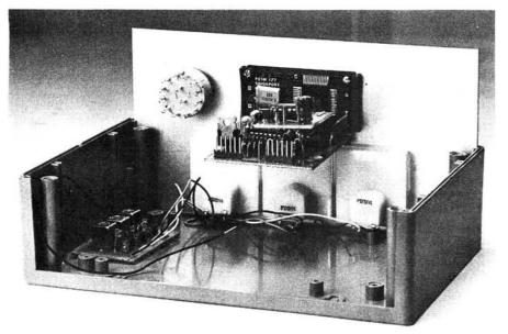
Internal view of the test set before final wiring. Note that the d.f.m. main p.c.b. has yet to have its extra support pillar fitted. This will be fitted between the bottom of the Verobox and the hole drilled in the rear corner of the p.c.b. and will consist of a suitable length pillar
