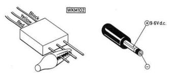
Fig. 2 (left): Identifying leads to be shorted Fig. 3 (right): Polarity of the external power connector
