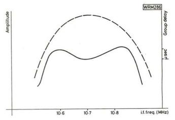
The crucial feature of any f.m. filter is the group delay (see Fig. 17)—which is related to the phase linearity by: Group Delay = Phase change/frequency change. The ideal phase change from one side of the filter to the other is a straight line. This is the same as the slope of the f.m. detector, which uses exactly the same principle when demodulating f.m. signals in a quadrature system, to convert frequency change into amplitude change.
