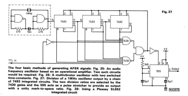
Generating AFSK tones by division of a crystalcontrolled oscillator is a useful method, particularly if an accurate source of, say, 1MHz is already available from a counter, MPU or other test oscillator.
