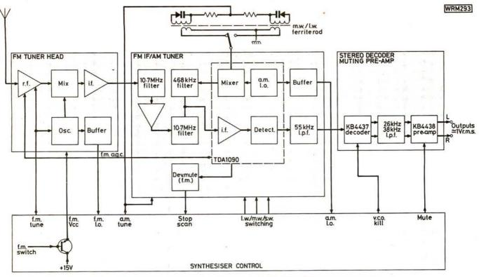
Fig. 11: Simplified block diagram of the complete tuner system
