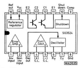
Fig. 1: The connections to the SG3524 device
