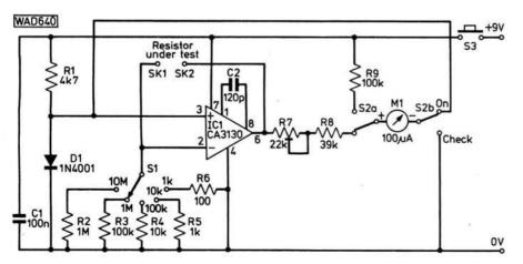
Fig. 2: The complete circuit diagram of the resistance meter
