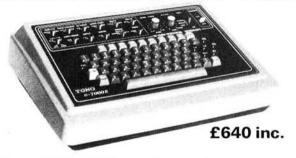
The new THETA 7000E means that every Amateur can enjoy the visual display of CW, RTTY, and ASC11 in both transmit and receive modes. Just connect the TONO to any TV set via the antenna terminals or to a page printer from the parallel port provided. Bring up your CW speed in receiving or sending by either watching receiver sent or from recorded cassettes. Connection to the transceiver is via the key, phone and mic sockets.
