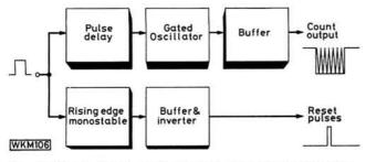
Fig. 2: Block diagram of the add-on period measuring
