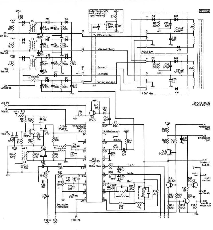
Fig. 14: Circuit diagram of the f.m. i.f./a.m. tuner module, with associated remote tuned and switched ferrite rod aerial
