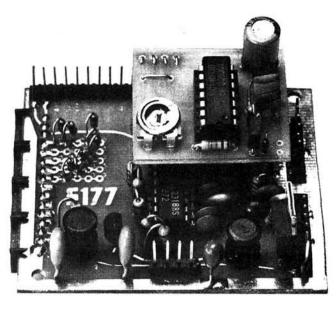
The main d.f.m. board with the add-on unit in position.
