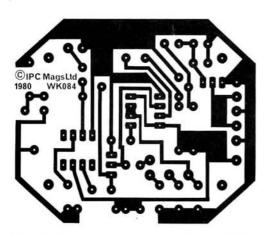
Fig. 2: Copper track pattern shown full size
