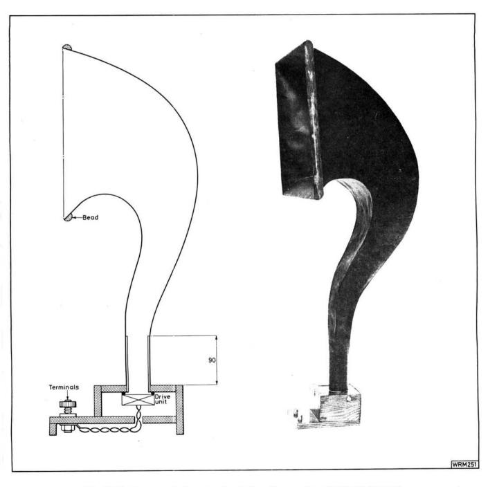
Fig. 7: The home-made horn speaker built up from papier maché and plywood
