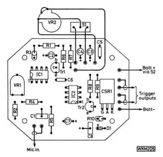
Fig. 3: Component overlay on the p.c.b. CSR1 is fitted with its normal mounting surface facing away from the board
