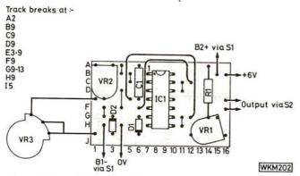
Fig. 2: The layout of the components on a piece of Veroboard. A socket should be used for the c.m.o.s. integrated circuit
