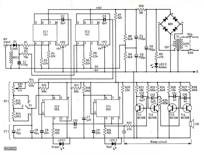
Fig. 5: The complete circuit diagram of the r.f. activated repeater timer
