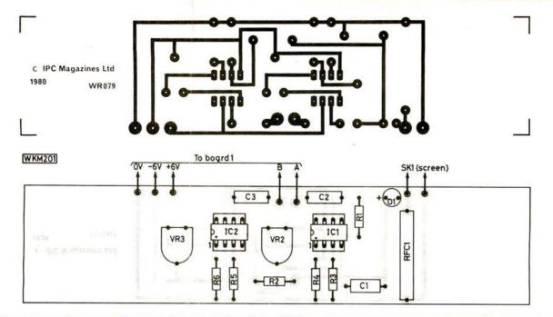
Fig. 7: The copper track pattern (top) of the r.f. input board shown full size with the component placement drawing below it
