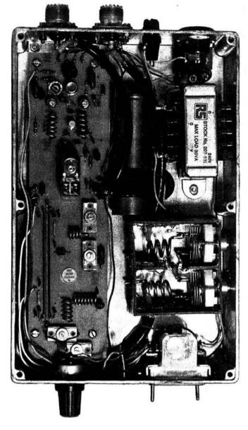
from the amplifier module to provide power for the "Nimbus" or any other transceiver used as the exciter. This makes a considerable saving on the internal battery consumption of the "Nimbus" when it is operated in conjunction with the amplifier module.
