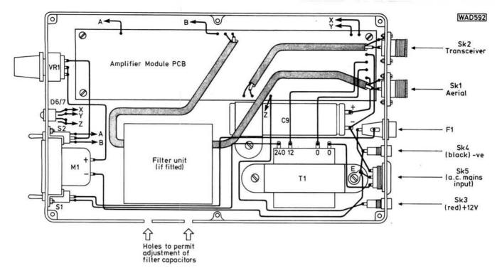
Fig. 5: Interconnecting wiring and internal layout of the complete p.a. module also showing the position of the filter unit
