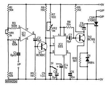
Fig. 1: Circuit diagram of the Acoustic Flash Trigger Unit. The outputs each go in screened lead (as shown in Fig. 3) to the flash-gun/camera connectors. Note that C8 should be shown as  $0\mu 22$ , and is non-polarised
