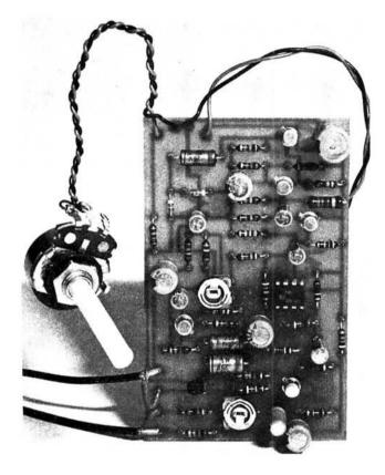
Any audio limiter is, in essence, an electronic device which accepts an a.f. signal at its input and ensures that the voltage of the same signal at the output does not exceed a previously selected value. Well-designed and working correctly it should have no other effect whatsoever.
