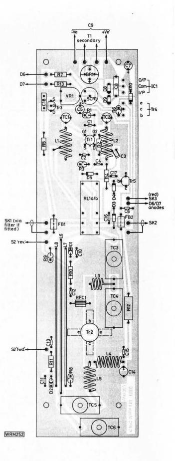
Fig. 3: Copper track layout of the amplifier p.c.b. module shown full size
