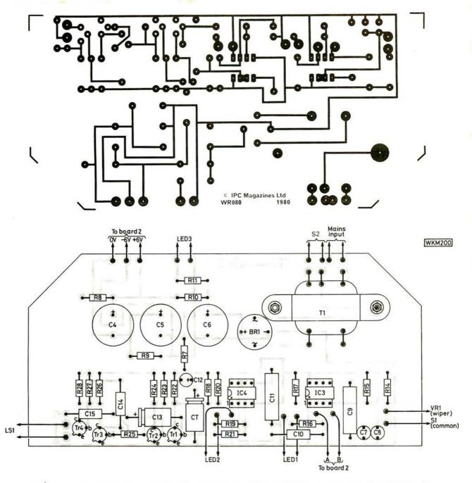
Fig. 6: The copper track pattern (top) is shown here full size with the components layout below it
