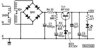
Fig. 8: Circuit for a 30V stabilised power supply
