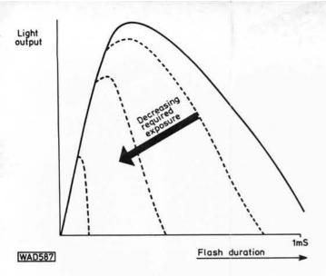
Fig. 4: Effect of thyristor circuit on the duration of the flash
