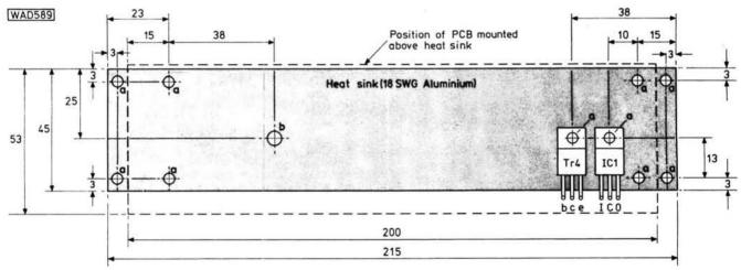
Notes: All dimensions given in mm. Holes marked 'a' are M2.5 or 6BA clearance, hole marked 'b' is 4mm diameter
