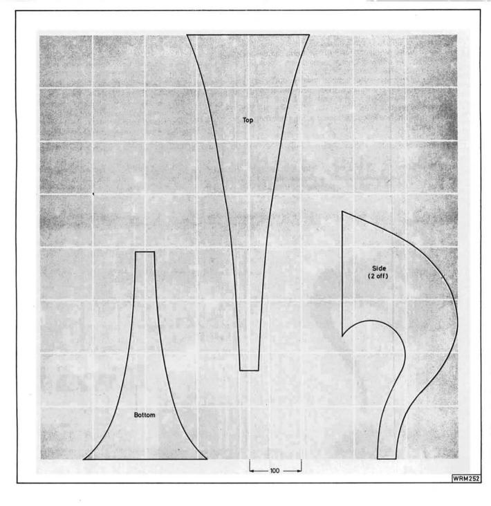
Fig. 8: (Above) the patterns for constructing the horn. The patterns should be scaled up using squared paper, each square being 100mm  $\times$  100mm
