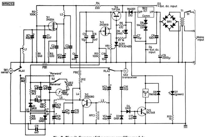
Fig. 2: Circuit diagram of the power amplifier module
