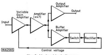
Fig. 2: Limiter block diagram
