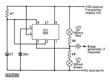
Fig. 1: The basic timer circuit using a 555 timer integrated circuit
