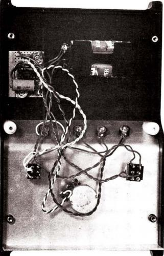
The servo tester was built into a plastics box with a metal front panel. The size and shape of the box is not important and if the constructor felt so inclined the tester can be incorporated with the battery charger described last month
