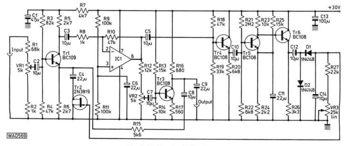
Fig. 4: Limiter circuit diagram
