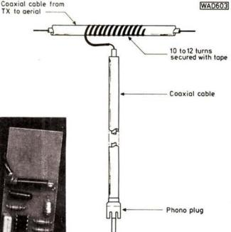
Fig. 8: The construction of the r.f. pick-up. The ten or twelve turns of wire are wound round the coaxial cable from the transmitter to the aerial
