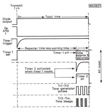
Fig. 4: The timing sequences used in Fig. 5
