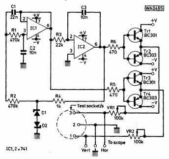
Fig. 2: Circuit diagram of the semiconductor tester.
