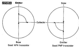
Fig. 3: The displays for good transistors showing the portions of the display representing the base, emitter and collector connections
