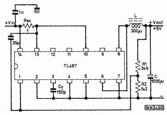
Fig. 3: A typical step-down TL497 circuit providing a +5V output
