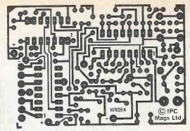
Fig. 9: The copper track pattern for the printed circuit board used for the complete receiver and decoder is shown full size on the right. The laminate should be  $\frac{1}{32}$  inch thick and the p.c.b. is carefully trimmed to fit snugly in the plastics case. The component placement for the p.c.b. is shown above. It should be noted that all components must be as small as possible and fitted flush with the board surface with the exception of the two jacks for the crystal
