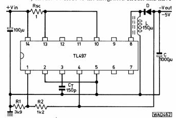
Fig. 5: An inverting switching regulator circuit providing an output of about —5V
