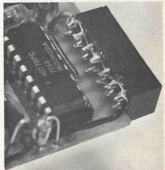
Close-up view of the SLM socket block showing the method of mounting and wiring to the p.c.b. The two rows of pins above the board are wired using 22s.w.g. tinned copper wire which also serves to complete the power rails on the p.c.b.
