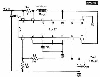
Fig. 4: A step-up circuit providing an output of +16.2V with the component values shown
