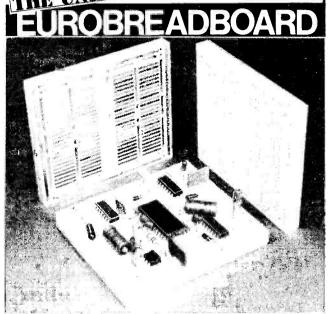
Logically laid out to accept both 0.3" and 0.6" pitch DIL packages as well as Capacitors, Resistors, LED's, Transistors and components with leads up to 85mm dia
