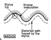
Fig. 12: Illustration of tracing distortion
