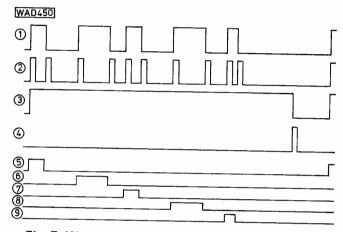
Fig. 7: Waveforms at various points in the decoder
