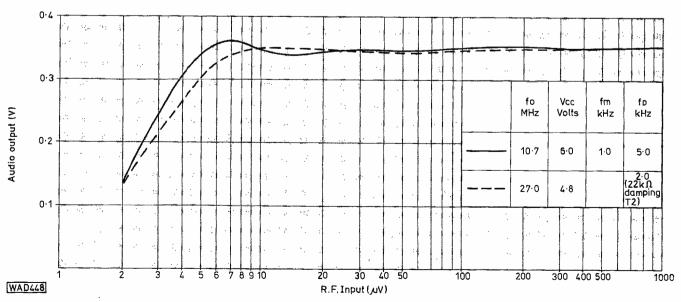
Fig. 4: The response curves for the r.f. input stage of the receiver
