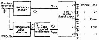
Fig. 6: Block diagram of the decoder
