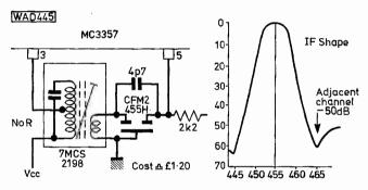
Fig. 5: Two different filter design approaches for the receiver. The filter chosen for the FM-80 system is the Murata CFW455HT
