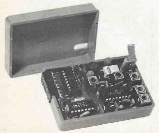
The finished p.c.b. mounted into the SLM case. This picture also shows the two cut-outs to be made in the case halves
