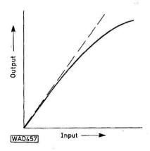
Fig.15: Transfer characteristic of amplifier. Ideal state shown by the broken-line (perfectly linear), and realistic state (exaggerated) shown by the full-line curve
