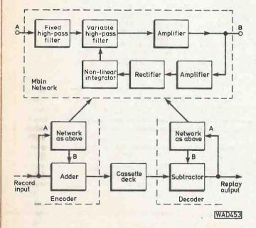
Fig. 11: Block diagram of Dolby B noise reduction encoding and decoding
