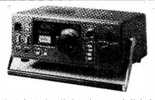
For the first time in a mid price receiver, a true noise blanker is provided to remove pulse type ignition noise.
