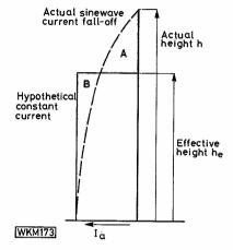
Fig. 6: Relationship of Actual Height and Effective Height of a  $\lambda/4$  vertical aerial. Areas ''A'' and B'' are equal
