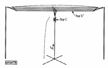
Fig. 9: A "T" aerial with multiple top span giving added capacitance loading, and top loading inductance
