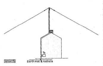
Fig. 12: If space does not permit a mast in the garden, the aerial of Fig. 11 may be mounted on the house-top
