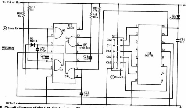
Fig. 8: Circuit diagram of the FM-80 decoder. The output socket is shown wired in a suitable manner for the majority of servos available but if servos of a different design to those to be described later are used then the socket connections must be checked
