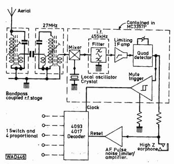
Fig. 2: The design approach chosen for the PW FM-80 f.m. receiver
