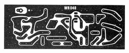
Fig. 2: Layout of the p.c.b. (shown full-size)
