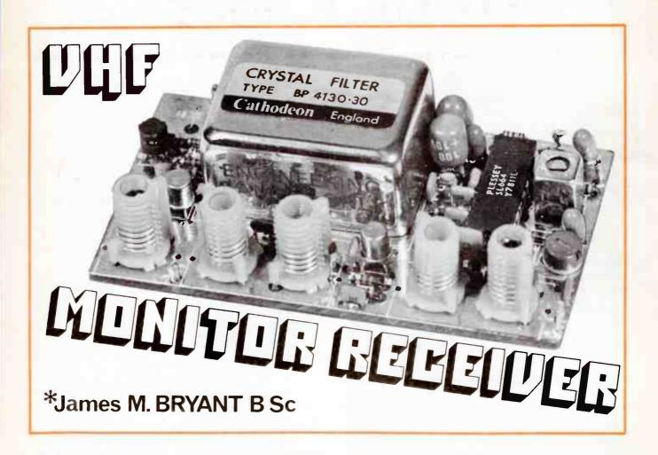
The circuit diagram of the complete receiver is given in Fig. 1. It can be seen to consist of a double-tuned input arrangement feeding a dual-gate m.o.s.f.e.t. amplifier with a gain of 18dB. Another double-tuned circuit couples the amplifier to a second dual-gate m.o.s.f.e.t. which acts as a
