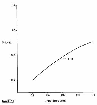
Fig. 5: Relationship between total harmonic distortion and input signal level
