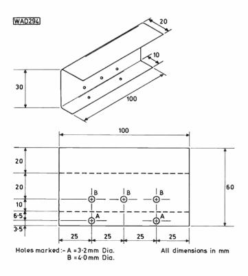
Fig. 5: Construction of the tinplate screen
