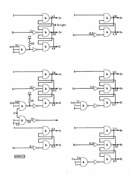
Fig. 2(b): The display gating for squares 2, 4, 6 and 8 are shown in this drawing. These gates ensure that the correct symbol is displayed in the appropriate square
