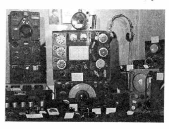
Fig. 5: Now museum pieces, the R1155/T1154 stands proudly in the centre with three sets from the Heinkel 111 on the left and a piece of wartime RADAR on the right
