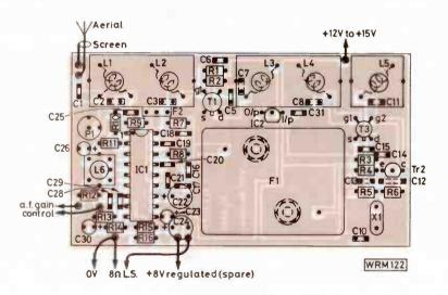
Feed a 10.7MHz frequency-modulated signal to the input side of the crystal filter. Now, with full audio gain and minimum setting of the squelch resistor, tune the quadrature coil for minimum distortion at the output. If clipping occurs, back off the audio gain slightly.
