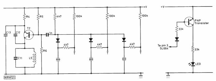
Fig. 2 (left): Adding multi-channel facilities. Grounding one terminal "T" activates the associated crystal
