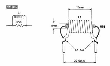
Fig. 6: Winding details of the two coils L1. Internal diameter 8mm; Length 15mm; 3 layers of 10 turns each (Total 30 turns) 18 s.w.g. enamel copper wire. R58 is  $10\Omega$  1W carbon resistor
