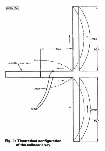
Two folded half-wave elements driven in phase from a quarter-wave stub constitute the active parts of the device, originally built for use on the Norwich 70cm repeater. The requirement called for a pair of aerials with at least 3dB gain which could be mounted on a mast without undue effect on their omni-directional properties—i.e. with minimal distortion of the otherwise circular radiation pattern.
