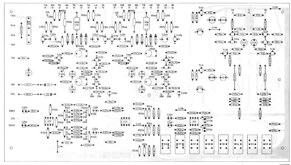
Fig. 7: Component layout for the PW Winton amplifier. This is shown slightly reduced in size
