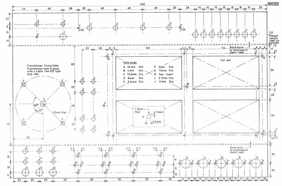
Fig. 14: Marking out details for the aluminium chassis which is made from 1-2mm thick sheet
