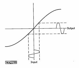
Fig. 2: Transfer characteristic of magnetic tape showing non-linearity of odd-order terms, which is responsible for odd-order distortion on the output signal. The curve takes account of the correction provided by the h.f. bias
