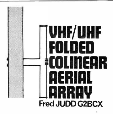
This aerial is a two-element colinear design for vertically polarised (omni-directional) radiation. It may be constructed for use on either the 2m or 70cm amateur bands and is a development of the very successful "Slim Jim", published in April 1978.
