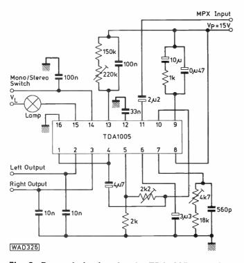
Fig. 8: External circuitry for the TDA1005 operating in the time multiplex mode
