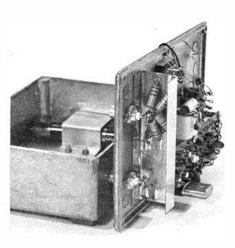
Internal view of the unit, showing arrangement of dummy load resistors
