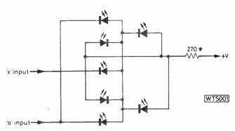
Fig. 4: Circuit diagram of one l.e.d. display. This forms the display for one square and nine of these are required for the complete game. The 270 $\Omega$  resistor is the approximate value needed to limit total current to 10mA
