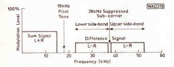
Fig. 1: Spectrum of the stereo multiplexed signal
