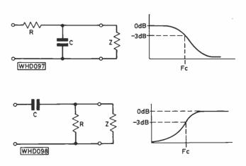
Fig. 1: Basic filter circuits and their response curves: (a) (Top) Low-pass. (b) (Bottom) High-pass
