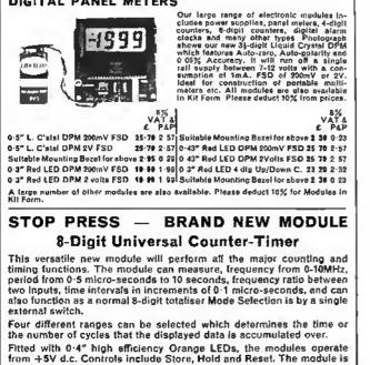
from +5V d.c. Controls include Store, Hold and Reset. The module is fitted with a 10MHz Quartz Crystal to give a highly accurate timebase, with a temperature stability of  $\pm$ 10ppm over the temp. range -20 C to +70°C.
