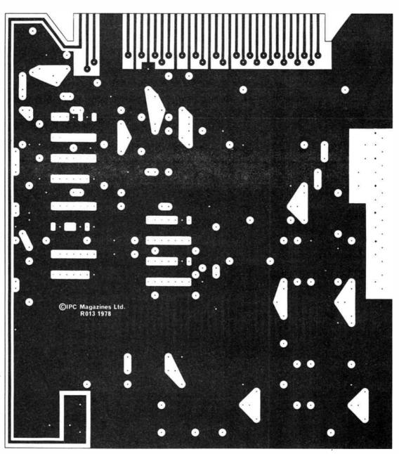
Fig. 3: The copper ground plane pattern of board 4
