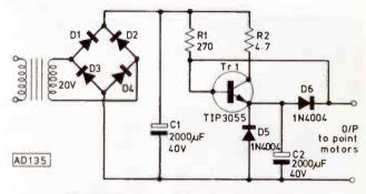
Fig. 1 The complete circuit diagram
