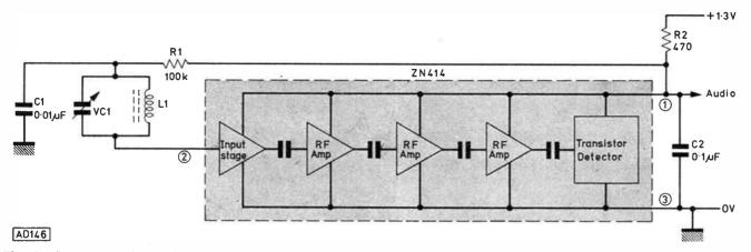
Fig. 2: A basic t.r.f. receiver circuit using the ZN414
