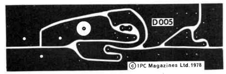
Fig. 3: PCB viewed from the copper side. This board is available from the PW Readers PCB Service
