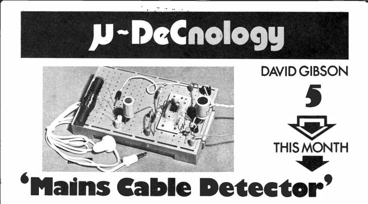
This month's circuit uses the 741 op. amp. in a closed loop inverting mode to form a sensitive mains cable detector. A simple but very useful device it can save certain disaster when deciding where to bang nails, etc., into walls.
