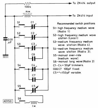
Fig. 11: A six position switching circuit
