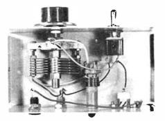
Fig. 3: A photograph of the practical layout, which is simple enough to construct from the theoretical circuit details
