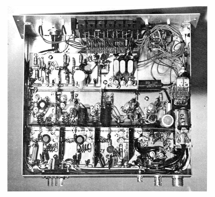
An inside view of the 'Avon Transmitter'. Note, that while six are specified, the prototype used only 3 channels in the crystal oscillator on Board 1
