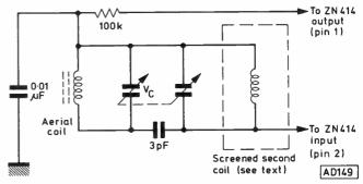
Fig. 10: A double tuned circuit for greater selectivity
