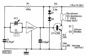
Fig. 5: Adding a single transistor amplifier stage
