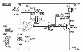
Fig. 1: Circuit diagram of the cable detector
