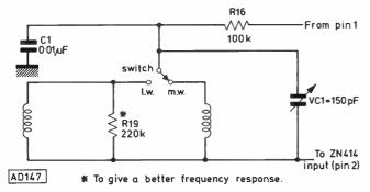
Fig. 9: Switching circuit for I.w. and m.w. coils
