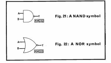
As we might expect, the symbol for a NOR gate is like that for OR but with a circle on the output line to show that the output is inverted. This is shown in Fig. 22. We can write down the action of a NOR gate as
