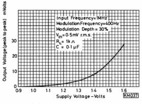
Fig. 3: Gain characteristics of the ZN414
