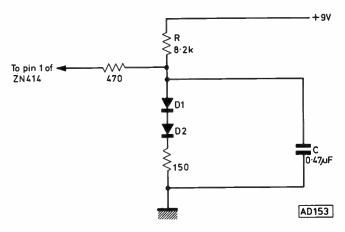
Fig. 6(a): An alternative voltage stabiliser using two silicon diodes
