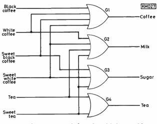
Fig. 16: Logic circuit for a hot drinks machine
