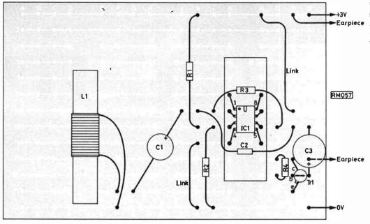
Fig. 2: Layout of the mains cable detector on a µDeC. The same layout can be used to build the circuit permanently on a matching Blob Board
