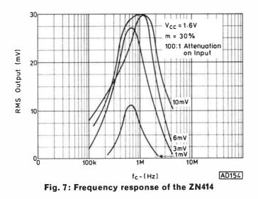
It can be seen from Fig. 7 that there is a considerable difference in the output voltage as the input rises from 1mV up to 3mV, but any further increase in the input voltage produces a relatively small change in the audio output level owing to the a.g.c. action.
