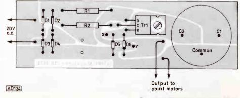
Fig. 2: The component layout. (Note; The two unmarked holes are for alternatively mounting C1 remote from the p.c.b.)
