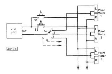
Fig. 4 Circuit diagram showing switching arrangement for operating more than one point motor
