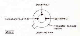
Fig. 1: Pin connections of the ZN414
