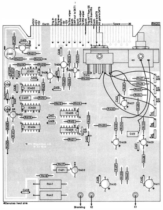
Fig. 2: Component layout of board 4. Note that the components are mounted on the copper ground plane side of the board
