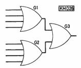
Fig. 15: Cascading OR gates to provide more inputs
