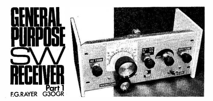
A frequency coverage of approximately 1.7MHz to 15MHz includes many useful bands and is obtained in this receiver by two switch-selected ranges. The tuned circuits comprise the four coils shown in Fig. 1, and a few points should be noted.
