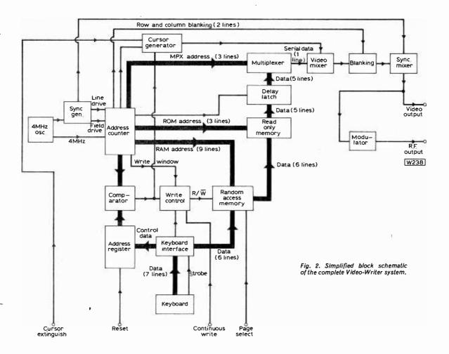
ponds to the ADDRESS for column 31. Fig. 3. The five wires that carry the 32 codes are fed to the Random Access Memory (RAM) and tell it to give out the codes for the characters that occur in that column. There will, of course, be 16 possible codes depending on which line of text (Row) we are considering and this is where the idea of matrixing comes in.
