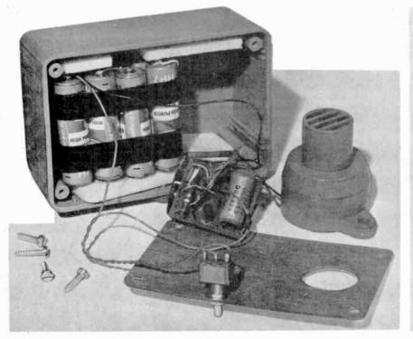
Fig. 3: above, is a full size template of the five pleces of SRBP required for the sensor head. Holes are drilled as indicated to accommodate the wiring. The photograph, left, shows the individual parts of the Alarm before being assembled in the box.
