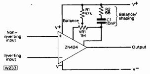
Fig. 2: The basic circuit utilising the ZN424 gated amplifier.
