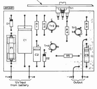
Fig. 2: Actual size printed circuit board showing foil side above and component overlay below.
