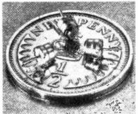
Lemo (UK) are now marketing what must surely rank among the smallest variable resistors ever made: the Siegert Type VW 00. The cylindrical body of this p.c.b. or hybrid-circuit resistor measures only 2:45mm high by 2:6mm diameter. It is of dusttight design, and as it has a stainlesssteel body it has good corrosion resistance: for example it resists perspiration.
