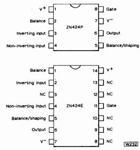
Fig. 1: The pin connections for the two types of ZN424 package likely to be encountered.
