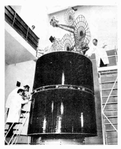
An Intelsat IVA satellite during pre-flight testing. Note the great area of solar cells and the reflectors at the top for the various aerials. (Courtesy : Intelsat Washington).
