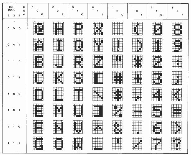
Fig. 4. Character Fount and the ASCII coding used to designate each character.
