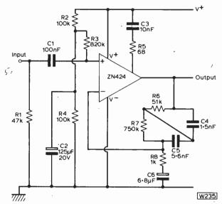
Fig. 4: This circuit shows the ZN424 as a pre-amplifier for use with a magnetic cartridge.
