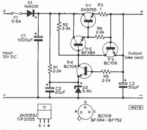
Fig. 1: Complete circuit diagram of the unit, which is basically a series-pass voltage regulator. The output in this case is 6V, although 7.5V and 9V are obtainable by the alteration of D2, R1 and R2.
