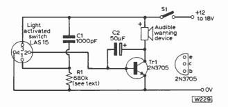
Fig. 1 : Circult diagram of the Audio Depth Alarm. The audible warning device gives a very penetrating note of about 2 ·6kHz. It is NOT a loudspeaker.
