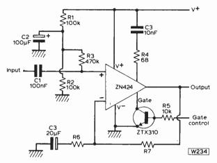
Fig. 3 : The ZN424 in an audio amplifier circuit using the gating facility.
