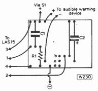
Fig. 2: The layout of the few components on a small piece of 0-1in. stripboard.
